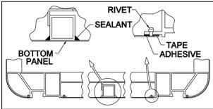
FIGURE 45 : TOP AND BOTTOM PANEL INSTALLATION
