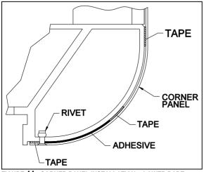
FIGURE 44 : CORNER PANEL INSTALLATION – LOWER PART
