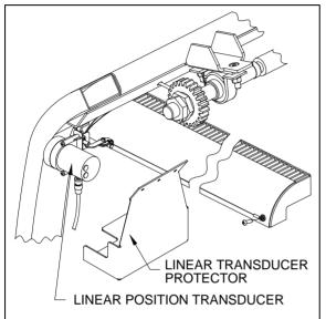
FIGURE 41 : REAR SLIDE-OUT LINEAR POSITION TRANSDUCER
