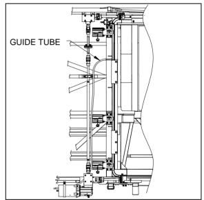
FIGURE 31 : FRONT SLIDE-OUT INFLATABLE SEAL AIR INLET
