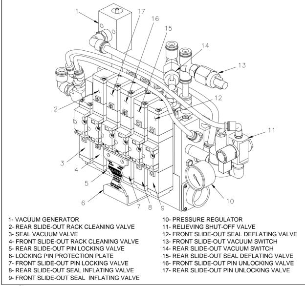
FIGURE 50 : PNEUMATIC COMPONENT PANEL
