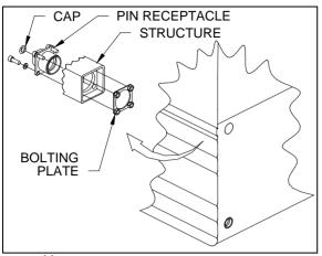
FIGURE 14 : PIN RECEPTACLE INSTALLATION
