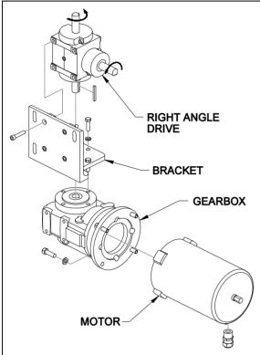
FIGURE 25 : REAR SLIDE-OUT MOTOR ASSEMBLY
