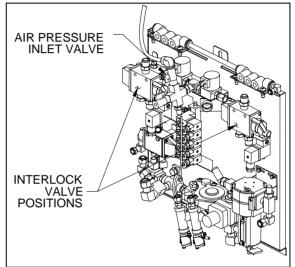
FIGURE 29 : FRONT SERVICE COMPARTMENT
