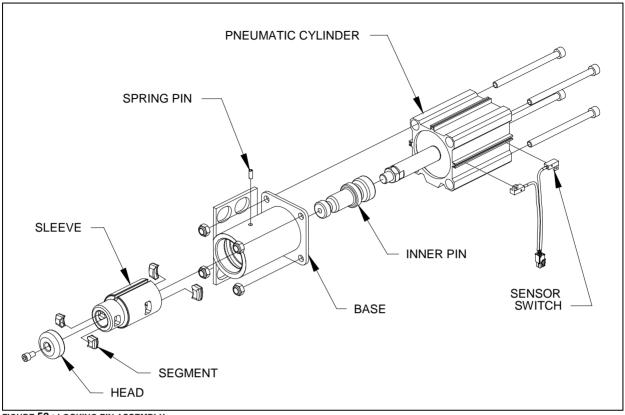
FIGURE 52 : LOCKING PIN ASSEMBLY
