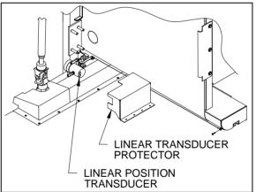
FIGURE 40 : FRONT SLIDE-OUT LINEAR POSITION TRANSDUCER
