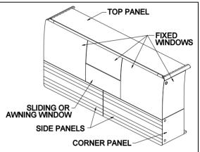
FIGURE 42 : SLIDE-OUT PANELS AND WINDOWS
