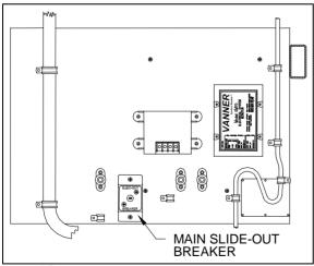
FIGURE 35 : BREAKER IN MAIN POWER COMPARTMENT
