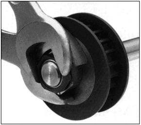
FIGURE 20 : KEYLESS BUSHING TIGHTENING
