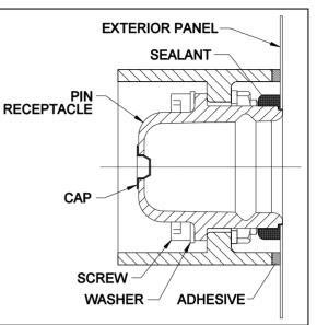
FIGURE 16 : PIN RECEPTACLE ON STAINLESS STEEL PANELS
