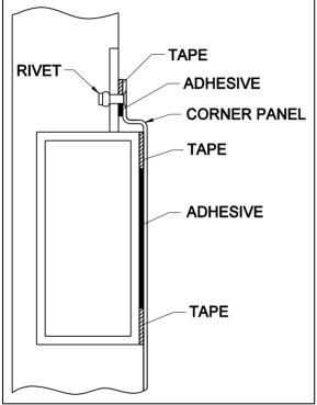
FIGURE 43 : CORNER PANEL INSTALLATION - UPPER PART
