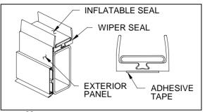
FIGURE 30 : SEAL ASSEMBLY
