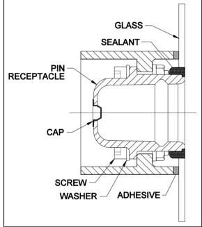
FIGURE 15 : PIN RECEPTACLE ON GLASS
