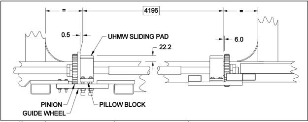
FIGURE 49 : PINION & PILLOW BLOCK ADJUSTMENT (DIMENSIONS ARE IN MILLIMETRES)
