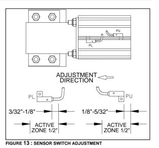
**Note:** It is important to adjust the sensor following the adjustment direction figure 13).
