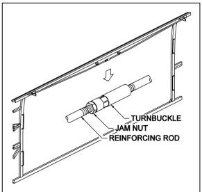
FIGURE 17 : FRONT SLIDE-OUT ROOF REINFORCING ROD
