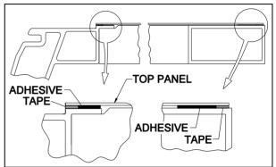
FIGURE 46 : TOP AND BOTTOM PANEL INSTALLATION
