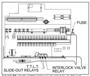
FIGURE **36** : FUSE, INTERLOCK VALVE AND T.T.L.T. RELAYS
