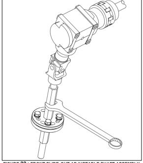
FIGURE 22 : FRONT SLIDE-OUT ADJUSTABLE SHAFT ASSEMBLY
