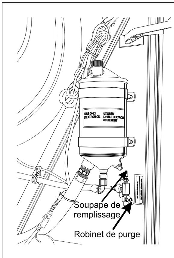
SOUPAPE DE REMPLISSAGE DU COMPARTIMENT MOTEUR 12148F
