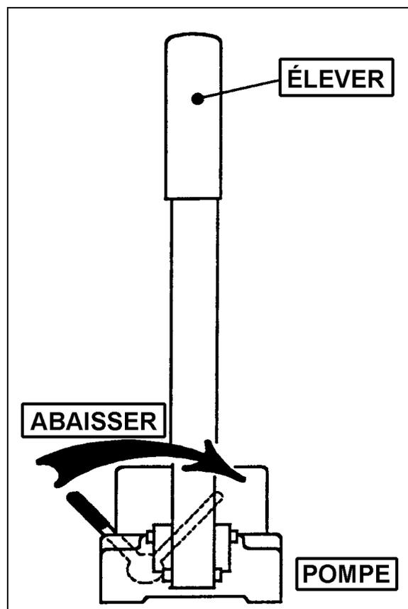
FONCTIONNEMENT MANUEL DU SYSTÈME D'ÉLEVATION 23283F
