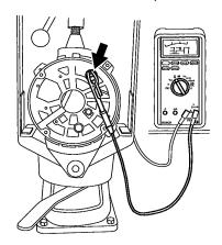
Figure 15 Testing of W Terminal Dampening Resistor
