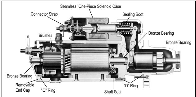
FIGURE 34: DELCO 50MT STARTER SECTIONAL VIEW
