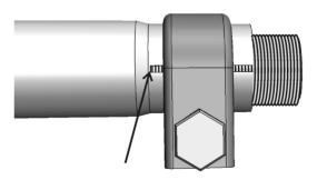
position (centered) before final clamp tightening.
