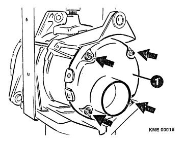
Figure 5 Air Intake Cover Removal (1)
