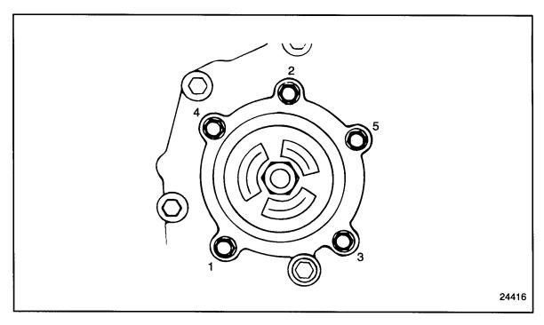
Figure 1-413 Accessory Drive Housing Bolt Torque Sequence
