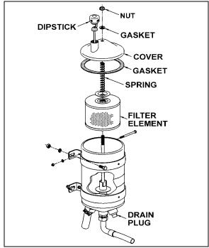
FIGURE 8: POWER STEERING FLUID RESERVOIR 14018A
