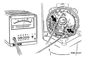
**Figure 12 Stator Resistance Testing**
