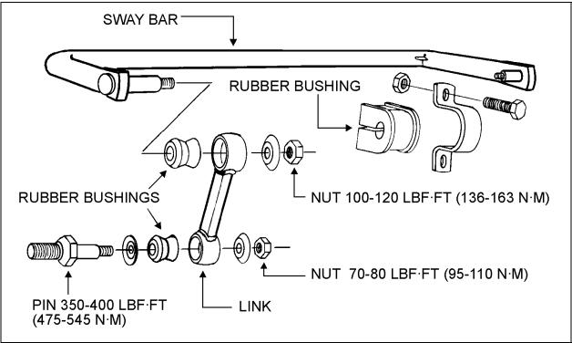
FIGURE 22: SWAY BAR (REAR SUSPENSION)
