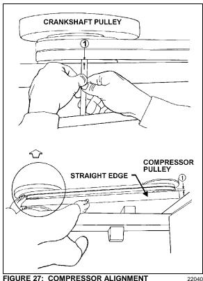
FIGURE 27: COMPRESSOR ALIGNMENT
