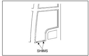
FIGURE 34: ADHESIVE-MOUNTED WINDOW
