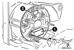
Figure 6 Voltage Regulator (1) and Suppression Capacitor (2)
