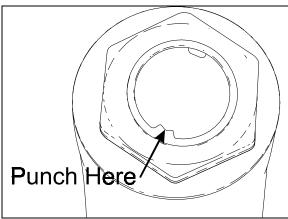
FIGURE 6: FIXING NUT PUNCH MARK
