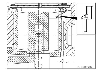
c) Wear Indicator using built in Potentiometer. This is available either as an on/off version or as a continuous signal version which can be linked to the vehicle's electronic monitoring systems.
