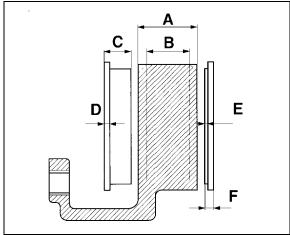
FIGURE 32: ROTOR AND PAD WEAR LIMITS
