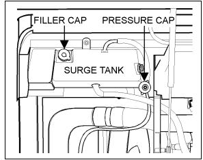
FIGURE 2: SURGE TANK - ENGINE COMPART.
