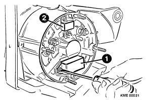
**Figure 38 Capacitor Installation** (1) Voltage Regulator (2)
