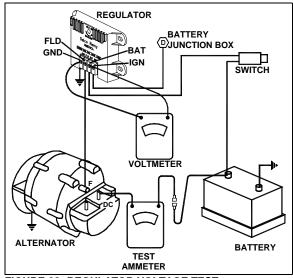
FIGURE 28: REGULATOR VOLTAGE TEST
