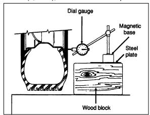
FIGURE 3: DIAL GAUGE INSTALLATION
