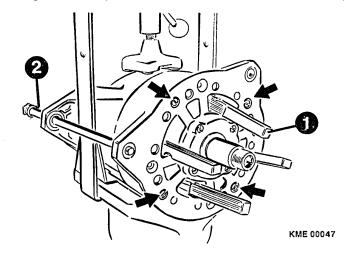
Figure 36 Drive End Shield, Stator and Collector End Shield Assembly (1) Feeler Gauge (2) Tool KDLJ 6015
