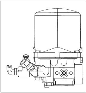
FIGURE 5: HALDEX AIR FILTER DRYER
