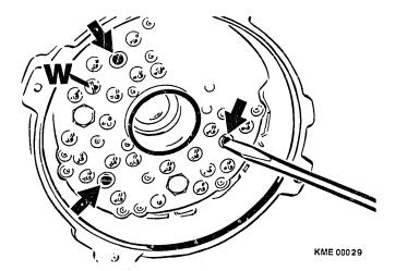
Figure 14 Rectifier Assembly Removal
