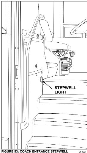
The three stepwell lights are illuminated when the door opening system is activated (Fig. 53).
