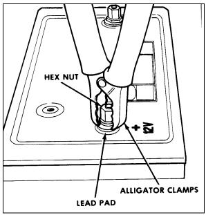
FIGURE 15: ALLIGATOR CLAMPS AND BATTERY 0606
