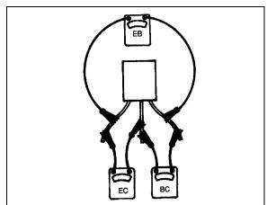
FIGURE 32: CHECKING TRANSISTORS TR2
