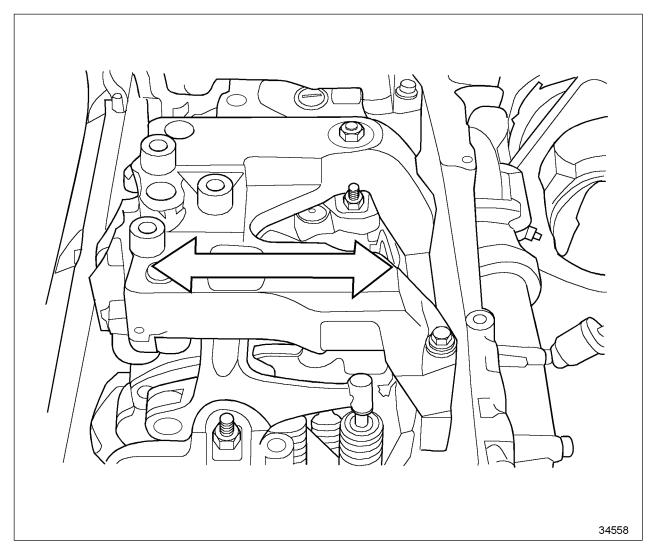
Figure 1-440 Locating Center Position of Housing
