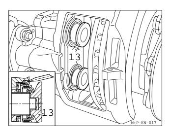
The Tappets (13) can be removed from the Threaded Tubes by using Wedge Fork A. (Order No. II32202).
