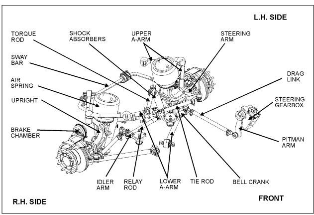
FIGURE 1: SUSPENSION AND STEERING LINKAGE
