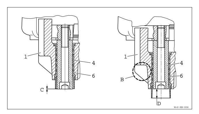
The condition of the Pads can be visually determined without removing the road wheel by noting the position of the Fixed Sleeve (4) in the Floating Caliper (1).
