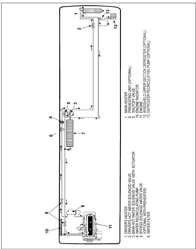
FIGURE 41: CENTRAL HEATING SYSTEM COMPONENTS
