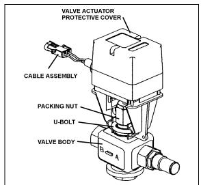
FIGURE 45: MAIN HOT WATER SOLENOID VALVE 22217
