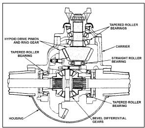
FIGURE 2: DIFFERENTIAL ASSEMBLY
