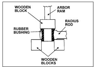
FIGURE 11: RADIUS ROD BUSHING INSTALLATION 16012
