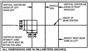
FIGURE 49: AIM INSPECTION LIMITS FOR UPPER-BEAM HEADLIGHTS 06505
