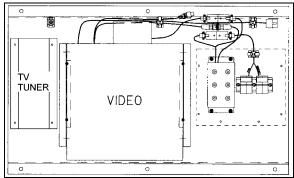
FIGURE 5: INSTALLATION IN PARCEL COMPARTMENT
