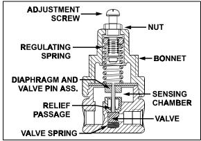
FIGURE 6: AIR PRESSURE REGULATING VALVE
