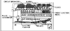
FIGURE 9: FRONT ELECT. & SERVICE COMPARTMENT<sub>06461</sub>
