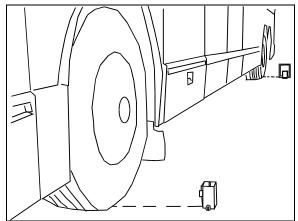
FIGURE 45: INSTALLING CALIBRATION FIXTURES 06497
