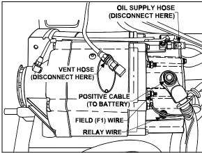
FIGURE 23: ALTERNATOR (HOSES AND WIRES)
