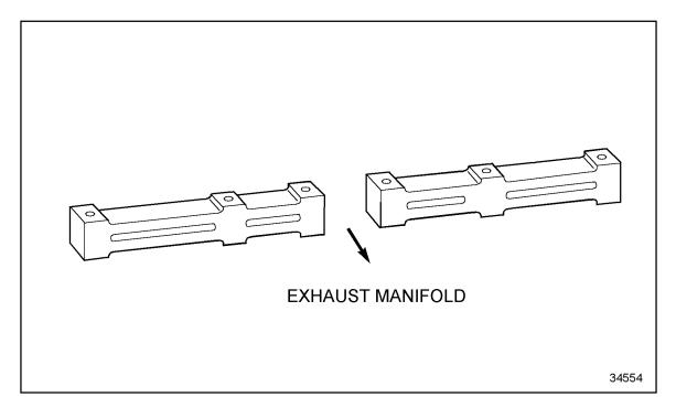
Figure 1-435 Spacer Bars with "Out" Marks Adjoined
