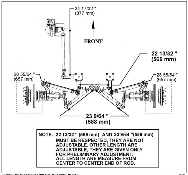
FIGURE 16: STEERING LINKAGE MEASUREMENTS
