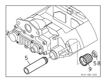
Put new Boot (9) into the Sleeve (arrow) of the Tool C (Order No II19253).
