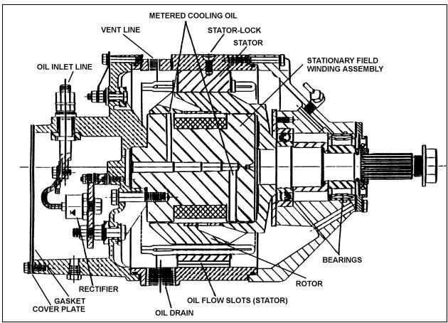
FIGURE 16: 50DN DELCO ALTERNATOR SECTIONAL VIEW
