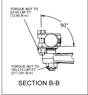
**FIGURE 3: CLAMP POSITIONING**
