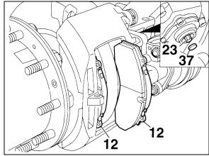
FIGURE 35: PAD INSTALLATION
