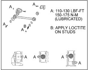
FIGURE 12: RADIUS ROD INSTALLATION
