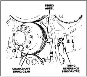
FIGURE 6: TIMING GEAR
