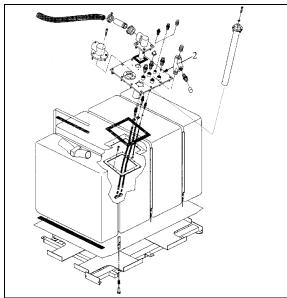
FIGURE 6: FUEL TANK ARRANGEMENT
