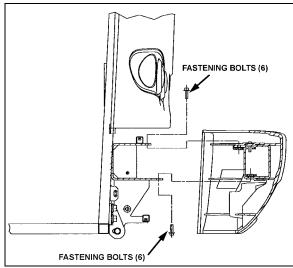
FIGURE 10: BUMPER FASTENING MECHANISM
