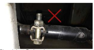
Clamp is bent. Replace clamp.
