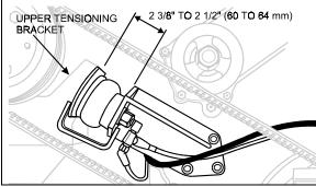
FIGURE 25: TENSIONING AIR BELLOWS
