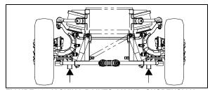
FIGURE 66: JACKING POINTS ON IND. SUSPENSION
