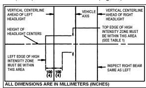
FIGURE 50: AIM INSPECTION LIMITS FOR LOWER-BEAM HEADLIGHTS 06506
