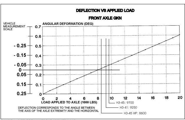
FIGURE 6: DEFLECTION VERSUS APPLIED LOAD
