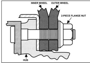
FIGURE 5: HUB-MOUNTED WHEELS
