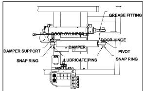
FIGURE 16: DOOR CYLINDER AND DAMPER
