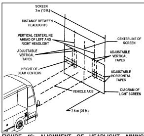
FIGURE 46: ALIGNMENT OF HEADLIGHT AIMING SCREEN 06502
