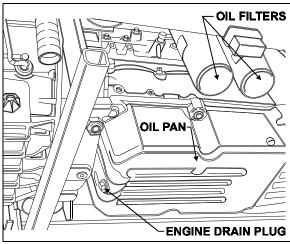
FIGURE 13: UNDER VEHICLE VIEW
