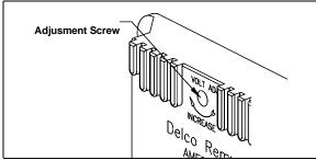
FIGURE 29: ADJUSTING REGULATOR VOLTAGE SETTING
