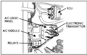
FIGURE 8: HVAC LOGIC PANEL (REAR ELECTRICAL COMPARTMENT)
