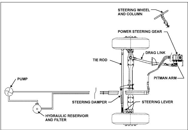
FIGURE 1: STEERING SYSTEM AXLE SETUP
