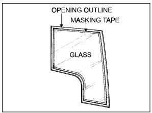
FIGURE 35: ADHESIVE-MOUNTED WINDOW
