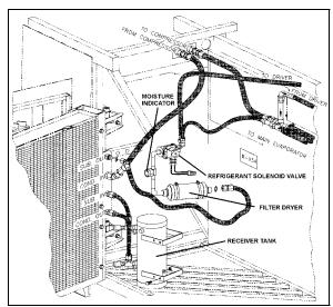
FIGURE 31: A/C CONDENSER COMPARTMENT
