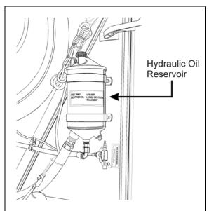
FIGURE 7: HYDRAULIC FLUID RESERVOIR LOCATION
