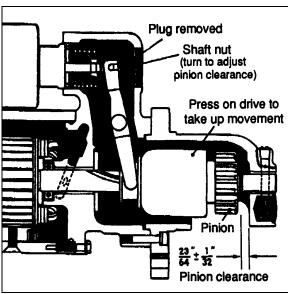
**FIGURE 35: PINION CLEARANCE**
