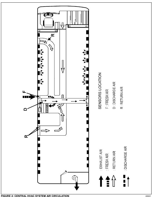
FIGURE 2: CENTRAL HVAC SYSTEM AIR CIRCULATION
