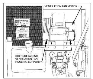
FIGURE 22: VENTILATION FAN INSTALLATION
