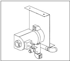
FIGURE 28: AIR HORN VALVE
