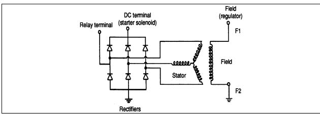
FIGURE 17: ALTERNATOR WIRING DIAGRAM (DELCO)
