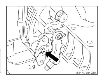
Attach Actuator with new Nuts (self-locking EN ISO 7042) and torque tighten to 180  $^{\scriptscriptstyle +30}$  Nm.
