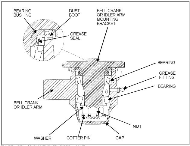
FIGURE 9: BELL CRANK AND IDLER ARM BALL JOINT
