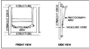
FIGURE 43: PANTOGRAPH DOOR ADJUSTMENT
