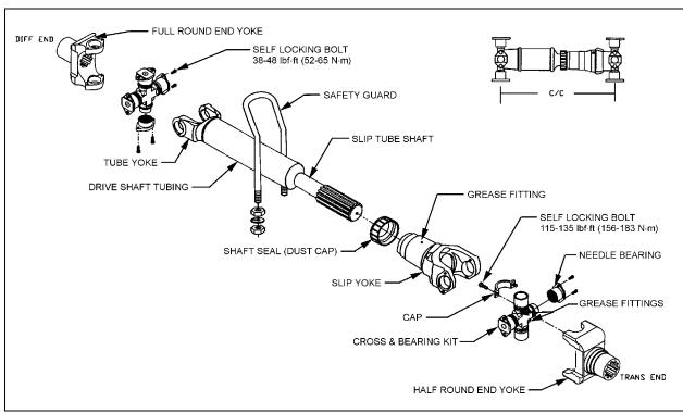
FIGURE 1: PROPELLER SHAFT ASSEMBLY
