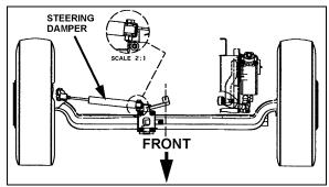
FIGURE 9: STEERING STABILIZER (DAMPER)
