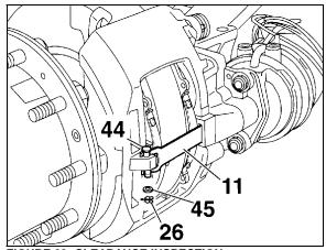
FIGURE 23: CLEARANCE INSPECTION
