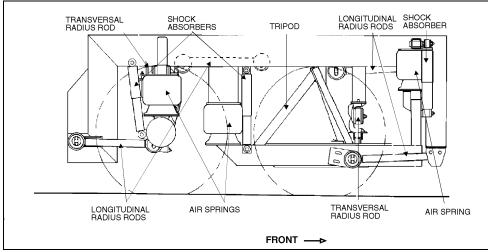
FIGURE 3: REAR SUSPENSION COMPONENTS
