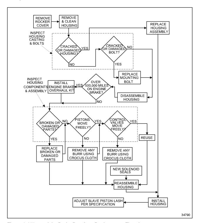
Figure 1-417 Jake Brake Repair or Replacement Flowchart
