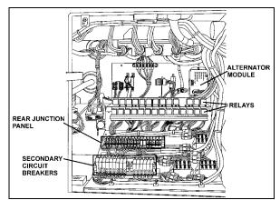
FIGURE 7: REAR ELECTRICAL COMPARTMENT
