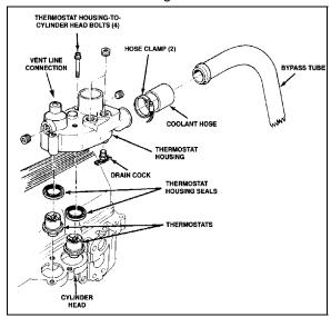
FIGURE 11: THERMOSTAT AND RELATED PARTS 0503
