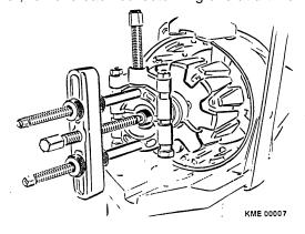
Figure 24 Collector Ring Removal
