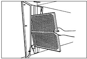
FIGURE 18: MAIN HVAC UNIT AIR FILTER
