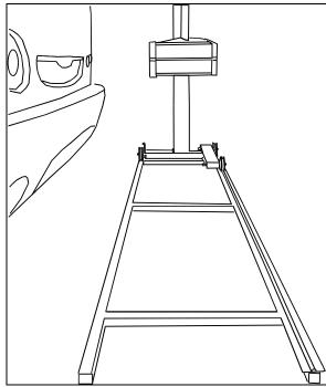
FIGURE 42: INSTALLATION OF HOOPY 100 ALIGNER 06496
