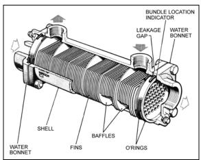
FIGURE 10: OIL COOLER SECTION VIEW
