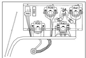
FIGURE 7: LOCATION OF RELAYS AND RESISTORS06483
