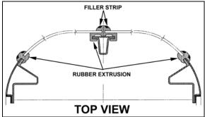
FIGURE 38: WINDSHIELD INSTALLATION TOP VIEW18098
