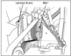
FIGURE 10: MECHANICAL LOCKING DEVICE
