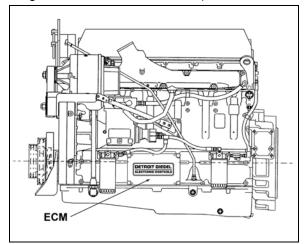
FIGURE 2: ELECTRONIC CONTROL MODULE (ECM) 01064
