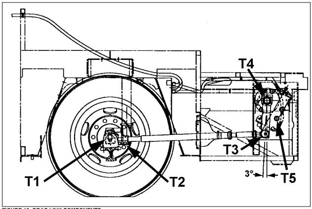
FIGURE 10: DRAG LINK COMPONENTS
