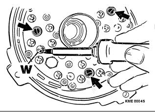
Figure 34 Rectifier Mounting and Soldering of Terminal W
