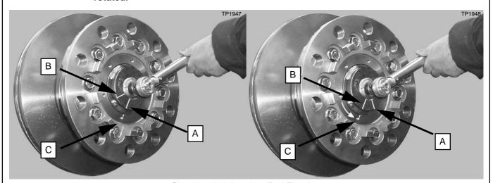
Checking hub bearing 'End Float'
