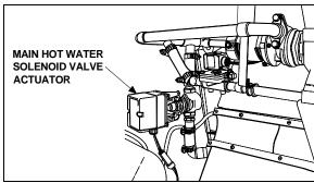
FIGURE 44: HVAC COMPARTMENT
