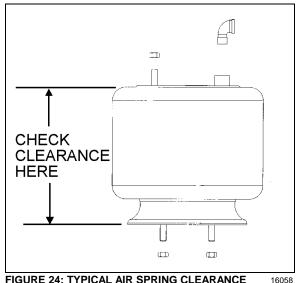
FIGURE 24: TYPICAL AIR SPRING CLEARANCE
