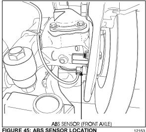
FIGURE 45: ABS SENSOR LOCATION
