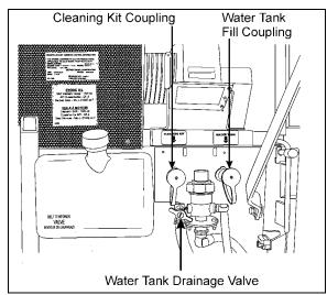
FIGURE 24: FRESH WATER TANK SERVICE VALVES
