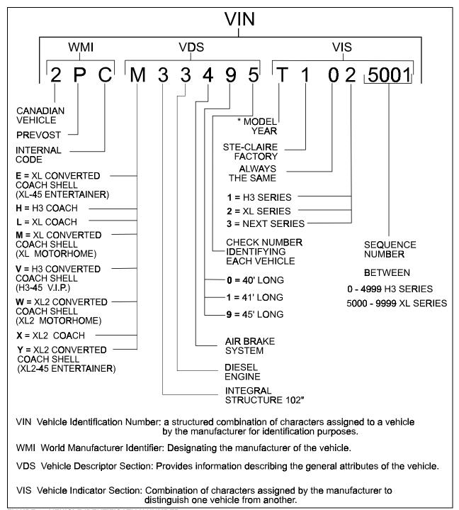
FIGURE 9 : VEHICLE IDENTIFICATION NUMBER
