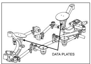
FIGURE 5: ISS TYPICAL SERIAL & MODEL NUMBERS00025C
