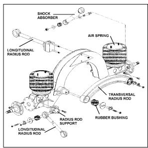
FIGURE 5: TAG AXLE SUSPENSION
