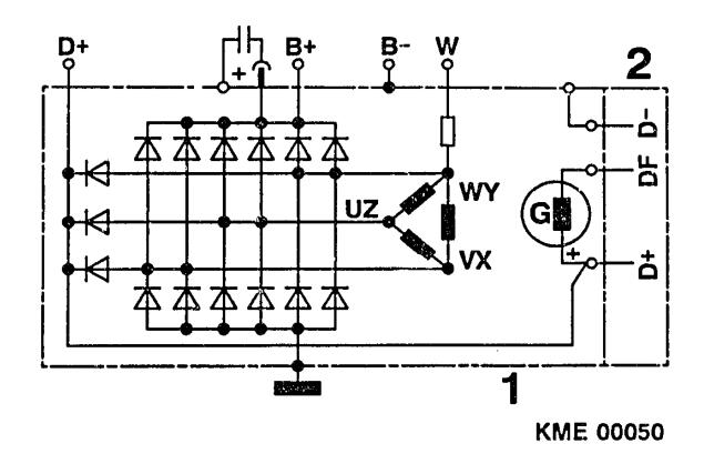
Figure 3 Alternator/Voltage Regulator Schematic
