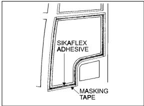
FIGURE 36: ADHESIVE-MOUNTED WINDOW
