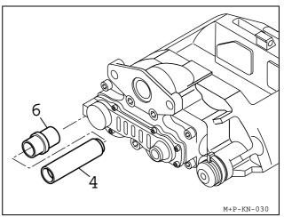
Deform new Rubber Bush (6) and push from the inner side of the Caliper into the bore. Push Rubber Bush (6) so that the outer positioning ring locates in the groove (see arrows).
