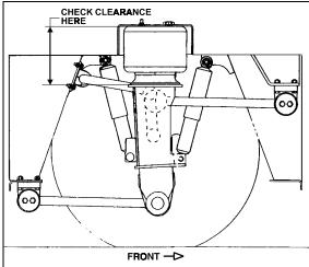
FIGURE 14: TYPICAL AIR SPRING CLEARANCE
