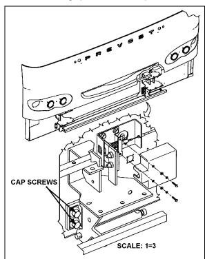
FIGURE 11: FRONT BUMPER ASSEMBLY
