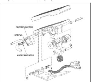
FIGURE 10: ELECTRONIC FOOT PEDAL ASSEMBLY03035
