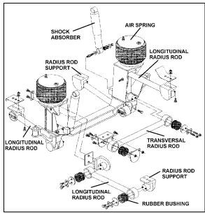
FIGURE 2: DETAILS OF FRONT SUSPENSION
