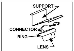
FIGURE 56: ENGINE COMPARTMENT LIGHT
