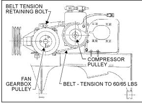
FIGURE 37: SMALL A/C COMPRESSOR INST.
