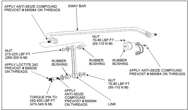
FIGURE 21: SWAY BAR (FRONT SUSPENSION)
