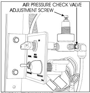
FIGURE 24: TENSIONING VALVE
