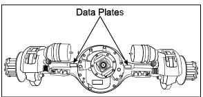
FIGURE 3: TYPICAL SERIAL AND MODEL NUMBERS 11019
