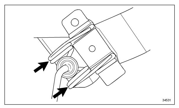
Figure 1-434 Installing the Slave Piston Assembly Torsion Spring
