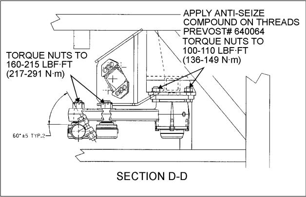
FIGURE 5: CLAMP POSITIONING
