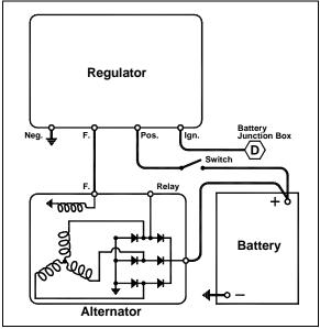
FIGURE 27: TYPICAL WIRING DIAGRAM OF A
