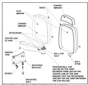
FIGURE 63: REAR-VIEW MIRROR (RAMCO)
