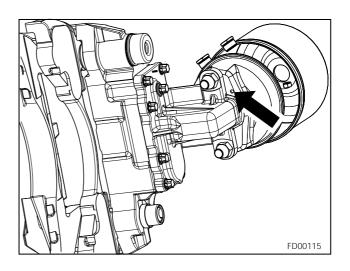
Attach Actuator with new Nuts (self-locking EN ISO 7042) and torque tighten to 180  $^{^{\tiny{+30}}}$  Nm.
