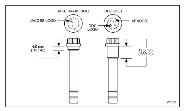
Figure 1-437 Jake Brake and DDC Bolt Identification
