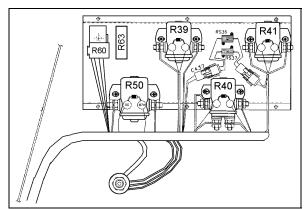
FIGURE 11: CONTROL PANEL IN HVAC COMPARTMENT<sub>06483</sub> Each relay or resistor is identified to facilitate its location (Fig. 11).
