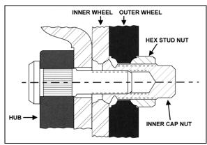
FIGURE 4: STUD-MOUNTED WHEELS
