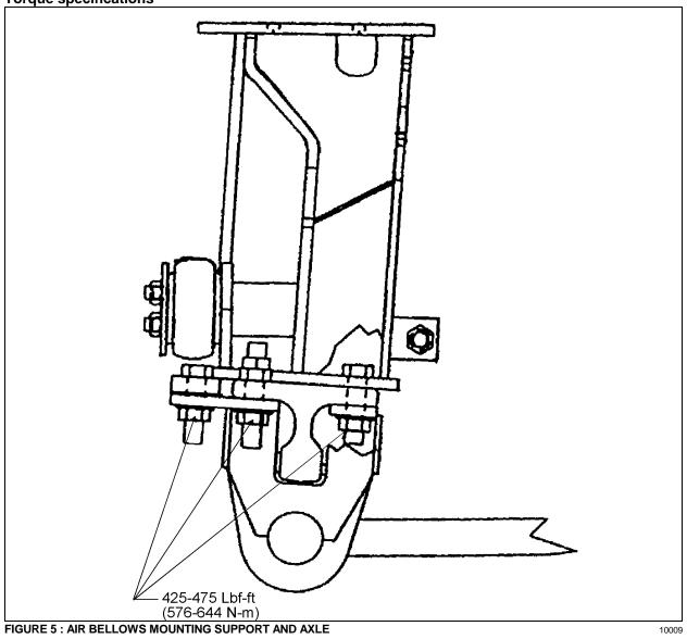
For more torque specifications, see "GKN Parts and Service Manual for Axles" annexed at the end of this section, under heading "Tightening Torque Table for type S-82 Steer Axle.
