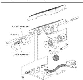
FIGURE 14: ELECTRONIC FOOT PEDAL ASSEMBLY 03035
