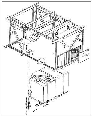
FIGURE 7: FUEL TANK INSTALLATION
