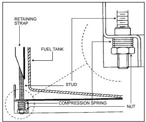
FIGURE 8: FUEL TANK RETENTION
