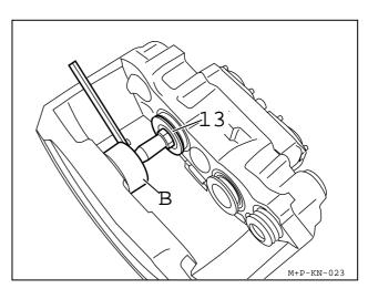
8 Caliper Suspension sealing (Replacement of inner Boot (9)) (for the Axial and Radial Disc Brake)
