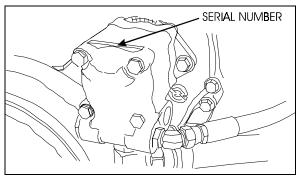
FIGURE 6 : POWER STEERING PUMP SERIAL NUMBER
