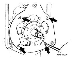
Figure 10 Drive End Shield Removal
