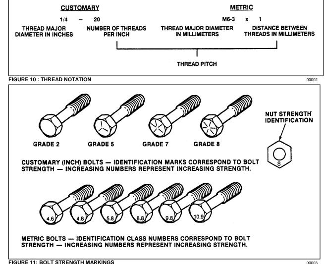
FIGURE 11: BOLT STRENGTH MARKINGS
