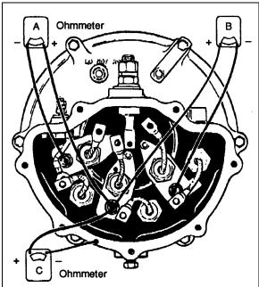
FIGURE 22: CHECKING STATOR WINDING FOR "OPEN"
