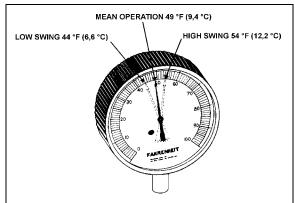
FIGURE 35: HIGH & LOW SWING TEMPERATURE AT REMOTE BULB 22047
