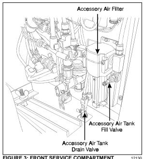
FIGURE 3: FRONT SERVICE COMPARTMENT
