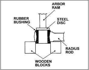
FIGURE 10: RADIUS ROD BUSHING REMOVAL
