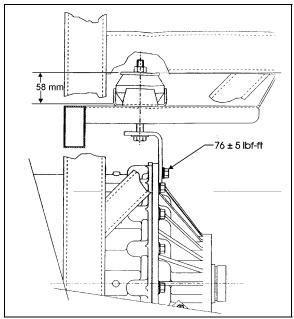
FIGURE 12: NUT TOLERANCE
