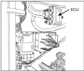
FIGURE 14: WTEC/ELECTRONIC CONTROL UNIT 07039
