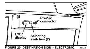
**Note:** The destination sign must be programmed with a computer connected to the RS-232 connector prior to first use. Follow the instructions on the computer disk to install and run the software.
