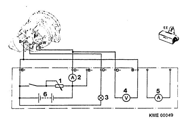
Figure 39 Alternator Test Bench Hook-up Schematic
