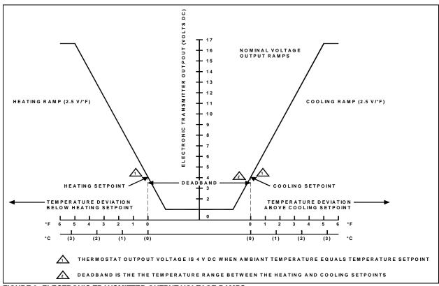
FIGURE 9: ELECTRONIC TRANSMITTER OUTPUT VOLTAGE RAMPS
