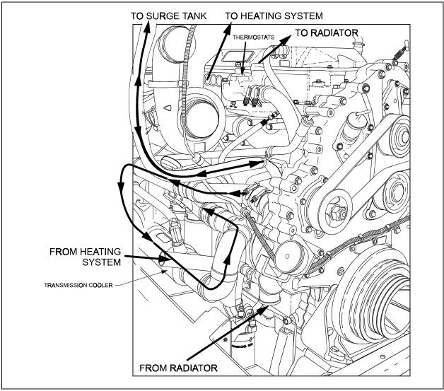
FIGURE 1: COOLING SYSTEM
