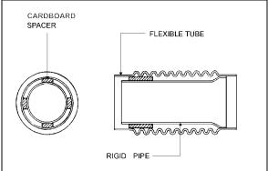
FIGURE 2: FLEXIBLE TUBE INSTALLATION
