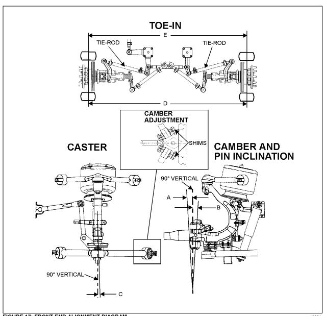
FIGURE 17: FRONT END ALIGNMENT DIAGRAM
