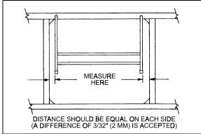
FIGURE 44: PANTOGRAPH DOOR ADJUSTMENT
