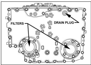
FIGURE 5: PLUG AND FILTERS
