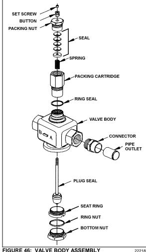
FIGURE 46: VALVE BODY ASSEMBLY
