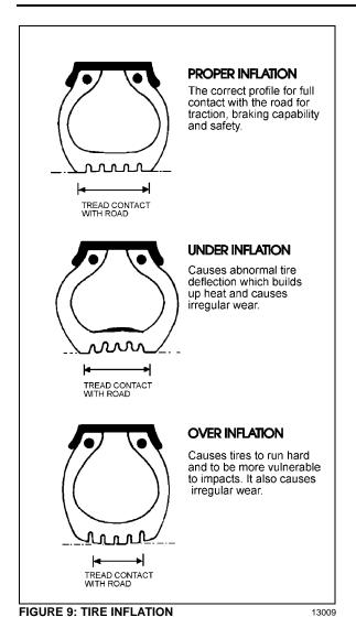
**Caution:** Never bleed air from hot tires as tires will then be under inflated. Use an accurate tire gauge to check pressures (Do not kick tires as an inflation check. This is an unreliable method).
