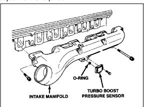
FIGURE 7: TURBO BOOST PRESSURE SENSOR
