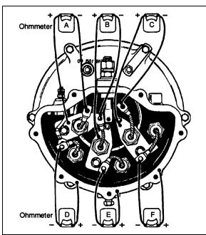
FIGURE 21: CHECKING DIODES WITH OHMMETER ON
