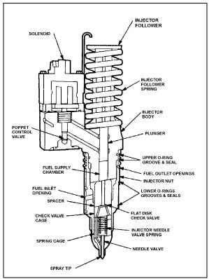
FIGURE 3: UNIT INJECTOR CROSS SECTION
