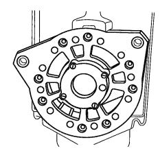
Figure 27 Drive End Bearing Retaining Screws
