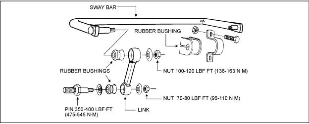
FIGURE 13: FRONT & DRIVE AXLE SWAY BAR
