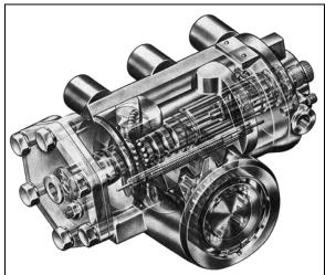
FIGURE 2: POWER STEERING GEAR
