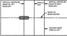
FIGURE 47: HIGH-INTENSITY ZONE (SHADED AREA) OF A PROPERLY AIMED UPPER BEAM ON THE AIMING SCREEN 7.6 M (25FT) IN FRONT OF VEHICLE 06503
