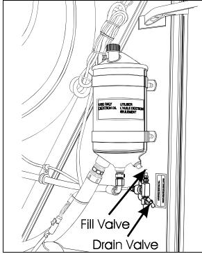
**FIGURE 27: REAR VALVE LOCATION**
