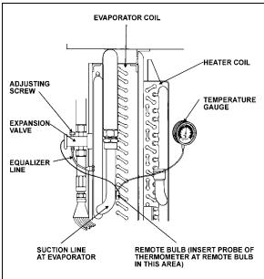
FIGURE 34: SUPERHEAT ADJUST. INSTALLATION 22046
