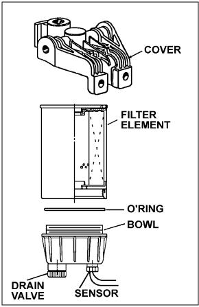
FIGURE 3: FUEL FILTER/WATER SEPARATOR
