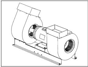
FIGURE 21: EVAPORATOR MOTOR ASSEMBLY
