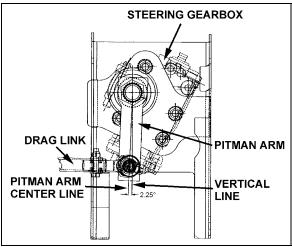
FIGURE 7: PITMAN ARM ALIGNMENT
