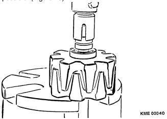
**Figure 25 Pressing on Collector Rings**
