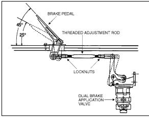
FIGURE 12: BRAKE PEDAL ADJUSTMENT
