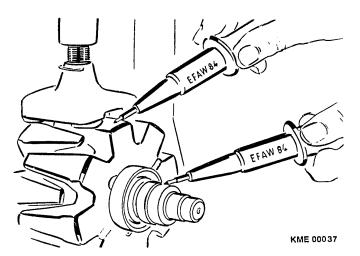
Figure 22 Rotor Insulation Testing
