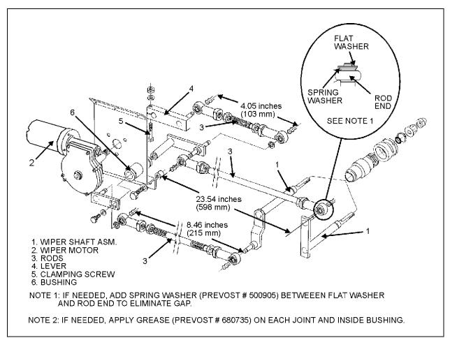
FIGURE 36: UPPER WINDSHIELD WIPER INSTALLATION
