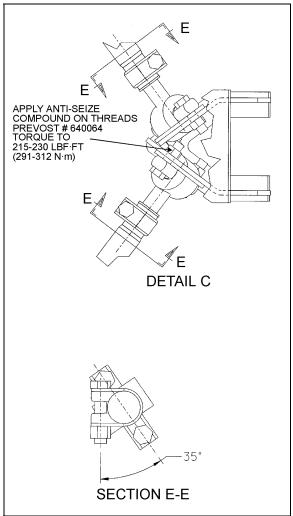
FIGURE 6: CLAMP POSITIONING
