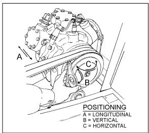
FIGURE 28: COMPRESSOR ALIGNMENT
