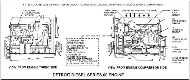
FIGURE 1: DETROIT DIESEL SERIES 60 ENGINE (TYPICAL)
