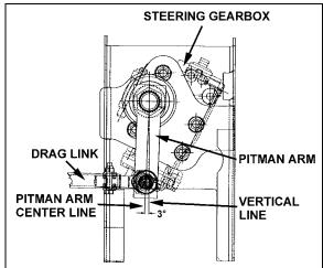
FIGURE 5: PITMAN ARM ADJUSTMENT
