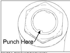
FIGURE 8: FIXING NUT PUNCH MARK
