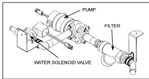
FIGURE 47: VIP WATER RECIRCULATION PUMP INSTALLATION
