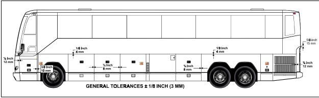
FIGURE 40: BODY PANEL SPACING
