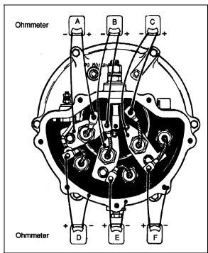
FIGURE 20: CHECKING DIODES WITH OHMMETER ON
