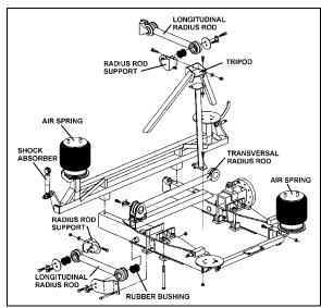
FIGURE 4: DETAILS OF REAR SUSPENSION
