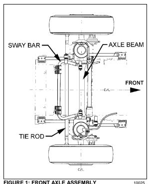
FIGURE 1: FRONT AXLE ASSEMBLY
