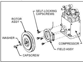
FIGURE 36: PULLEY INSTALLATION
