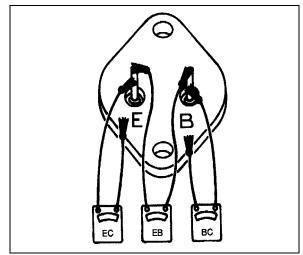
FIGURE 31: CHECKING TRANSISTORS TR1
