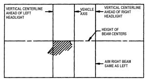
FIGURE 48: HIGH-INTENSITY ZONE (SHADED AREA) OF A PROPERLY AIMED LOWER BEAM ON THE AIMING SCREEN 7.6 M (25 FT) ON FRONT OF VEHICLE 06504
