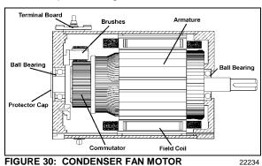
FIGURE 30: CONDENSER FAN MOTOR
