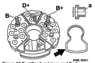
Figure 32 Rectifier Insulators and Seal
