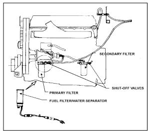
FIGURE 2: MANUAL SHUT-OFF VALVES
