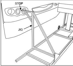
FIGURE 41: INSTALLATION OF JIGS
