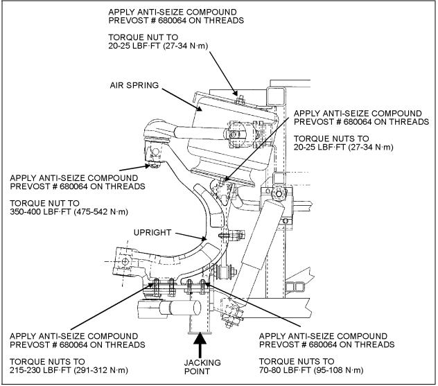
FIGURE 19: AIR SPRING AND SHOCK ABSORBER
