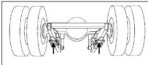
FIGURE 5: JACKING POINTS ON DRIVE AXLE
