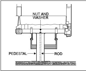
FIGURE 27: SEAT PEDESTAL ASSEMBLY
