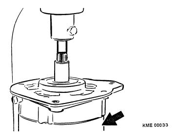
Figure 18 Pressing out Rotor
