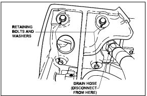
FIGURE 24: ALTERNATOR RETAINING BOLTS AND WASHERS 06350
