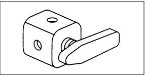
FIGURE 21: THREE WAY VALVE
