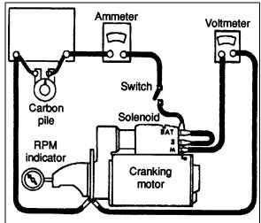
FIGURE 33: STARTING MOTOR TEST CONNECTIONS
