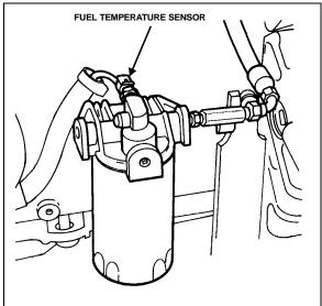
FIGURE 8: FUEL TEMPERATURE SENSOR
