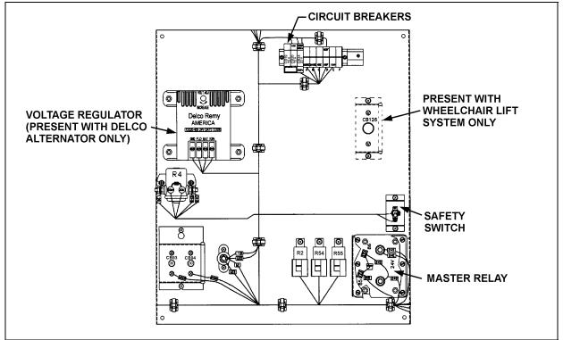
FIGURE 5: MAIN POWER COMPARTMENT
