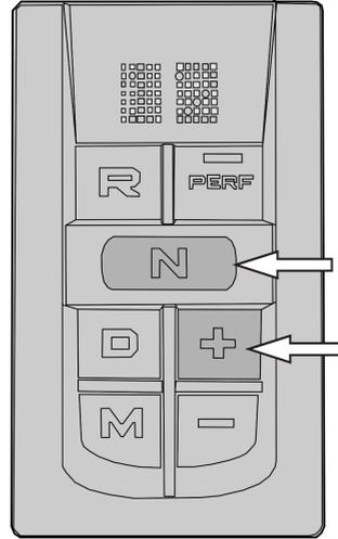
To activate the Limp Home mode for basic version of gear selector pad:
