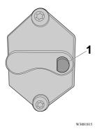
Circuit breaker button on thermal protector device.
