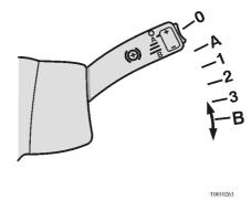
Use the "SET" button **A** in the retarder control lever to control the speed limiter.
