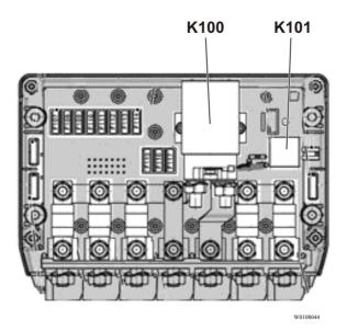
Relays in the electrical distribution box corresponding to the I-Start system
