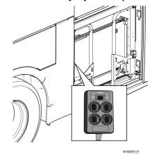
Locate of control pendant into the Wheel Chair Lift (WCL) bus compartment.
