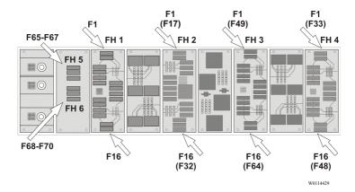
The fuses numbering its according to the circuit board position and into the parenthesis the equivalent printed on the electrical distribute unit labels.
