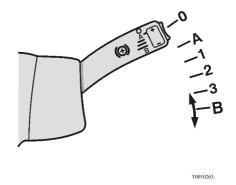
**Note:** The **B** position for the retarder control lever only appears in buses equipped with **I-Shift** transmission.
