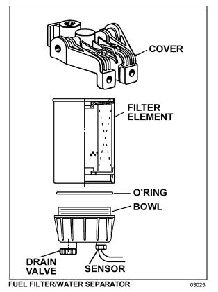
The optional Fuel Pro 382 diesel fuel filter system consists of a permanently mounted fuel
