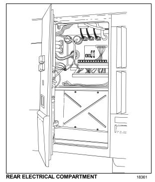
The rear electric compartment door can be locked/unlocked using the exterior compartment key. Turn the key in the compartment door lock to remove.
