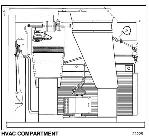
The HVAC compartment also contains relays and resistors. They are mounted on the control panel located on the R.H. side wall when facing the compartment.
