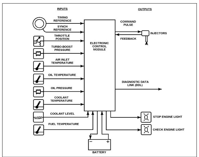
SHEMATIC DIAGRAM OF DDEC IV SYSTEM
