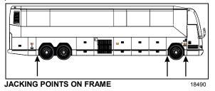
**Warning:** The suspension of the vehicle must be in the normal ride position before jacking. The level low system must be in the OFF position prior to turning OFF the ignition key.
