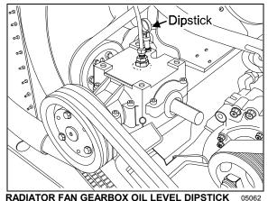
Check radiator fan gear box oil level as follows:
