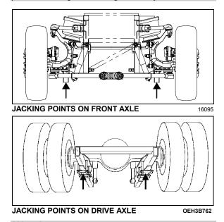
**Warning:** Always unload or retract the tag axle before jacking the vehicle from the front and drive axle jacking points to prevent damage to suspension components.
