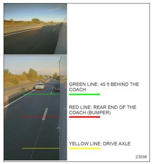
FIGURE 53: REFERENCE LINES IN MONITOR
