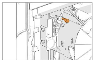
FIGURE 16: ENGINE COMPARTMENT AIR-FILL VALVE
