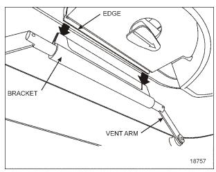
FIGURE 4: ROOF ESCAPE LATCHING
