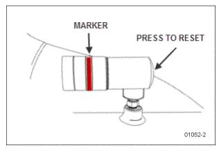
FIGURE 19: AIR FILTER RESTRICTION INDICATOR
