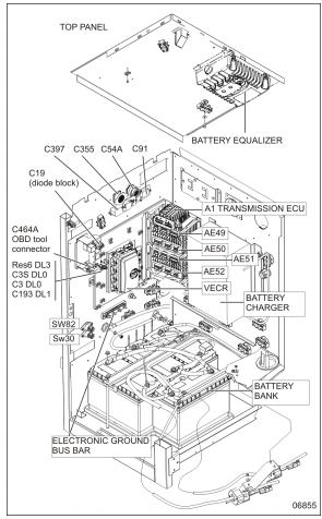
FIGURE 10: VIEW OF MAIN POWER COMPARTMENT (TYPICAL)
