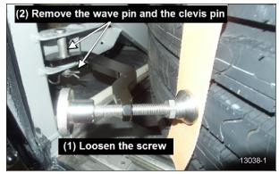
FIGURE 12: REMOVING THE SPARE WHEEL
