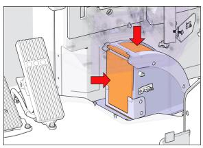
FIGURE 22: TWO RECIRCULATING AIR FILTERS LOCATED UNDER THE CENTRAL UTILITY COMPARTMEN
