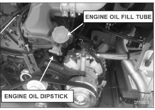
FIGURE 4: ENGINE OIL DIPSTICK - VOLVO D13 ENGINE
