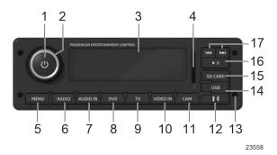
The VSS-06 Video and Sound Selector enables the driver to select audio, audio/video and video sources with settings of volume level, bass, treble, loudness for the passenger's area only. The DVD player, media player, microphones and auxiliary audio or video sources are controlled with this unit.
