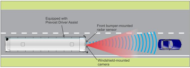
FIGURE 41: PREVOST DRIVER ASSIST™ SYSTEM USES A CAMERA AND RADAR SENSOR
