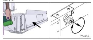
4. Lift the left handrail upward out of its socket. Lower handrail to platform. Repeat for right handrail.
