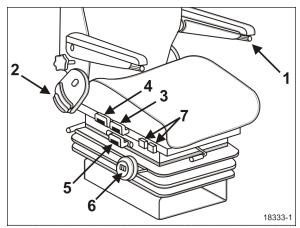
FIGURE 3: DRIVER'S SEAT ADJUSTMENT (MECHANICAL)
