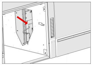
FIGURE 23: PASSENGERS AREA AIR FILTER
