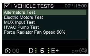
This feature will activate one alternator at a time during 5 seconds, cycling between alternator 1, 2 & 3.
