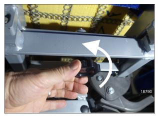
FIGURE 9: LOOSEN THE KNOB
