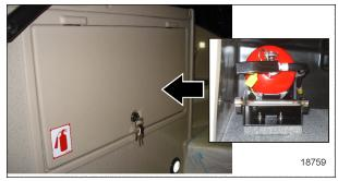
FIGURE 8: A DECAL INDICATES THAT A FIRE EXTINGUISHER (OPTION) IS LOCATED IN THE DRIVER'S PERSONAL COMPARTMENT
