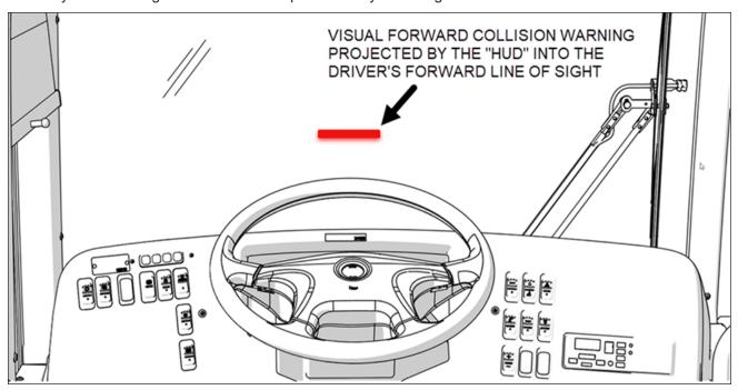
FIGURE 43: HEAD-UP DISPLAY PROJECTED VISUAL WARNING
