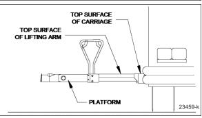
FIGURE 14: LIFTING ARM AND CARRIAGE AT SAME HEIGHT
