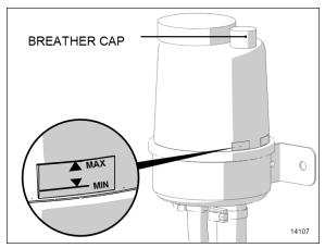
FIGURE 10: POWER STEERING FLUID TANK
