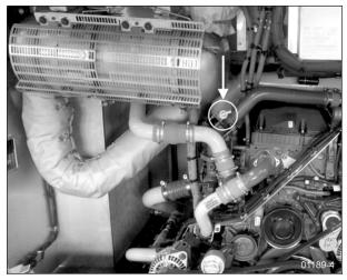
FIGURE 6: TRANSMISSION FLUID DIPSTICK (H3 SERIES)
