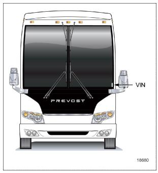
FIGURE 12: VEHICLE IDENTIFICATION NUMBER (H3 SERIES)
