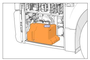
FIGURE 13: WINDSHIELD WASHER FLUID RESERVOIR
