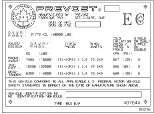
FIGURE 10: EXAMPLE OF CERTIFICATION PLATE
