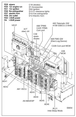
FIGURE 23: FRONT ELECTRICAL COMPARTMENT
