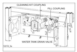
FIGURE 3: LAVATORY COUPLING & DRAIN VALVE
