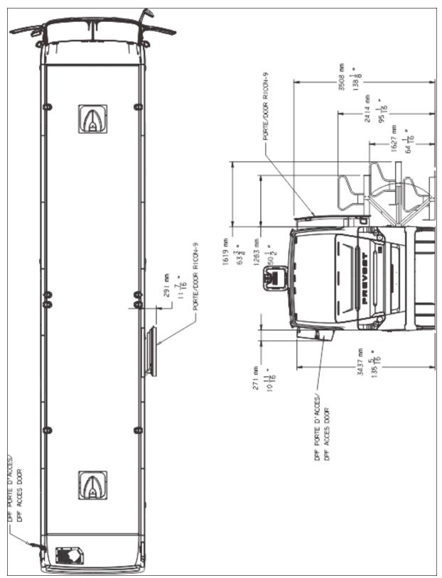
FIGURE 3: H3 SERIES WITH WHEELCHAIR LIFT - OVERALL DIMENSIONS
