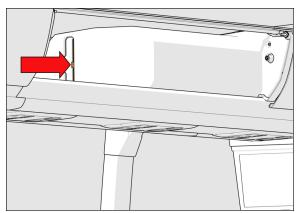
FIGURE 24: OVERHEAD COMPARTMENT FAN AIR FILTER
