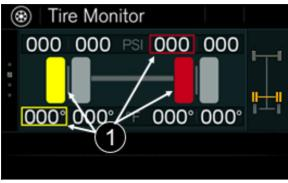
FIGURE 36: READING PRESSURE AND TEMPERATUREON ON DRIVE AXLE TIRES WITH IRREGULARITIES DETECTED (DISPLAY EXAMPLE)
