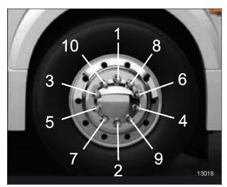
FIGURE 13: TIGHTENING SEQUENCE
