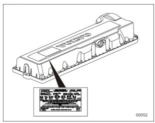
FIGURE 5: VOLVO D13 ENGINE DATA PLATE
