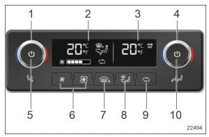
FIGURE 17: CONTROL UNIT FOR HIGH CAPACITY CENTRAL HVAC SYSTEM
