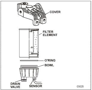
FIGURE 15: FUEL FILTER/WATER SEPARATOR
