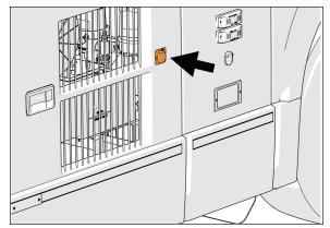
FIGURE 9: BATTERY CHARGER 120-VOLT CONNECTOR
