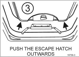
FIGURE 3: EMERGENCY ROOF ESCAPE OPENING
