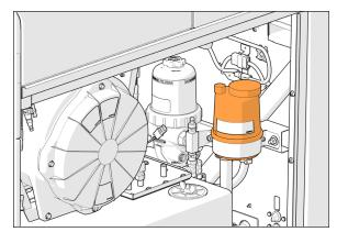
FIGURE 9: POWER STEERING RESERVOIR
