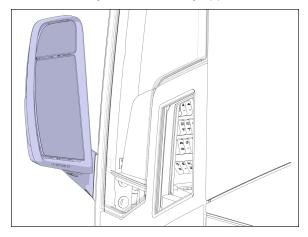
To provide good visibility in cold weather, the mirrors can be equipped with heating elements. The elements are activated by a rocker switch located on the dashboard. Refer to "Controls & Instruments" chapter. Thermostats are used to prevent continuous operation of the heating elements.
