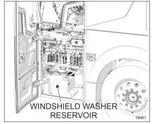
FIGURE 24: FRONT ELECTRICAL & SERVICE COMPARTMENT
