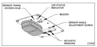
**FIGURE 25: TWS MODULE DETAIL**
