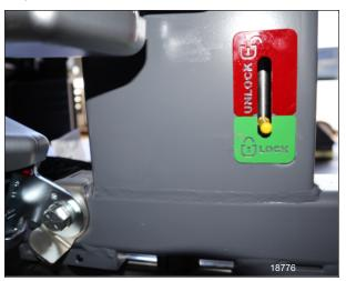
FIGURE 19: SECONDARY LOCK INDICATOR
