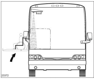
FIGURE 26: CHECKING NORMAL PLATFORM POSITION
