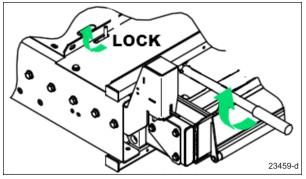
6. Lift right handrail to vertical and push firmly down into its socket. Repeat for left handrail.
