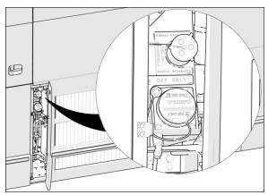
FIGURE 12: FUEL AND DIESEL EXHAUST FLUID (DEF) FILLER NECKS
