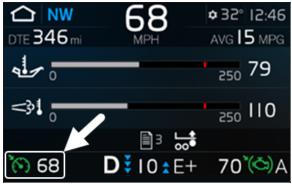
FIGURE 40: CRUISE CONTROL SET SPEED
