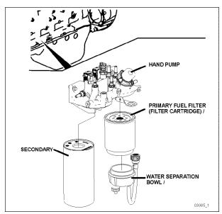
FIGURE 16: FUEL FILTERS WITH VOLVO D13 ENGINE
