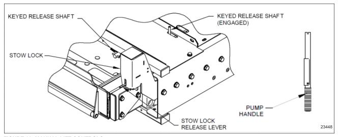
FIGURE 12: MANUAL LIFT CONTROLS
