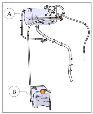
FIGURE 11: COOLANT TANKS ARRANGEMENT
