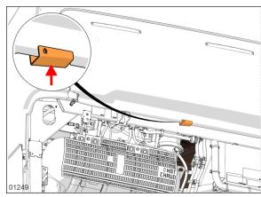
FIGURE 5: EXHAUST AFTERTREATEMENT SYSTEM ACCESS HATCH
