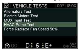
In test mode, with the parking brake applied and the passenger set point set to a value higher than 64°F (18°C), the circulator pump is not set to OFF as it would normally do when the outside temperature gets above 50°F (10°C). This feature allows verification of the pump when inside a garage. This is also useful when working on the heating system to remove air pockets trapped in the system.
