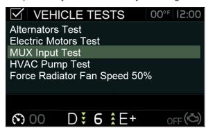
In VEHICLE TESTS, select MUX INPUT TEST. Press ENTER / SELECT button to start the test.
