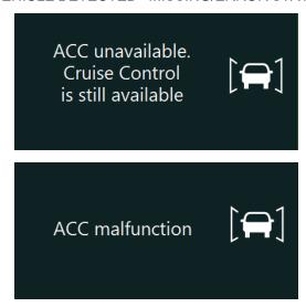
For the proper functioning of the system, the radar must be perfectly aligned and not blocked. If a radar fault condition is detected, one of the following pop-up messages will show in the DID.
