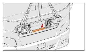
FIGURE 20: DRIVER HVAC SYSTEM FRESH AIR FILTER
