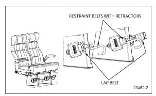
FIGURE 23: WHEELCHAIR AND OCCUPANT RESTRAINT SYSTEM
