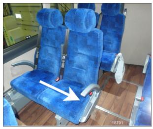
FIGURE 10: PULL TO UNLOCK THE ROTATION
