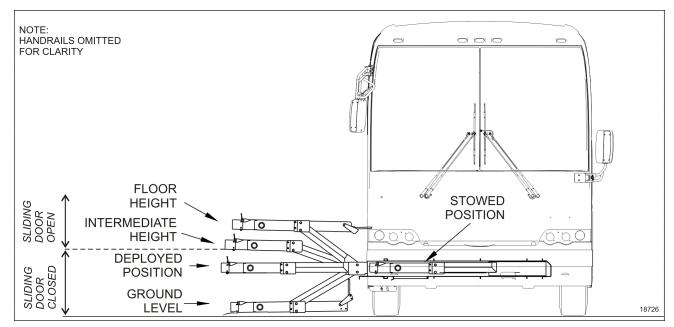
FIGURE 9: PLATFORM POSITION WITH INTERMEDIATE HEIGHT (OPTIONAL FEATURE)
