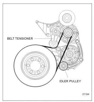
FIGURE 11: LIMP-HOME BELT ON TOP ALTERNATOR
