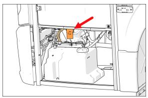
FIGURE 20: WIPERS MECHANISM ACCESS HATCH RELEASE LEVER
