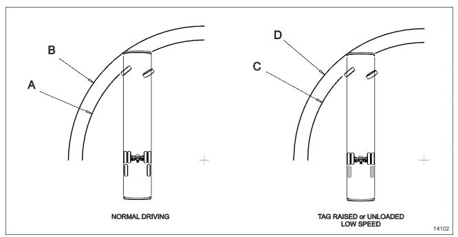
FIGURE 4: TURNING RADIUS DIAGRAM
