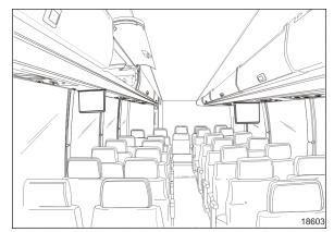
FIGURE 18: OVERHEAD STORAGE COMPARTMENTS
