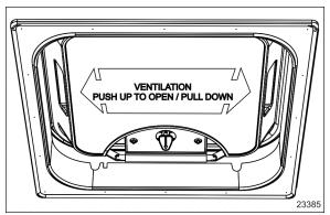
**FIGURE 17: VENTILATION HATCH**
