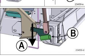
4. Pull rollstop control knob out and rotate fully counterclockwise. Rollstop must lie flat on ground.
