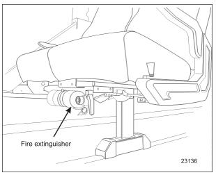
FIGURE 7: FIRE EXTINGUISHER UNDER FIRST ROW SEAT
