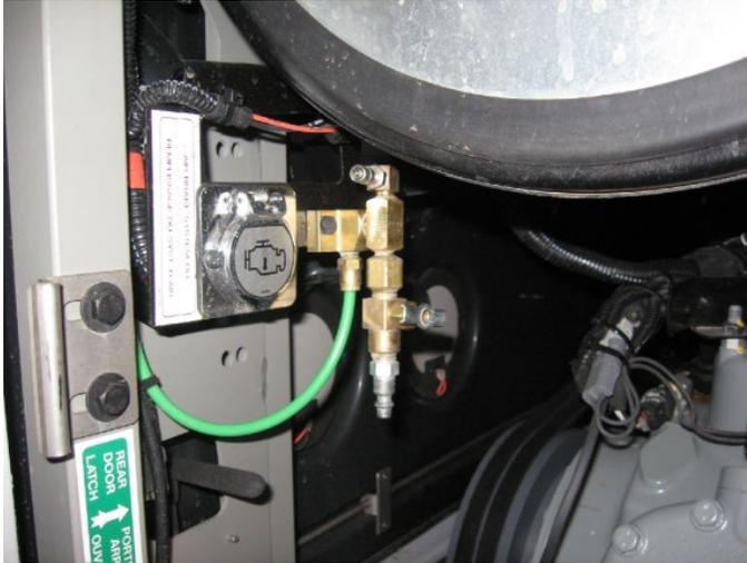
Figure 23: ENGINE COMPARTMENT EMERGENCY AIR-FILL VALVE
