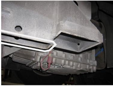
Figure 2: CHASSIS HOISTING POINTS - AFT OF TAG AXLE
