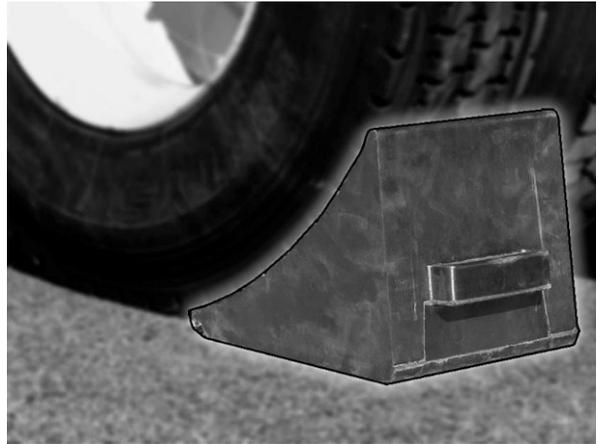
Figure 19: CHOCK THE FRONT AND REAR WHEELS
