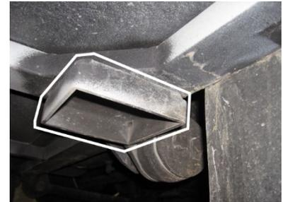
Figure 4: CHASSIS HOISTING RECEPTACLES - AFT OF FRONT AXLE
