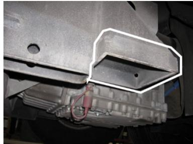
Figure 3: CHASSIS HOISTING RECEPTACLES - AFT OF TAG AXLE
