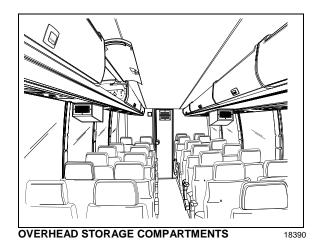
**Note:** The overhead storage compartments have a minimum amount of separators installed so as to quicken inspection for forgotten objects.
