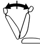
Lift lever (2) then adjust backrest to desired angle.
