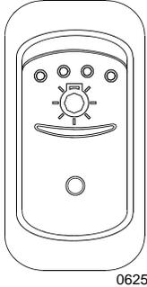
Press rocker switch to the first position to activate clearance, tail and marker lights. Push down fully to turn ON both the clearance and marker lights and the headlights. The controls and instrument lights will illuminate.
