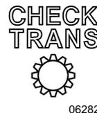
Illuminates when the ignition is switched ON. The indicator light should go out once the engine starts.
