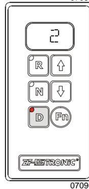
**Warning:** If the driver does not respond to the “CL”, a change is made from maneuvering mode into setting off mode. The vehicle may accelerate rapidly.
