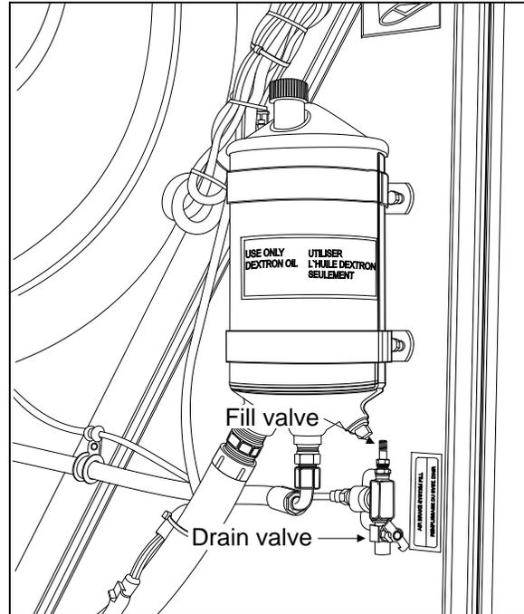
**FILL VALVE IN ENGINE COMPARTMENT** 12162
