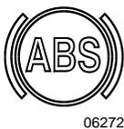
Illuminates when the ABS is not available or when the ABS is malfunctioning. Since the ABS system does not operate under 4 mph (7 km/h), the indicator will remain illuminated until the coach reaches that speed. Refer to "Other Features" chapter.
