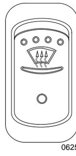
Optionally, the coach may be equipped with a de-icing system in the windshield upper section. Press the rocker switch to activate the recirculating pump and the blower in order to clear fog, frost or thin ice from either side of the windshield upper sections.
