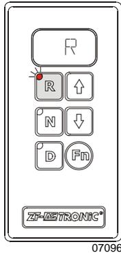
⇒ The vehicle **must** be at a standstill.
