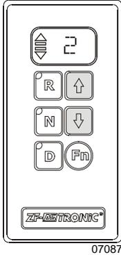
The system selects 2<sup>nd</sup> starting gear as default. The driver may select 1<sup>st</sup> starting gear.
