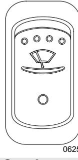
Press the rocker switch to the first position to activate the upper wipers intermittently.
