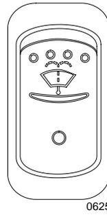
Press the rocker switch to spray the upper windshields with washer fluid. Windshield wipers will automatically come on and stop a few seconds after releasing the switch.
