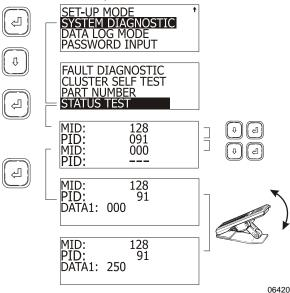
In this example, a throttle pedal in good working order will send a linear and continuous (no jumps) signal to the ECU, appearing as DATA value on the MCD screen. Full pedal movement will display values from 000 (no throttle) to 250 (maximum throttle).
