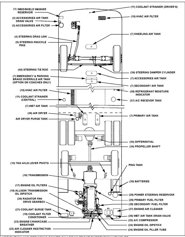
**LUBRICATION AND SERVICING POINTS ON I-BEAM FRONT SUSPENSION VEHICLES**
