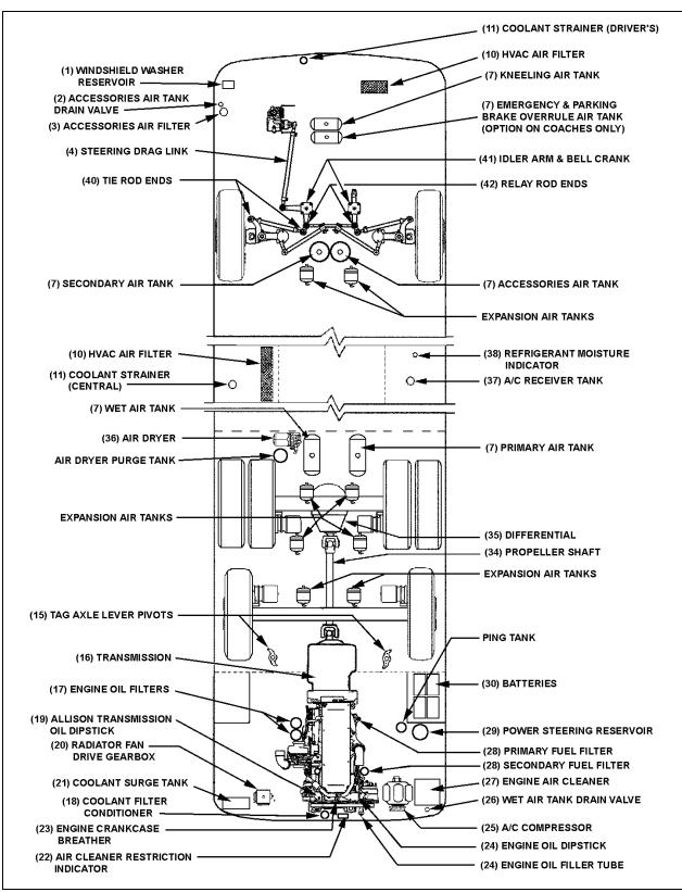
LUBRICATION AND SERVICING POINTS ON INDEPENDENT FRONT SUSPENSION VEHICLES
