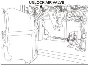
FRONT SERVICE COMPARTMENT UNLOCK AIR VALVE
