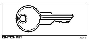
Ignition key also serves as a master switch. Use the ignition key to activate the electrical circuit by turning it counterclockwise to the *ACC* position or to start the engine by turning the key clockwise to the start position, then releasing.
