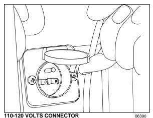
Caution: Connect only to a 110-120 VAC power source. Use only grounded (three prongs) extension cords with a minimum rated capacity of 15 amps. Disconnect the extension cord before starting. Before driving, make sure the extension cord is disconnected and the engine compartment door is closed.
