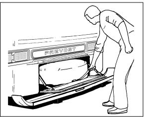
REMOVING SPARE WHEEL AND TIRE
