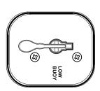
Toggle back the control lever to lower the coach by about four inches. Returning the lever to the normal (forward) position raises the vehicle back to its normal height.
