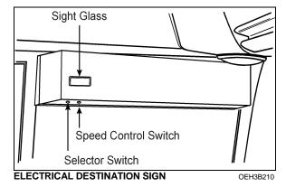
**Note:** Use the servo control switch to change the speed of the destination sign. Use high speed to search for the desired destination and slow speed to align the arrow in the sight glass.
