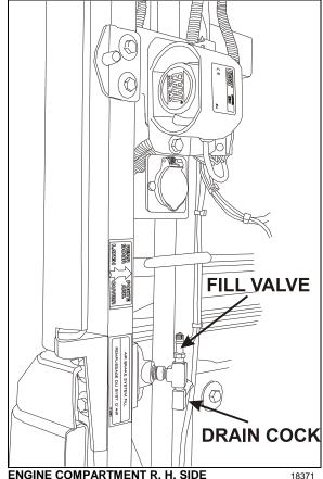
Drain tanks by turning cocks counterclockwise.
