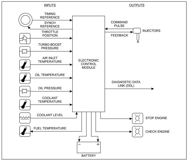
SHEMATIC DIAGRAM OF DDEC IV SYSTEM
