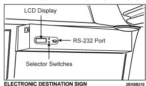
**Note:** The destination sign must be programmed with a computer connected to the RS-232 connector prior to first use. Follow the instructions on the computer disk to install and run the software.
