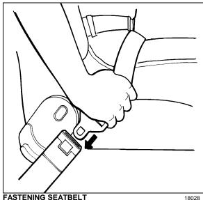
**Note:** The safety belt must be pulled out slowly and continuously, otherwise it will lock the reel before the latch plate reaches the buckle. If this happens, allow the belt to retract completely and repeat the procedure correctly.
