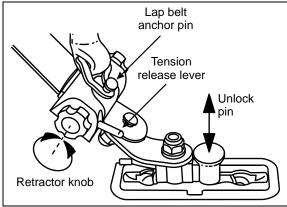
BELT ANCHORING AND RETRACTION SYSTEMS
