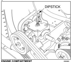
Check radiator fan gear box oil level as follows:
