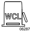
Illuminates when the wheelchair lift compartment door and/or the wheelchair access door are open. The parking brake is activated when this door is open. Refer to Other Features chapter.
