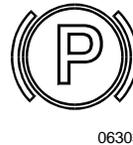
Illuminates when the emergency /parking brake is applied. The control valve is located on the L.H. control panel. An audible alert will sound if ignition is turned to OFF and the parking brake is not engaged.
