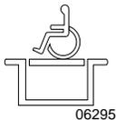
Illuminates when the wheelchair lift is enabled.
