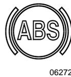
Illuminates when the ABS is not available or when the ABS is malfunctioning. Since the ABS system does not operate under 4 mph (7 km/h), the indicator will remain illuminated until the coach reaches that speed. Refer to "Other Features" chapter
