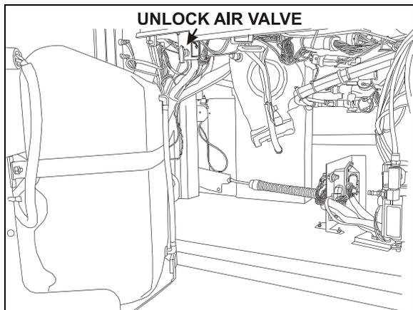
FRONT SERVICE COMPARTMENT UNLOCK AIR VALVE
