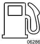
Illuminates when approximately 12 US gallons (45 liters) of fuel remain in the tank. After the light comes ON, the remaining fuel will provide less than 60 miles (100 km) of travel. Do not exceed this distance. Refuel as soon as possible.
