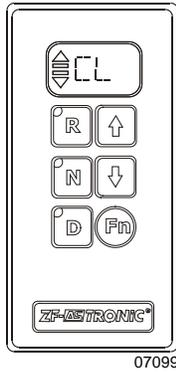
“CL” is displayed if there is a risk of clutch overload resulting from several starting processes occurring in a rapid succession or when running very slow in a starting gear too high.
