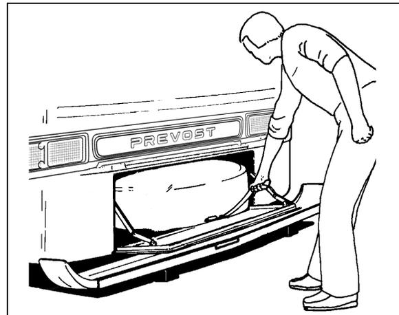
REMOVING SPARE WHEEL AND TIRE
