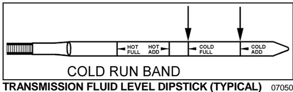
**Caution:** The oil level rises as oil temperature rises. Do not add oil above the "cold run" band before the transmission reaches 180°F to 220°F (82°C to 104°C).
