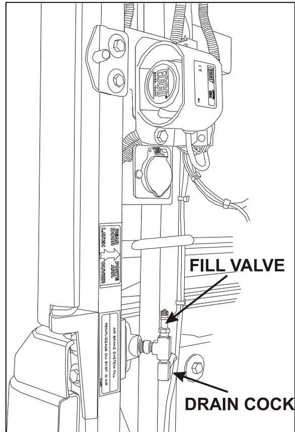
FILL VALVE IN ENGINE COMPARTMENT
