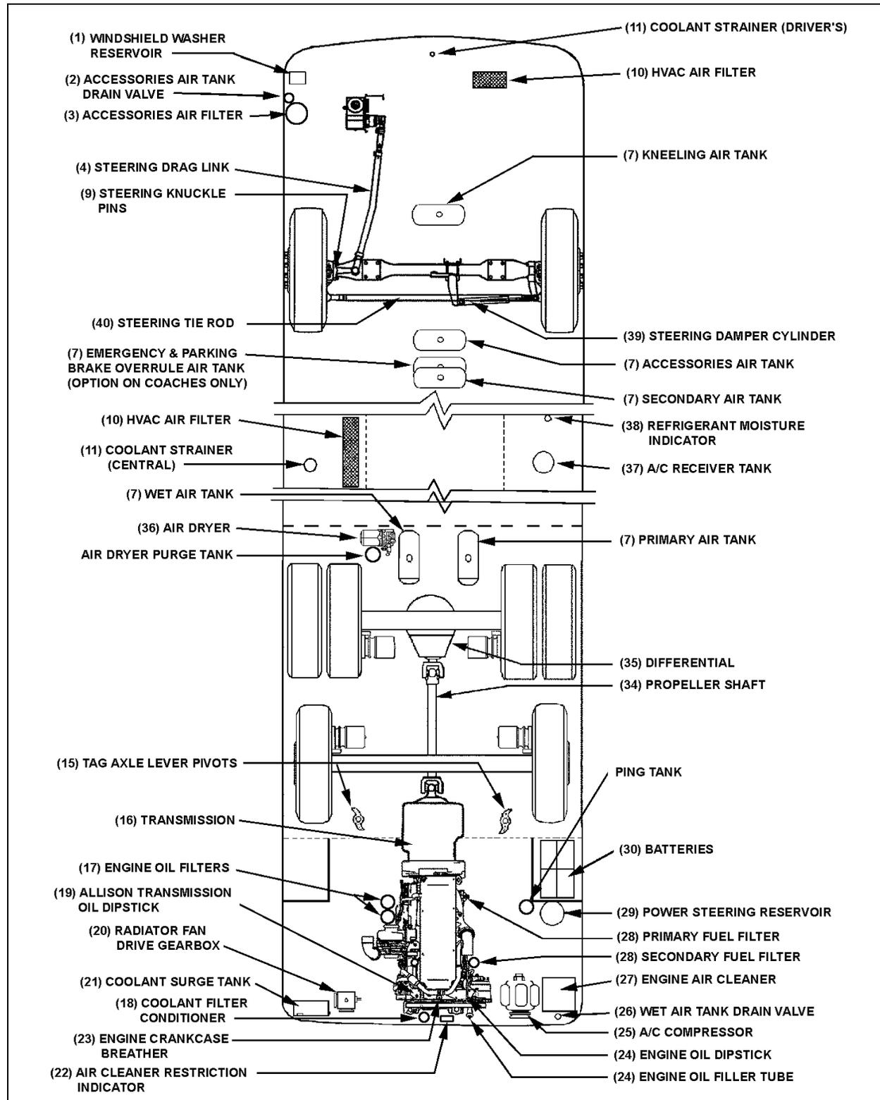
LUBRICATION AND SERVICING POINTS ON I-BEAM FRONT SUSPENSION VEHICLES
