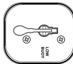
Toggle back the control lever to lower the coach by about four inches. Returning the lever to the normal (forward) position raises the vehicle back to its normal height.
