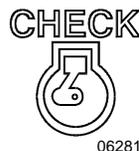
Illuminates when the ignition switch is ON as a light bulb check. The light should turn OFF after five seconds. If the indicator remains
