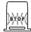
Illuminates when rear stoptlights illuminate. This occurs when either cruise control DECEL switch, service brake, parking brake, engine brake or transmission retarder is applied.
