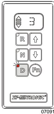
If the vehicle rolls forward with transmission in neutral “N” after that the brake is released and the driver shifts from “N” to “D”, the system selects a gear suitable for the running speed.
