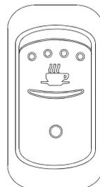
This switch activates the galley's electrical circuit.
