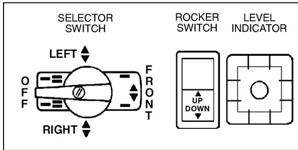
When driving, the conventional air leveling system of the vehicle controls the height at three points: the front, the left rear and the right rear. Your vehicle is equipped with a suspension system that consists of air springs (pressurized air bellows) located near each wheel. The amount of air in each air spring (and thus the vehicle height) is controlled by automatic leveling valves that operate between the chassis and the axles of the vehicle.
