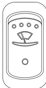
Press the rocker switch to the first position to activate the upper wipers intermittently.
