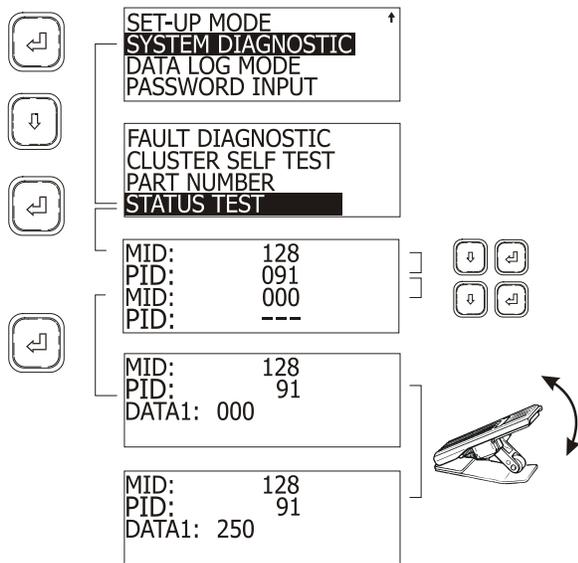
In this example, a throttle pedal in good working order will send a linear and continuous (no jumps) signal to the ECU, appearing as DATA value on the MCD screen. Full pedal movement will display values from 000 (no throttle) to 250 (maximum throttle).
