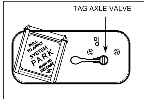
TAG AXLE VALVE ON LEFT LATERAL CONTROL PANEL
