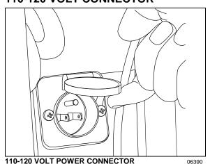
The optional 110-120 volt power connector is located on the engine compartment R.H. side access door. Refer to "Vehicle Exterior" chapter 1. Connect the female end of an extension cord to the male connector. Connect the plug at the other end of the cord to a 110-120 VAC outlet only.
