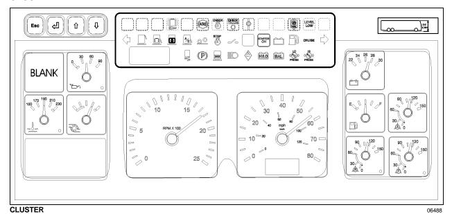
The cluster incorporates the Message Center Display, the Telltale Panel, the Gauges and Vehicle Clearance Information.
