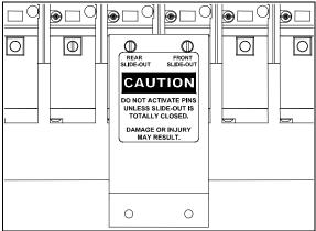
LOCKING PIN VALVE PROTECTION PLATE
