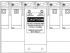
LOCKING PIN VALVE PROTECTION PLATE
