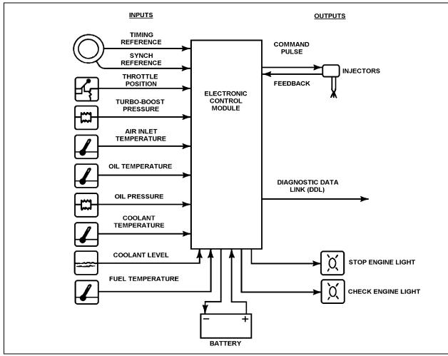
SHEMATIC DIAGRAM OF DDEC IV SYSTEM
