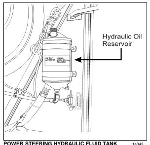
POWER STEERING HYDRAULIC FLUID TANK
