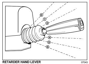
With the retarder activated (retarder switch depressed) and the accelerator pedal released, move the output retarder lever clockwise from the first to the sixth position. The efficiency for each position is as follows:
