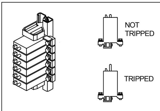
BREAKERS IN SLIDE-OUT CONTROL COMPARTMENT
