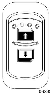
Use the rocker switch to open or close the driver's power window. The switch for the power window in the entrance door is on the R.H. dashboard panel.
