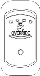
Press down this switch and release to override emergency engine shut down protection. Engine emergency shut down will be turned **OFF** for 30 seconds. This procedure can be repeated if done before the 30 seconds are up.
