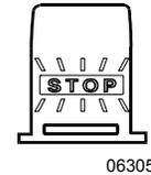
Illuminates when rear stop lights illuminate. This occurs when either cruise control DECEL switch, service brakes, parking brakes, engine retarder or transmission retarder is applied.
