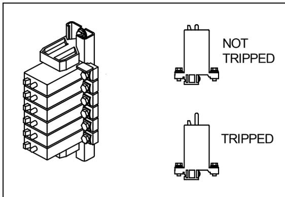
BREAKERS IN SLIDE-OUT CONTROL COMPARTMENT
