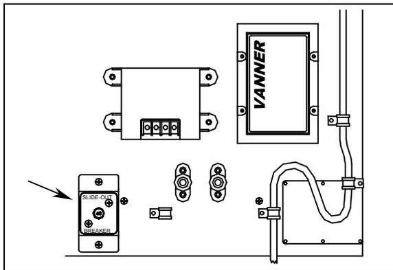
MAIN SLIDE-OUT BREAKER IN MAIN POWER COMPARTMENT
