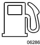
Illuminates when approximately 12 US gallons (45 liters) of fuel remain in the tank. After the light comes ON, the remaining fuel will provide less than 60 miles (100 km) of travel. Do not exceed this distance.
