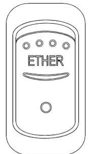
Activates the engine cold starting aid. Refer to "Starting and Stopping Procedures" chapter.
