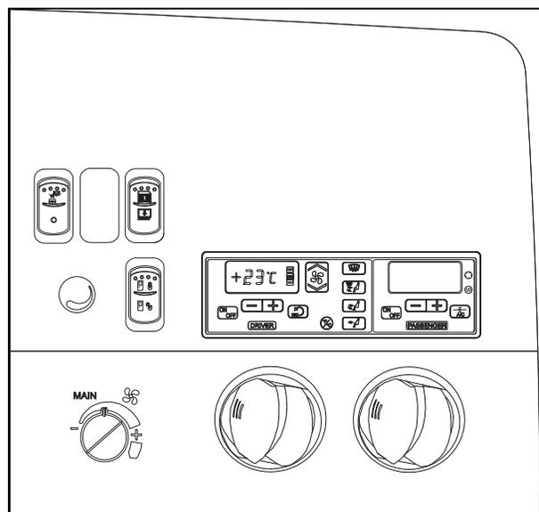
The HVAC control module as well as the cluster dimmer switch, miscellaneous control switches and air vents, are located in the R.H. dashboard panel.
