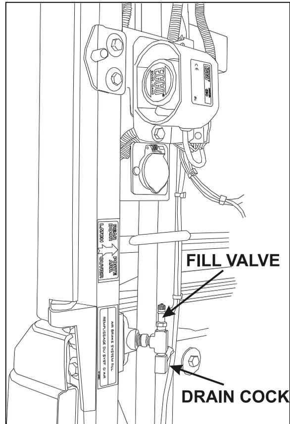
FILL VALVE IN ENGINE COMPARTMENT
