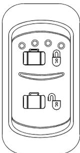
This system enables locking all compartments and doors by pressing down on the upper portion of the switch. To unlock all compartments, press down on the lower portion of the switch.
