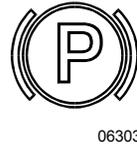
Illuminates when the emergency /parking brake is applied. The control valve is located on the L.H. control panel. A buzzer will sound if ignition is turned to OFF and the parking brake is not engaged.
