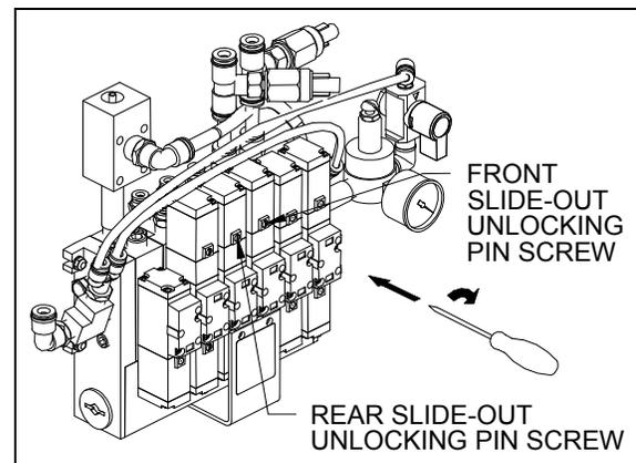
b) Ensure the ignition key is in the "OFF" position. When the proper valve has been identified (right side for front slide-out and left side for rear slide-out), turn clockwise the "pin valve manual override screw" to actuate the locking pins. Keep the override screw in this position. During the process, you should hear a hissing sound, as the air flows to the pin cylinders.
