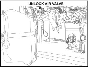
FRONT SERVICE COMPARTMENT UNLOCK AIR VALVE
