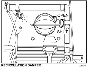
In the evaporator compartment, open or close the recirculation damper with the lever shown in the illustration above.
