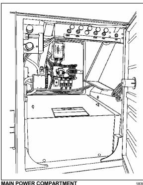
Lights in the compartment will turn *ON* automatically and also a dashboard telltale light will illuminate when the door is opened.
