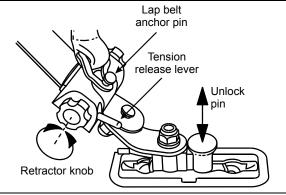
BELT ANCHORING AND RETRACTION SYSTEMS
