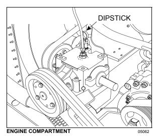
Check radiator fan gear box oil level as follows:
