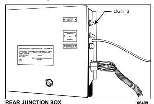
Turn the lights ON in the engine compartment using the switch on the right-hand side of the rear junction box.
