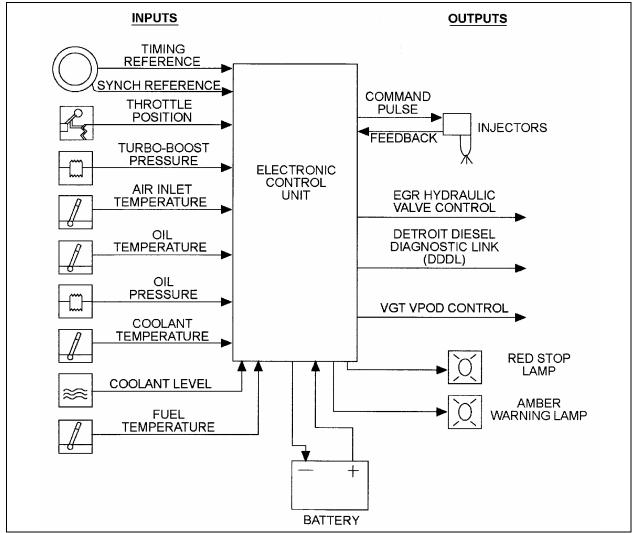
SCHEMATIC DIAGRAM OF DDEC V SYSTEM
