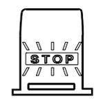
06305 Illuminates when rear stoptlights illuminate. This occurs when either cruise control DECEL switch, service brake, parking brake, engine brake or transmission retarder is applied.
