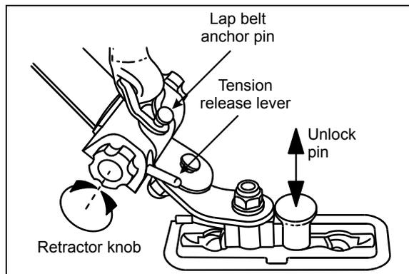
**BELT ANCHORING AND RETRACTION SYSTEMS**
