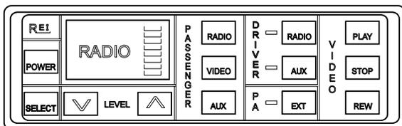
The control head enables the driver to independently control audio entertainment and volume level in the passenger and driver's areas. The video cassette player, the P.A. system and auxiliary systems, such as a DVD player are also controlled by the control head panel.
