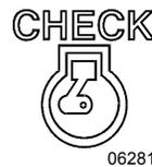
Illuminates when the ignition switch is ON as a light bulb check. The light should turn OFF after five seconds. If the indicator remains ON after five seconds or comes
