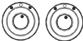
Turn left pointer knob counterclockwise for flat mirror adjustments and to the right for convex mirror adjustments, then use the joystick control to adjust the selected mirror's viewing angle. Adjust the right outside mirror similarly but by using the right side control.
