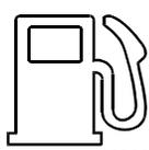
06286 Illuminates when approximately 12 US gallons (45 liters) of fuel remain in the tank. After the light comes ON, the remaining fuel will provide less than 60 miles (100 km) of travel. Do not exceed this distance. Refuel as soon as possible.
