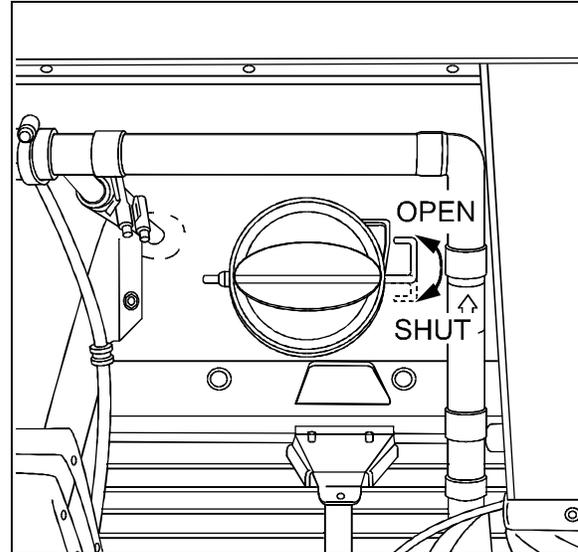
RECIRCULATION DAMPER IN HVAC COMPARTMENT
