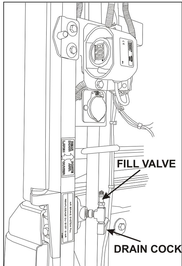
FILL VALVE IN ENGINE COMPARTMENT
