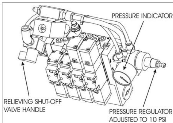
INFLATABLE SEAL RELIEVING SHUT-OFF VALVE
