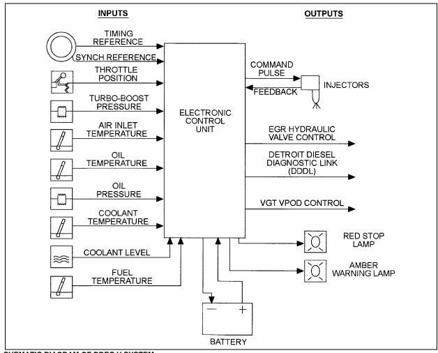
SHEMATIC DIAGRAM OF DDEC V SYSTEM
