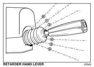
With the retarder activated (retarder switch depressed) and the accelerator pedal released, move the output retarder lever clockwise from the first to the sixth position. The efficiency for
