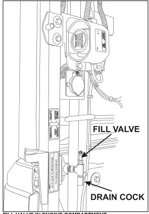
FILL VALVE IN ENGINE COMPARTMENT
