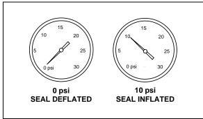
**INFLATABLE SEAL PRESSURE GAGE**
