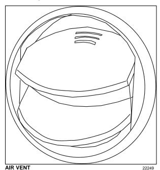
Three adjustable driver air vents in the dashboard and one near the door feed air to the driver's compartment. Use the HVAC control panel to set air temperature.
