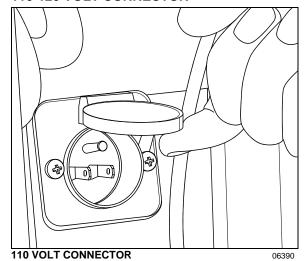
This connector is used with a 110-120 volt supply and is connected to the engine block heater. Refer to "Starting and Stopping Procedures" chapter.
