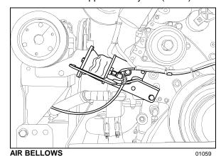
For belt replacement, air pressure must be released from bellows by means of the belt tensioning pressure control valve. This valve, mounted close to the pressure regulating valve, is manually operated. Before handling, be sure that all engine stopping safety precautions have been observed.
