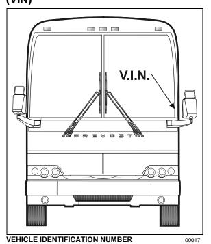
The Vehicle Identification Number is stamped on a plate located on the windshield frame pillar (driver's side). The VIN is visible from the outside of the vehicle. Make sure the correct vehicle identification number is given when ordering replacement parts. Using the VIN when ordering parts will facilitate processing.
