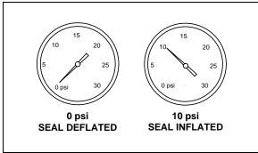
**INFLATABLE SEAL PRESSURE GAGE**
