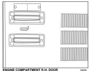
This door can be locked or unlocked using the exterior compartment key or, if so equipped, by the central door locking system. To open, push sideways the small lever located between the marker lights.
