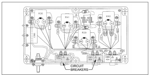
FIGURE 3: CB5 AND CB9 CIRCUIT BREAKERS AND RELAYS R29, R40, R41
