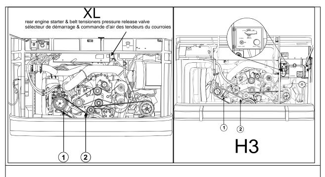
FIGURE 1 : FAN DRIVE ASSEMBLY COMPONENTS : (1) STOP; (2) DRIVING BELTS IN INSET : REAR ENGINE STARTER SELECTOR SWITCH AND BELT TENSIONERS PRESSURE RELEASE VALVE
