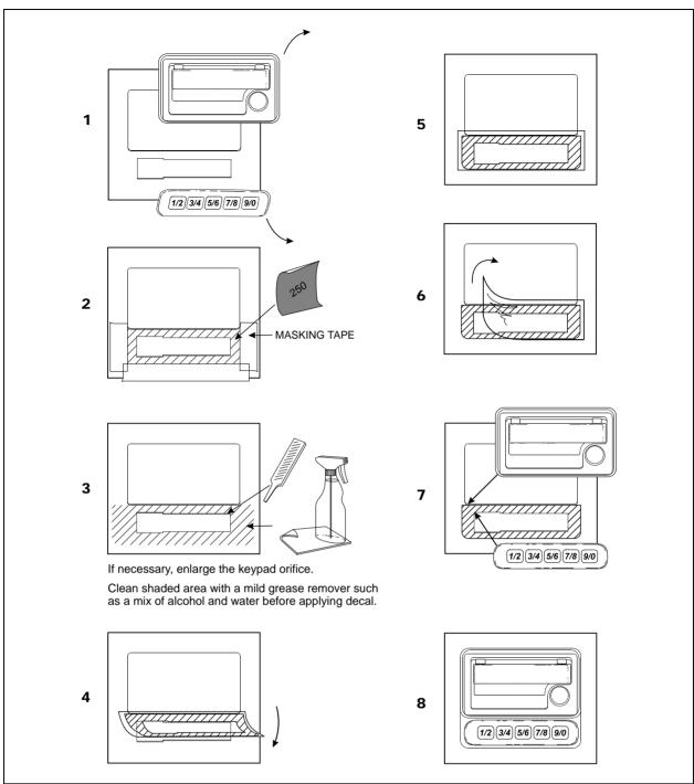
FIGURE 1: INSTALLATION OF THE DECAL AND KEYPAD ON H3-45 VIP
