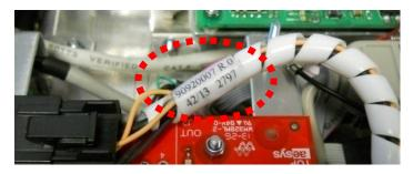
Figure 8-2: example of code and release imprinted on a wiring cable
