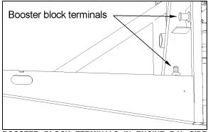
BOOSTER BLOCK TERMINALS IN ENGINE R.H. SIDE ACCESS COMPARTMENT 18595
