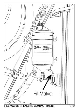
Both air system emergency fill valves are fitted with standard tire valve stems. The air systems can be filled using any standard external air supply line. The fill valve located in the engine compartment supplies air for all systems (brakes, suspension and accessories). The fill valve located in the service compartment supplies air for accessories only.
