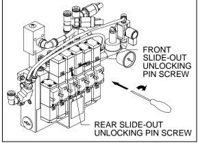
UNLOCKING PIN VALVE LOCATION
