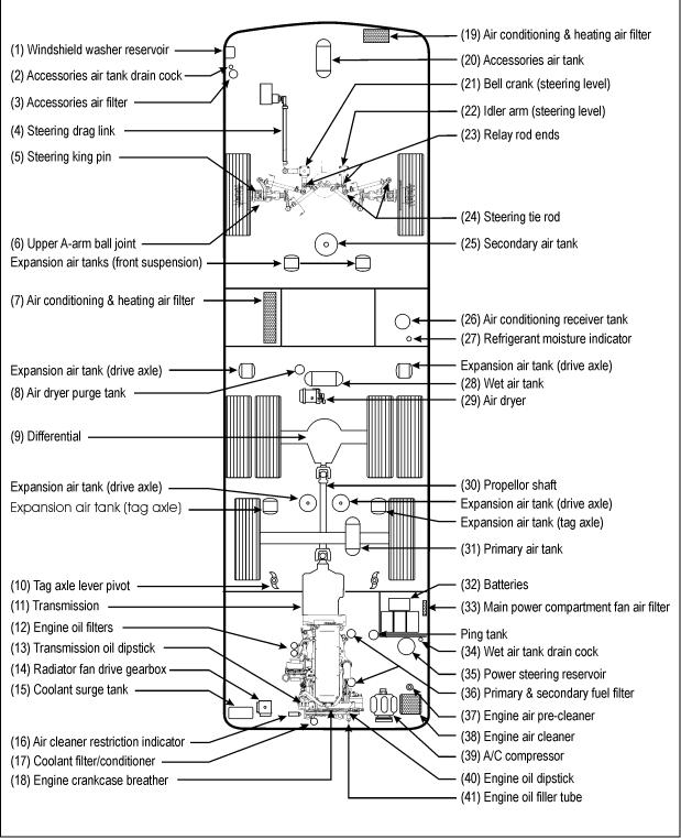
LUBRICATION AND SERVICING POINTS ON INDEPENDENT FRONT SUSPENSION VEHICLES (TYPICAL)
