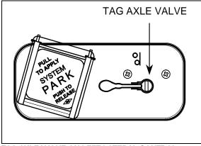
TAG AXLE VALVE ON LEFT LATERAL CONTROL PANEL06390
