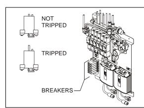
BREAKERS IN SLIDE-OUT CONTROL COMPARTMENT
