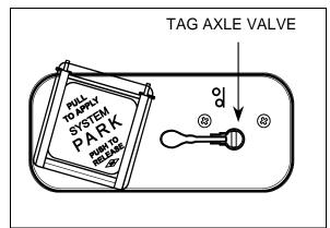
TAG AXLE VALVE ON LEFT LATERAL CONTROL PANEL
