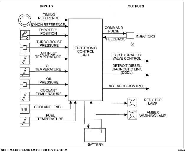
SCHEMATIC DIAGRAM OF DDEC V SYSTEM
