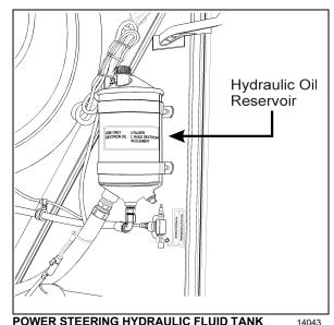
POWER STEERING HYDRAULIC FLUID TANK
