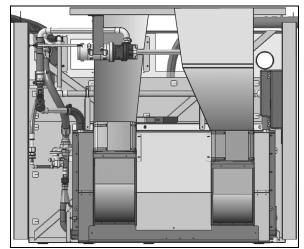
**EVAPORATOR COMPARTMENT (WITH CENTRAL A/C** SYSTEM ONLY)
