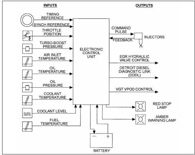
SCHEMATIC DIAGRAM OF DDEC V SYSTEM
