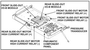
SLIDE-OUT CONTROL PANEL IN FIRST BAGGAGE COMPARTMENT
