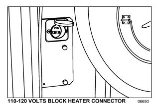
The vehicle is equipped with an engine immersion-type electric block heater to assist cold weather starting. A connector is located on the engine compartment door. Using an extension cord, connect to a 110 - 120 VAC outlet. Use the engine block heater when the vehicle is parked in cold weather for a long period and the proper power source is available.
