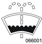
Illuminates when the windshield washer or the headlights washer fluid level is low. The washer fluid containers are located inside the front service compartment.
