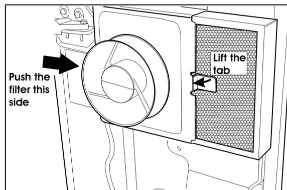
**MAIN POWER COMPARTMENT FAN AIR FILTER REMOVAL** 06603
