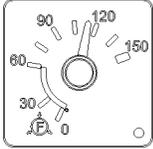
Indicates the secondary air system pressure. The normal operating pressure is from 95 to 125 psi (655 to 860 kPa).
