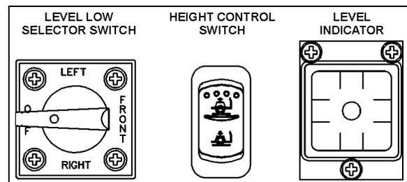
When driving, the conventional air leveling system of the vehicle controls the height at three points: the front, the left rear and the right rear. Your vehicle is equipped with a suspension system that consists of air springs (pressurized air bellows) located near each wheel. The amount of air in each air spring (and thus the vehicle height) is controlled by automatic leveling valves that operate between the chassis and the axles of the vehicle.
