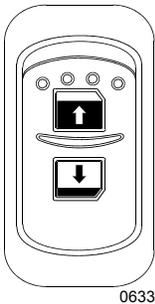
Use the rocker switch to open or close the driver's power window.
