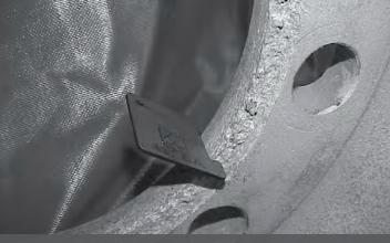
**UNACCEPTABLE** Figure 3-38: Hub Bore Gauge fits indicating severe hub bore corrosion. Remove any severely corroded wheel from service immediately and scrap.
