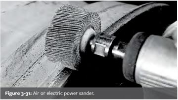
**Air or Electric Powered Sander:** This tool provides a very quick and effective method of removing the sharp edge. Technicians should use care to keep a uniform edge when using these tools (Figure 3-31).
