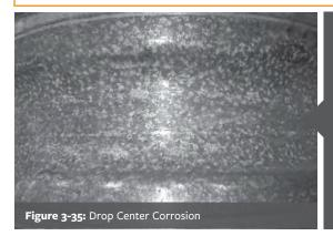
Bead seat and valve stem corrosion often are caused by trapped moisture. Mild corrosion as shown in Figure 3-35 should be removed until thoroughly cleaned. Remove any severely corroded wheel from service immediately and scrap.
