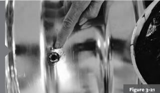
Before installing the valve, apply a thin coat of non-water based tire lubricant on the shaft and base of the valve stem where the O-ring or grommet is located. Do not use any other lubricants that are water-based or contain metals.
