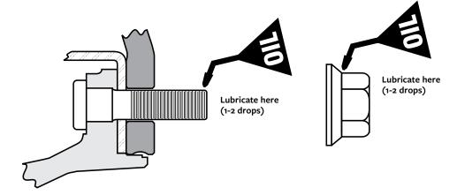
Prior to mounting hub piloted wheels, coat the wheel hub bore. Then push wheels onto the hub so that excess lube will scrape off and not be pushed between the mounting surfaces with a non-water-based lubricant to minimize corrosion and build-up between the wheel and hub pilot. Excessive corrosion build-up between the wheel and hub pilots can make wheel removal difficult. Do not lubricate the face of the wheel, hub or brake drum.
