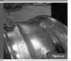
7. Push the tire bead onto the rim as far as possible. Using the curved end of the tire iron (with the stop resting on the rim flange) take small bites to work the remaining section of the bead onto the rim/wheel.
