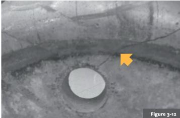
Inspect the hub/drum contact area thoroughly for cracks or other damage.
