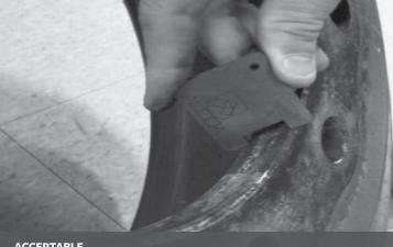
Figure 3-37: Hub Bore Gauge does not fit. This wheel is acceptable for use.
