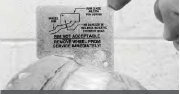
Figure 3-27: Not serviceable (scrap wheel)
