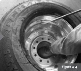
8. Take small bites, repeat the operation progressively around the rim. Keep the tire bead in the well with your foot or with self-locking pliers. Continue until the second tire bead is full mounted over the flange.
