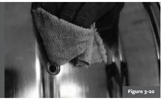
Apply a layer of non-water based tire lubricant in the valve hole and the outer and inner side wheel surface, up to 1 inch or 2 centimeters in diameter around the valve hole.
