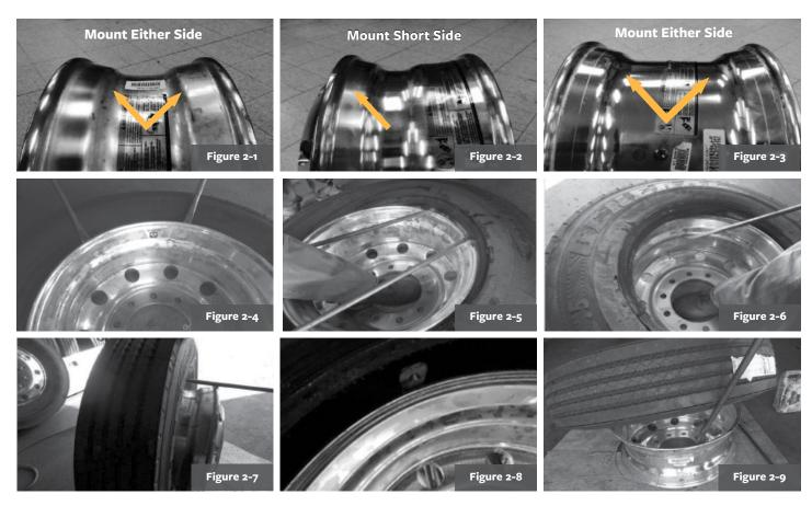
For aluminum wheels, a mat should be placed on the floor to prevent damage to the mounting surface of the wheel.
