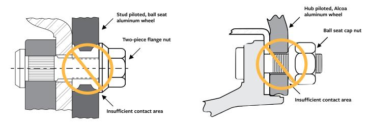
Incorrect use of a ball seat cap nut on a hub piloted system. Do not use ball seat cap nuts with hub piloted wheels.
