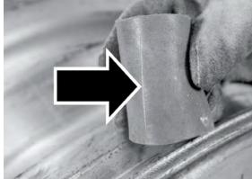
Figure 3-29: Run the sharpness indicator gauge along the wheel in the area of the wear to determine if the wear is sharp enough to cut or damage the rubber on the sharpness indicator.
