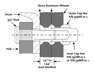
Correct mounting for dual aluminum, stud piloted / ball seat mount wheels.
