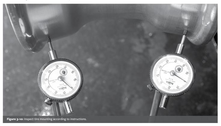
Tire wear can also be caused by improperly seated tires. Inspect the tire for proper seating on the wheel if the tire beads are not seated properly. Remove the wheel from the vehicle, deflate and break the bead seats (see Section 2 for recommendations and instructions for demounting tubeless tires). Adequately lubricate the tire/wheel bead seats and properly re-seat the tire beads. Reinflate the tire in a restraining device. Refer to OSHA rule 1910.177, paragraph b. See Section 6.
