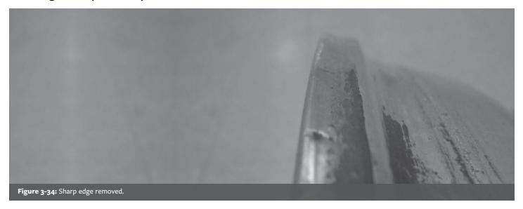
**STEP 4.** Figure 3-34 shows the result of removing the sharp edge on the rim flange. With whatever tool is selected, work the tool around the wheel's circumference removing only enough material to eliminate the sharp edge. This should only be a small amount of metal. Perform this work on both flanges if there is evidence of sharpness. Take care to make sure the edge removal is as uniform as possible and avoid gouging the wheel.
