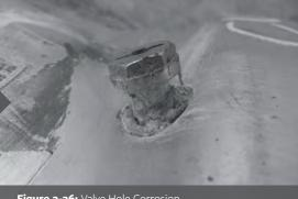
Figure 3-36: Valve Hole Corrosion
