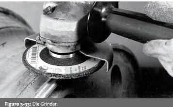
**Die Grinder:** Used with a sanding wheel, cutting stone or grinding tool, this is a version of an electric grinder. This tool is very quick and effective as well, but care must be taken to remove metal as uniformly as possible and not to gouge the wheel (Figure 3-33).
