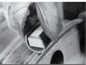
**Figure 3-28:** A rubber sharpness gauge or a suitable piece of rubber attached to a block of wood.
