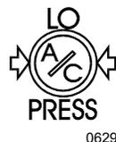
Illuminates when the A/C system pressure is too low. If the A/C pressure is too low, the compressor clutch disengages and the fan stops.
