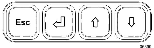
Use the up (↑) and down (↓) arrows to highlight a function or a setting. At any given level, small arrows may appear in the upper and lower right corner of the display. This means that more information is available by scrolling up or down with the arrow keys.
