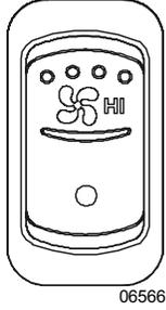
Switches fan speed to HI for cabin ventilation (only available on models equipped with central HVAC).
