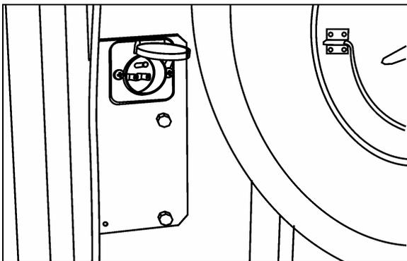
The vehicle is equipped with an engine immersion-type electric block heater to assist cold weather starting. A connector is located on the engine compartment door. Using an extension cord, connect to a 110 - 120 VAC outlet. Use the engine block heater when the vehicle is parked in cold weather for a long period and the proper power source is available.
