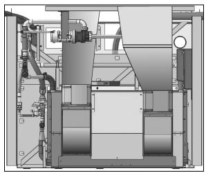
**EVAPORATOR COMPARTMENT (WITH CENTRAL A/C** SYSTEM ONLY)
