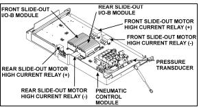
SLIDE-OUT CONTROL PANEL IN FIRST BAGGAGE COMPARTMENT
