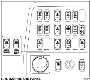
The L.H. dashboard panel includes driver-exclusive controls, ether start control switch, ignition switch and an adjustable air register for the driver.
