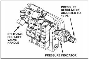
INFLATABLE SEAL RELIEVING SHUT-OFF VALVE
