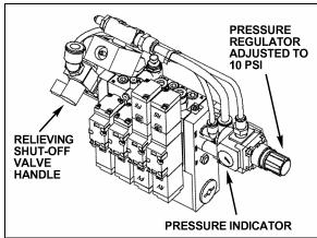
INFLATABLE SEAL RELIEVING SHUT-OFF VALVE 26098
