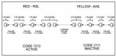
FIGURE 1: FLASHING FAULTS CODES
