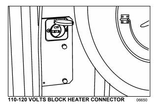
The vehicle is equipped with an engine immersion-type electric block heater to assist cold weather starting. A connector is located on the engine compartment door. Using an extension cord, connect to a 110 - 120 VAC outlet. Use the engine block heater when the vehicle is parked in cold weather for a long period and the proper power source is available.
