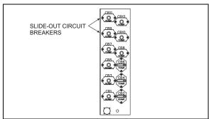
SLIDE-OUT CIRCUIT BREAKERS CB9 & CB11 IN MAIN POWER COMPARTMENT 26091
