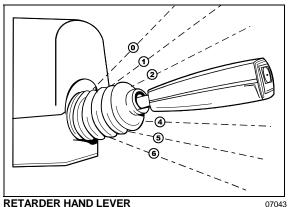
With the retarder enabled and the accelerator pedal released, move the output retarder lever clockwise from the first to the sixth position. The braking level for each position is as follows:
