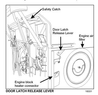
The engine compartment rear door provides access to the following:
