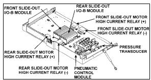
SLIDE-OUT CONTROL PANEL IN FIRST BAGGAGE COMPARTMENT 26107
