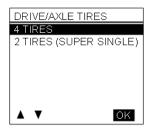
Pressing the up down arrow when the number of tires is highlighted allows flipping the number to 2 or 4 which are the only valid choices.
