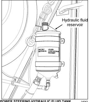
POWER STEERING HYDRAULIC FLUID TANK
