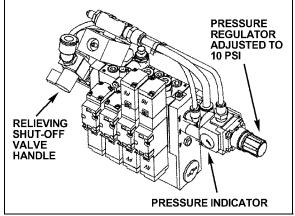
INFLATABLE SEAL RELIEVING SHUT-OFF VALVE 26098
