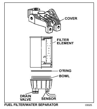
The optional Fuel Pro 382 diesel fuel filter system consists of a permanently mounted fuel processor, a replaceable filter element, a filter element cover and collar and a fluid filter base assembly. This system is installed between the fuel tank and the fuel pump and replaces the primary fuel filter. The filter serves as a water separator as well as a fuel filter. To drain, turn 1/4 turn the drain valve below filter, close when water has been flushed out.
