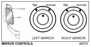
Turn left pointer knob counterclockwise for flat mirror adjustments and to the right for convex mirror adjustments, then use the joystick control to adjust the selected mirror's viewing angle. Adjust the right outside mirror similarly but by using the right side control.
