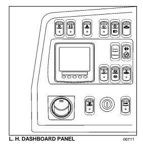
The L.H. dashboard panel includes driver-exclusive controls, ether start control switch, ignition switch and an adjustable air register for the driver.
