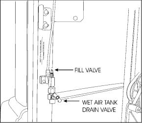
FILL VALVE IN ENGINE R.H. SIDE COMPARTMENT 12219
