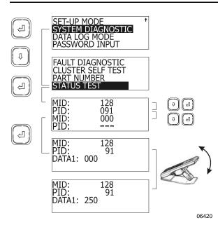
In this example, a throttle pedal in good working order will send a linear and continuous (no jumps) signal to the ECM, appearing as DATA value on the MCD screen. Full pedal movement will display values from 000 (no throttle) to 250 (maximum throttle).
