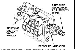
INFLATABLE SEAL RELIEVING SHUT-OFF VALVE 26098
