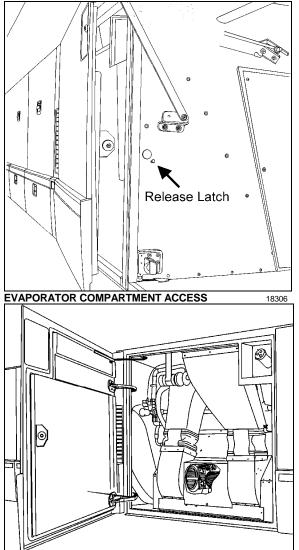
EVAPORATOR COMPARTMENT (WITH CENTRAL A/C SYSTEM ONLY) 22365
