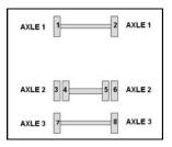
The sequence increments to the next wheel on the same axle counting wheels from left to right and then moves to the next axle counting axles from front to rear. The display activates the next wheel parameter each time a wheel is done. This parameter is use by the vehicle electronic to activate an audible signal on the vehicle thus providing a feedback to the user that he can move to the next wheel.
