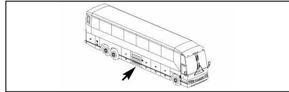
Pull the release latch located inside the adjacent baggage compartment to open the condenser door.
