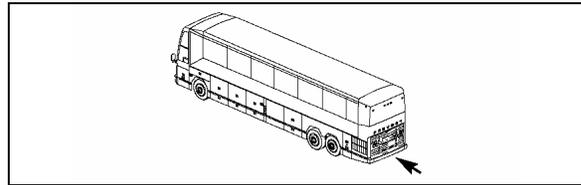
To open the rear engine door, first open the curb side door then press the release lever. The rear door release lever is located in the upper rear section of the engine compartment, as seen when looking into the curb side engine compartment. Unlatch the door and pull it out and up. The door should stay open on it's own but it is recommended to always use the safety catch as shown.
