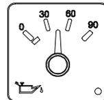
Indicates engine oil pressure. The normal reading should be between 50 and 70 psi (345 - 480 kPa) at 55 mph (90 km/h).
