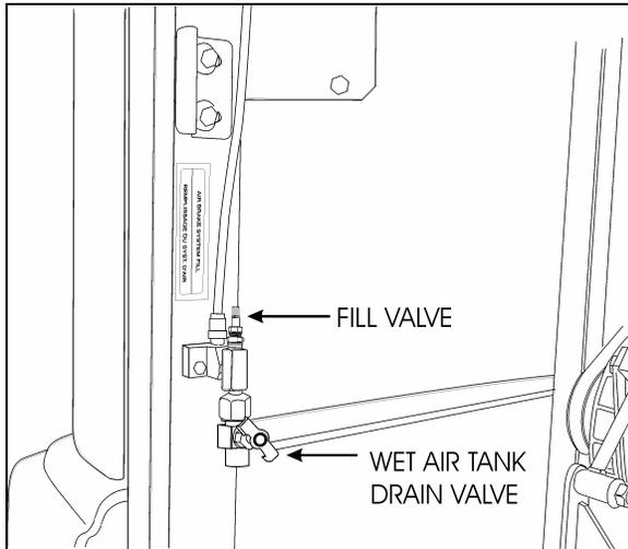
**FILL VALVE IN ENGINE COMPARTMENT** 12219
