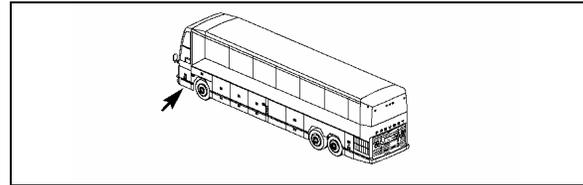
The front electrical and service compartment provides access to the following:
