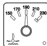
Indicates the operating temperature of the engine coolant. The normal reading should be between 190°F and 222°F (88°C to 106°C).
