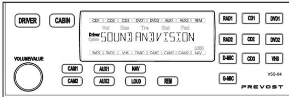
The VSS-04 Multichannel Sound Selector enables the driver to select audio and video entertainment with independent settings of volume level, bass, treble, etc. in the passenger and driver's areas. The dashboard radio, DVD player, video cassette player, the P.A. system, auxiliary systems and other components are controlled by this unit.
