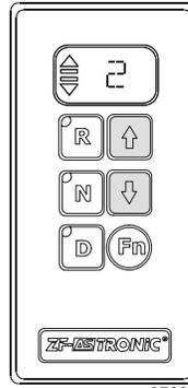
The system selects 2<sup>nd</sup> starting gear as default. The driver may select 1<sup>st</sup> starting gear.
