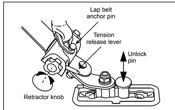
**BELT ANCHORING AND RETRACTION SYSTEMS**
