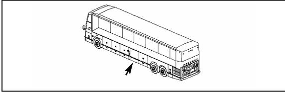
To access the evaporator compartment, pull the release latch located on the left side wall of the rearmost baggage compartment.
