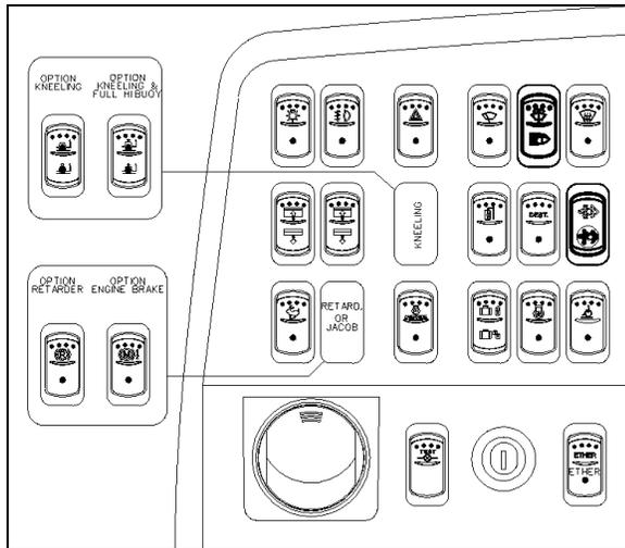
The L.H. dashboard panel includes controls for the operation of the coach, it also includes the ether start control, the ignition switch and an adjustable air register.
