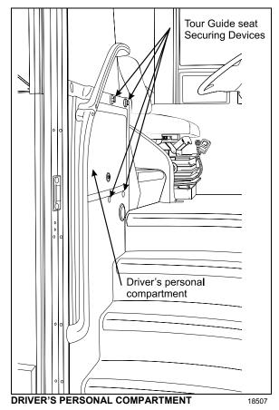
A lockable compartment for the driver is located on the L.H. side of the entrance stepwell. This compartment may be locked using the appropriate key. A tour guide seat is available as an option and is installed in front of the driver's
