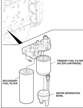
**FUEL FILTERS WITH VOLVO D13 ENGINE**
