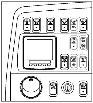
The L.H. dashboard panel includes controls for the operation of the coach; it also includes the ether start control, the ignition switch and an adjustable air register.
