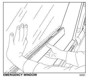
To close, lift the release bar and pull the window into position. Push down on release bar to lock the window shut.
