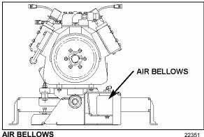
For belt replacement, air pressure must be released from bellows by means of the belt tensioning pressure control valve. This valve, mounted close to the pressure regulating valve, is manually operated. Before handling, be sure that all engine stopping safety precautions have been observed.
