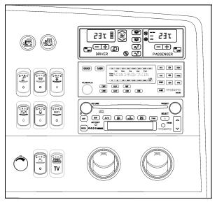
Controls for passenger comfort and entertainment are grouped on this panel. The HVAC control module as well as the cluster dimmer switch, miscellaneous control switches and air vents are therefore located on the R.H. dashboard panel.
