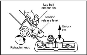
BELT ANCHORING AND RETRACTION SYSTEMS
