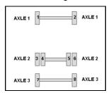
The sequence increments to the next wheel on the same axle counting wheels from left to right and then moves to the next axle counting axles from front to rear.
