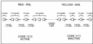
FIGURE 1: FLASHING FAULTS CODES
