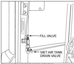
FILL VALVE IN ENGINE COMPARTMENT
