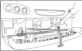
REMOVING SPARE WHEEL AND TIRE
