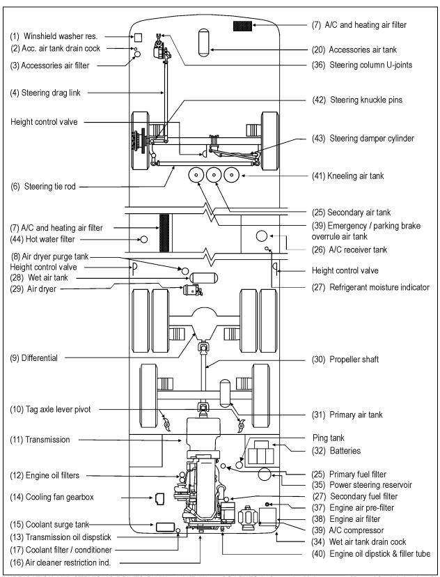
LUBRICATION AND SERVICING POINTS ON H3-41 AND H3-45 COACHES (refer to the Maintenance Manual for Iubrication & servicing schedule)
