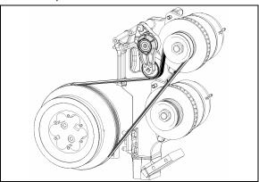
LIMP-HOME BELT ON TOP ALTERNATOR (WITH VOLVO D13 ENGINE) 01194
