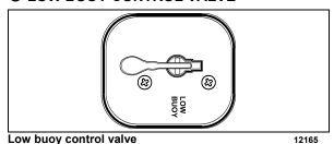
Toggle back the control lever to lower the coach by about four inches. Returning the lever to the normal (forward) position raises the vehicle back to its normal height.
