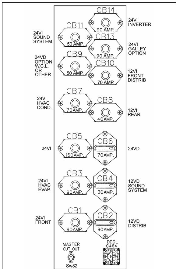
REAR ELECTRICAL COMPARTMENT SAFETY SWITCH<sup>06621</sup>
