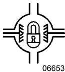
Illuminates when the differential action is locked
