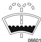
Illuminates when the windshield washer or the headlights washer fluid level is low. The washer fluid reservoirs are located inside the front service compartment.
