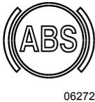
Illuminates when the ABS is not available or when the ABS is malfunctioning. Since the ABS system does not operate at less than 4 mph (7 km/h), the indicator will remain illuminated until the coach reaches that speed. Refer to "Other Features" chapter.
