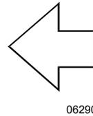
Flashes when the left turn signals are activated. Signal right and left turns by operating the multi-function lever. See Steering Column Controls in this chapter.
