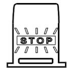
Illuminates when rear stoplights illuminate. This occurs when service brake, engine brake or transmission retarder is applied and when the parking brakes are applied with engine running.
