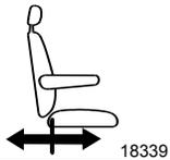
To adjust distance between driver and dashboard, pull handle #5 up and slide the seat forward or backward.
