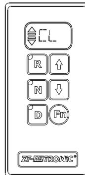
"CL" is displayed if there is a risk of clutch overload resulting from several starting processes occurring in a rapid succession or when running very slow in a starting gear too high.
