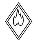
Illuminates if a fire is detected in the engine compartment while the vehicle is on the road. An audible alert informs the driver when a fire is detected. In case of fire detection when parked (parking brake applied, engine running or not), the electric horn is activated to alert the driver. Refer to Safety Features and Equipment chapter.
