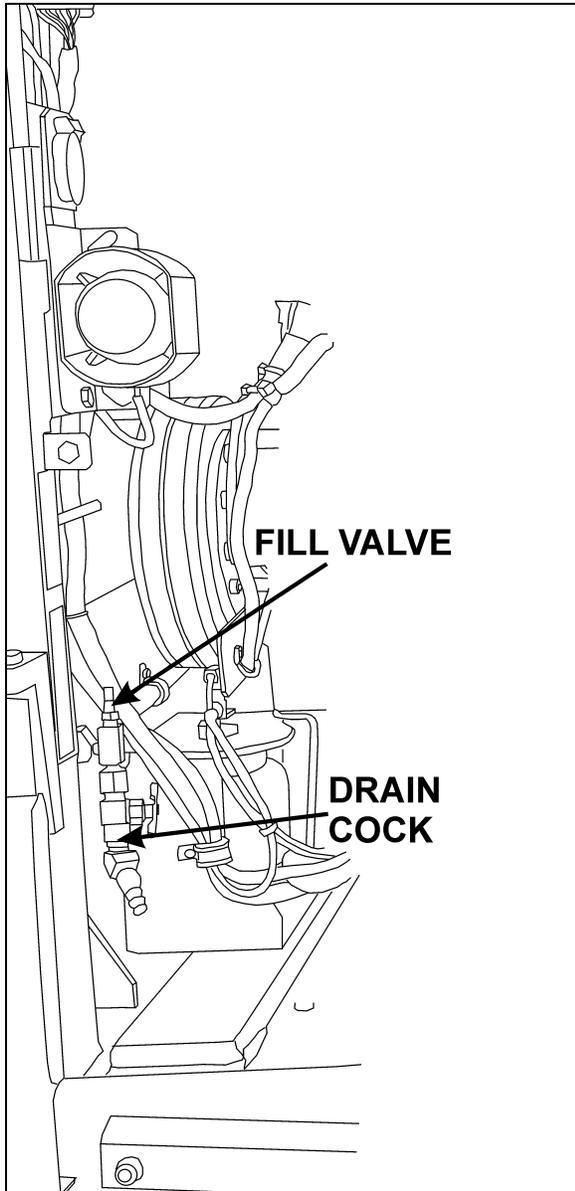
FILL VALVE IN ENGINE COMPARTMENT
