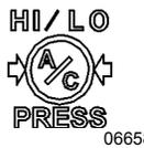
Illuminates when the A/C system pressure is too low or too high. If the A/C pressure is too low, the compressor clutch disengages and the fan stops.
