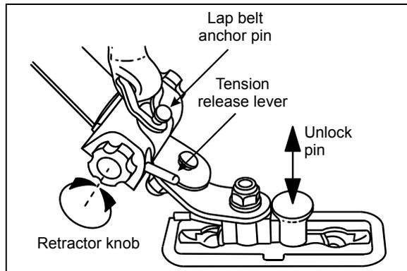
BELT ANCHORING AND RETRACTION SYSTEMS 23266
