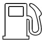
Illuminates when approximately 12 US gallons (45 liters) of fuel remains in the tank. After the light comes ON, the remaining fuel will provide no more than 60 miles (100 km) of travel. Do not exceed this distance.
