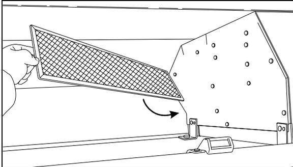
OVERHEAD COMPARTMENT FAN AIR FILTER
