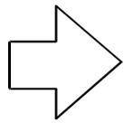
Flashes when the right turn signals are activated. Signal right and left turns by operating the multi-function lever. See Steering Column Controls in this chapter.
