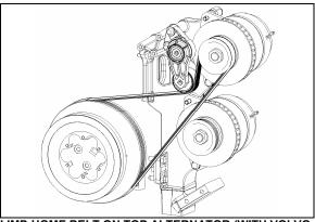
LIMP-HOME BELT ON TOP ALTERNATOR (WITH VOLVO D13 ENGINE)
