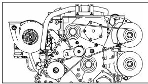
LIMP-HOME BELT ON TOP ALTERNATOR (WITH DDC S60 ENGINE) 01154
