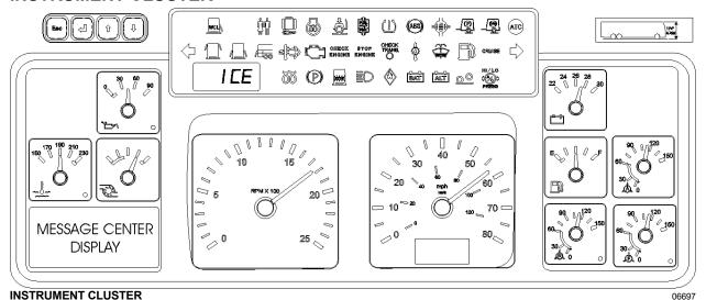
The instrument cluster incorporates the Message Center Display, the Telltale Panel, the Gauges and Vehicle Clearance Information.
