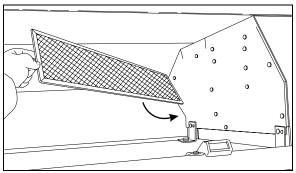
OVERHEAD COMPARTMENT FAN AIR FILTER
