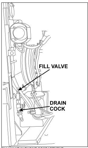
FILL VALVE IN ENGINE COMPARTMENT
