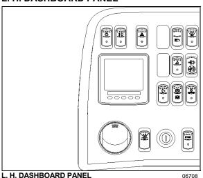
The L.H. dashboard panel includes controls for the operation of the coach; it also includes the ether start control, the ignition switch and an adjustable air vent.
