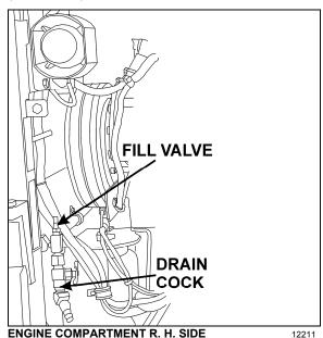
The accessory air tank drain cock is accessible from the front service compartment.
