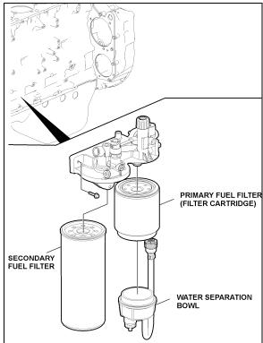
**FUEL FILTERS WITH VOLVO D13 ENGINE**
