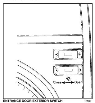
From the inside, open the door by pressing the door opening switch (L.H. button) on the R.H. dashboard panel. Close by pressing the door closing switch (R.H. button) on the dashboard. Refer to "Controls and Instruments" chapter for more information.
