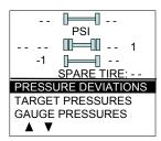
As illustrated, the pressure readings will appear replacing the dash lines as the TPMS display starts to receive pressure data from the TPMS receiver. It can take 1 minute to get all pressure readings updated since the sensors transmit at a one minute interval.
