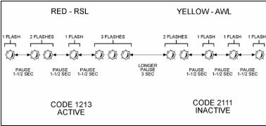
Figure 1: flashing faults codes
