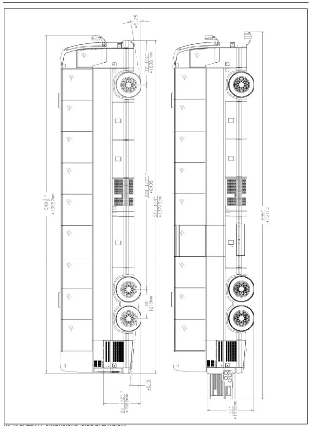
X3-45 OVERALL DIMENSIONS (SIDE ELEVATION)
