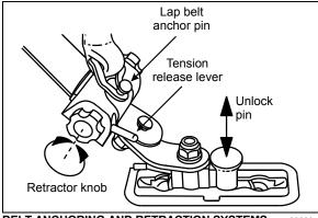
BELT ANCHORING AND RETRACTION SYSTEMS
