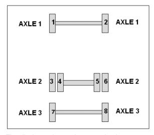
The display activates the next wheel parameter each time a wheel is done. This parameter is use by the vehicle electronic to activate an audible signal on the vehicle thus providing a feedback to the user that he can move to the next wheel.
