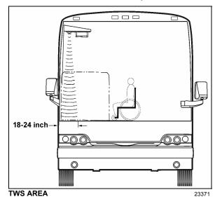
Turn power to lift on (LED on TWS module will light steady) and indicator light on the control device illuminates. If wheelchair and passenger are detected by acoustic sensors the LED will flash, the buzzer will sound and the module red light will flash. If this occurs it is necessary to adjust aiming of sensors.  Turn sensor angle adjustment screw clockwise to move direction of beam away from center aisle and towards doorway. Stop adjustment when LED ceases to flash.
