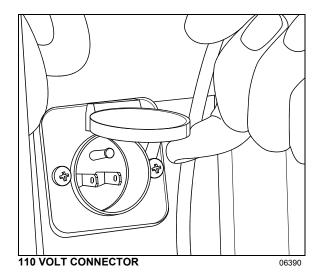
To access the connector, open the engine compartment R. H. side door. The connector is attached to the L. H. side frame post.
