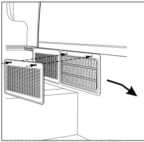
ACCESS TO DRIVER'S HVAC UNIT AIR FILTERS
