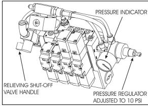
INFLATABLE SEAL RELIEVING SHUT-OFF VALVE
