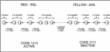
Figure 1: flashing faults codes
