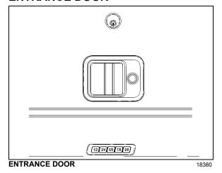
Lock or unlock the entrance door from outside the vehicle by either turning the key in the door
