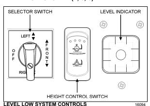
During driving, the conventional air leveling system of the vehicle controls the height at three points: the front, the left rear and the right rear. Your vehicle is equipped with a suspension system that consists of air springs (pressurized air bellows) located near each wheel. The amount of air in each air spring (and thus the vehicle height) is controlled by automatic leveling valves that operate between the chassis and the axles of the vehicle.
