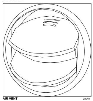
Three adjustable driver air vents in the dashboard feed air to the driver's area. Use the HVAC control module to set air temperature.
