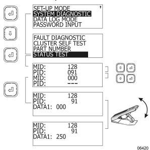
In this example, a throttle pedal in good working order will send a linear and continuous (no jumps) signal to the ECM, appearing as DATA value on the MCD screen. Full pedal movement will display values from 000 (no throttle) to 250 (maximum throttle).
