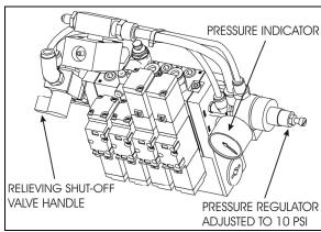
INFLATABLE SEAL RELIEVING SHUT-OFF VALVE
