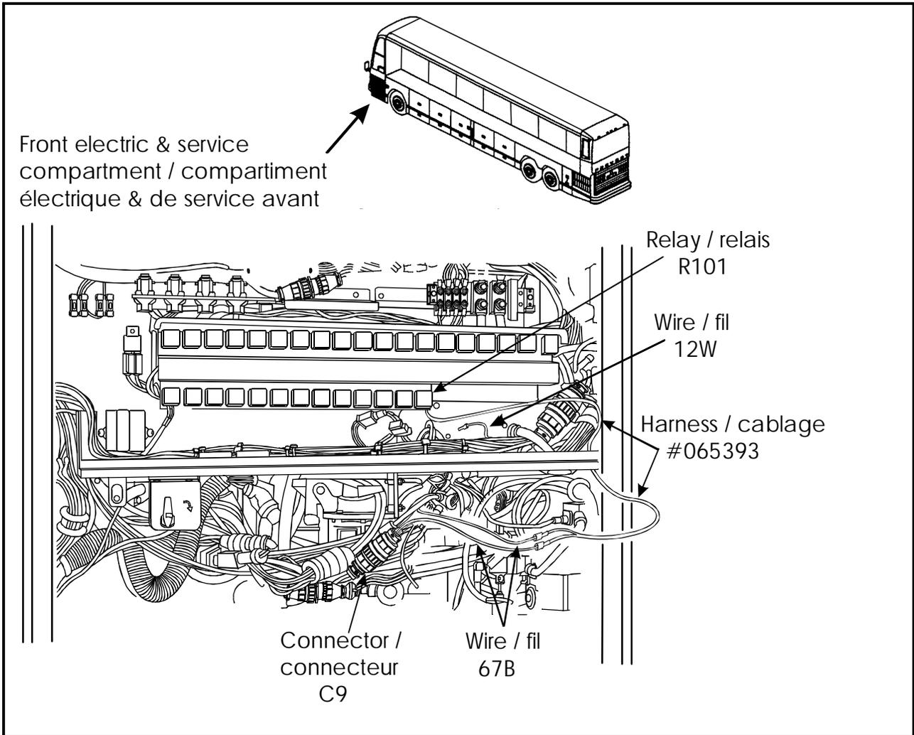
FIGURE 1 : FRONT ELECTRIC AND SERVICE COMPARTMENT
