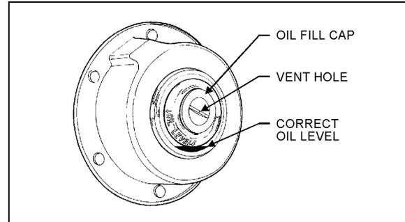
WHEEL BEARING LUBRICATION
