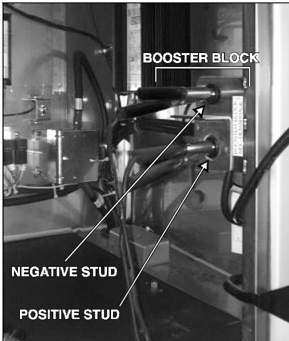
1. Remove the protective caps from the booster block posts, located in main power compartment.
