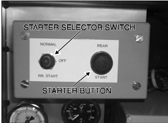
**Warning:** Before attempting to start engine from engine compartment, make sure parking brake is applied and transmission is in neutral.
