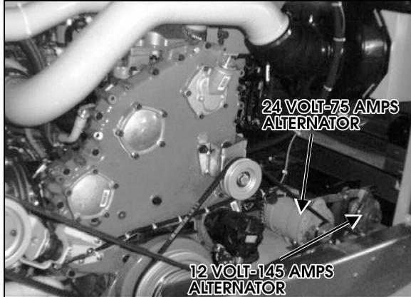
FIGURE 74: ENGINE REAR COMPARTMENT (ALTERNATOR)
