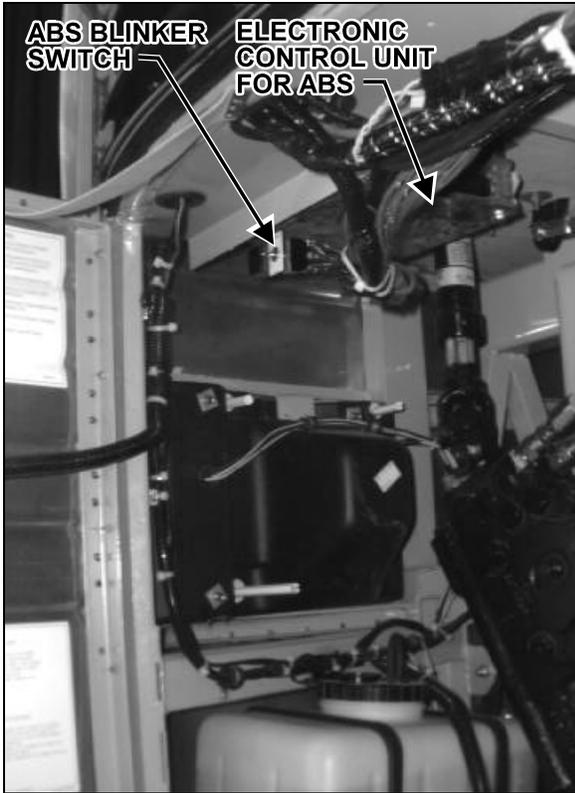
FIGURE 9: STEERING COMPARTMENT (LEFT WALL) 06119
