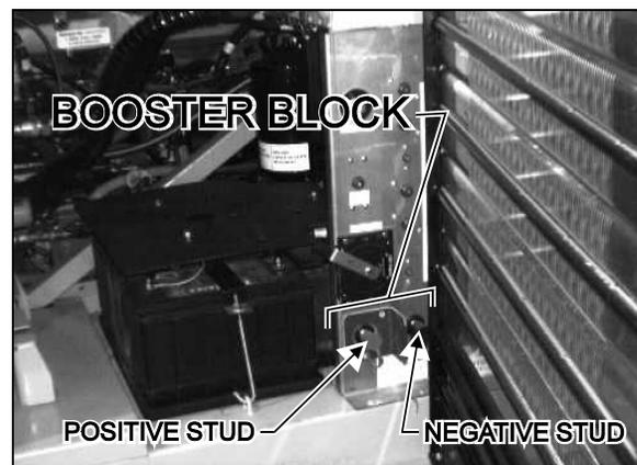
FIGURE 62: BOOSTER BLOCK (XL-45 CONVERTED VEHICLE) 06045
