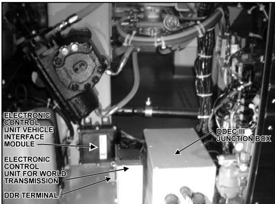
FIGURE 10: STEERING COMPARTMENT 06120
