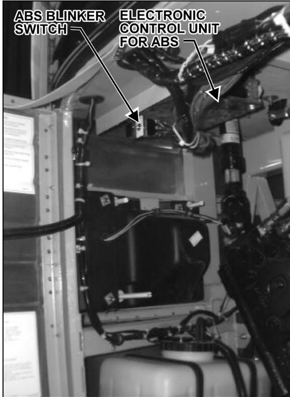
FIGURE 23: STEERING COMPARTMENT (LEFT WALL) 06119
