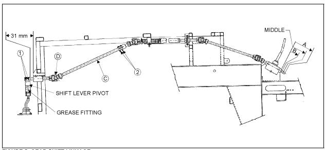
FIGURE 5: GEAR SHIFT LINKAGE
