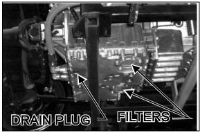
**FIGURE 4: PLUG AND FILTERS**
