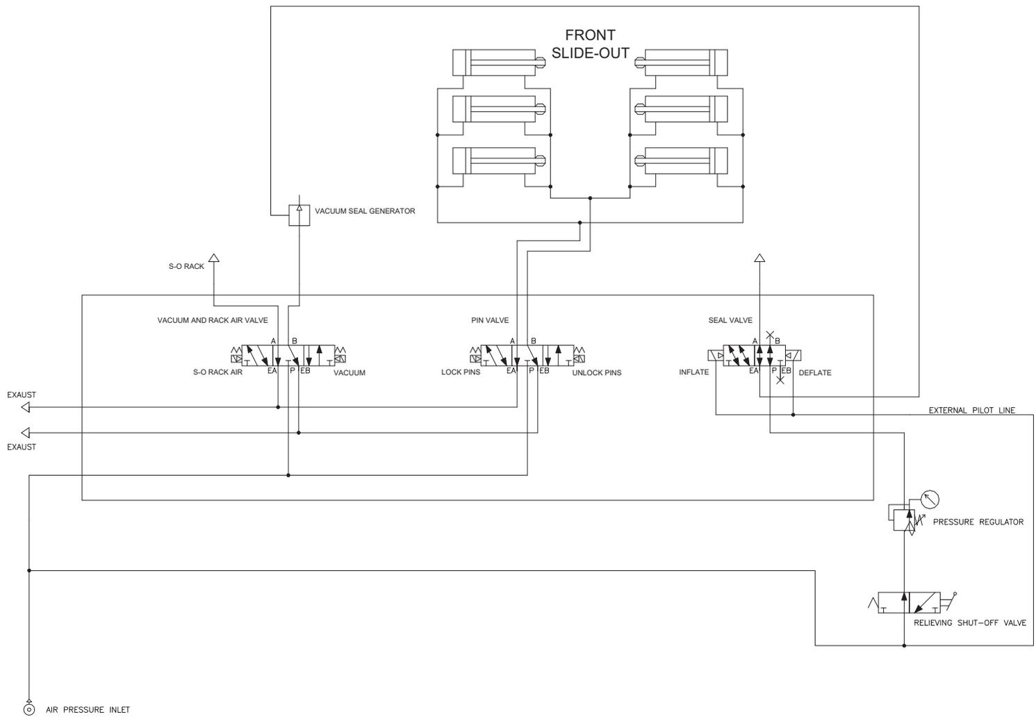
**XL2 SINGLE SLIDE-OUT PNEUMATIC SCHEMATIC DIAGRAM**
