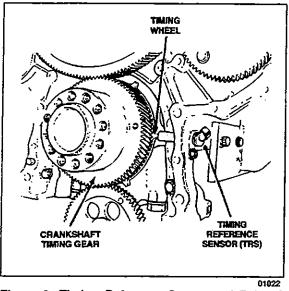
Figure 6: Timing Reference Sensor and Related Parts
