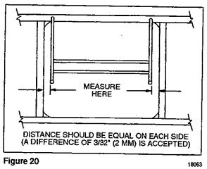
Install the baggage compartment door. Unscrew and remove both striker pins. Loosen bolts retaining door to pantograph and balance arm supports. With door closed, adjust height so the top of the door fits flush with the adjacent doors, then complete tightening the four bolts retaining door to each pantograph arm support. A gap of 1/8" (3 mm) between the top of the door and the stainless steel support is given as a guide. Refer to figure 21.
