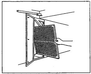
Figure 14: Main HVAC Unit Air Filter
