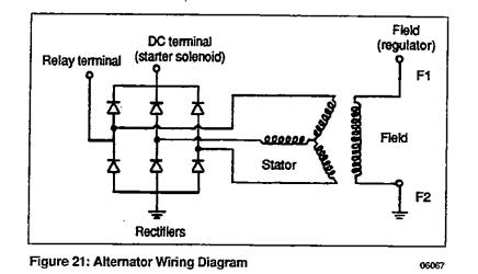
**Note:** The relay coils connected to the alternator "relay terminal" SHOULD NEVER BE PROVIDED WITH A SUPPRESSOR DIODE as the output current at this terminal is not rectified, thus rendering relay inoperative.
