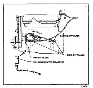
Figure 1: Location of Manual Shut-off Valves
