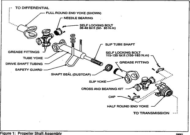
Figure 1: Propeller Shaft Assembly
