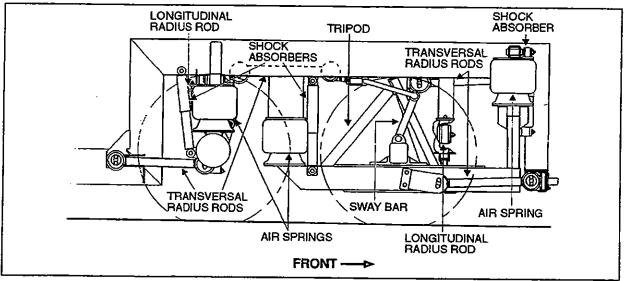
Figure 3: Rear Suspension Components
