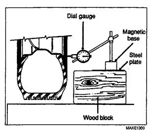
Figure 3: Suggested Dial Gauge Installation
