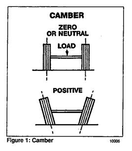
The camber angle is not adjustable. Camber variations may be caused by wear at the wheel bearings, steering knuckle pins, or by a bent knuckle or sagging axle center. Steering effort is affected by improper camber, and uneven tire wear will result. Excessive positive camber causes an irregular wear of tire at the outer shoulder, and excessive negative camber causes wear at the inner shoulder.
