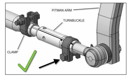
Note horizontal orientation of clamp bolt and bolt insertion direction. Prescribed torque for clamp bolt (arrow) is between 50 and 60 lbf-ft. Applies to both clamps. If replacement is required, order the following parts:
