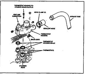
Figure 14: Thermostat and Related Parts 05034
