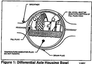
Figure 1: Differential Axle Housing Bowl
