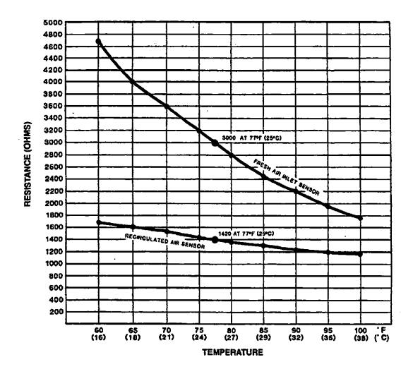
Table 2: Resistance Range According to Ambient Temperature Sensors
