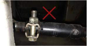
Clamp is bent. Replace clamp.
