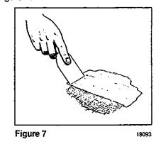
Smooth off surface with coarse sandpaper #100 to desired shape. Further smooth surface with fine sandpaper #120 until repaired surface matches surrounding area panelling. Prime and paint the area to match surrounding paintwork.
