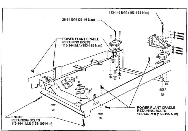
Figure 18: Power Plant Cradle Installation
