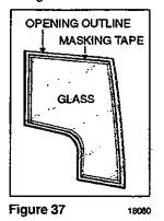
Clean all around the window opening and the window glass edge with isopropyl alcohol, enamel reducer or NAPA 6383 surface cleaner. Let dry 1 to 2 minutes.
