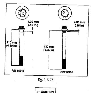
It is imperative that the correct Jacobs bolts be used for the engine brake housing being installed. Installation of incorrect bolts will result in engine and engine brake damage.
