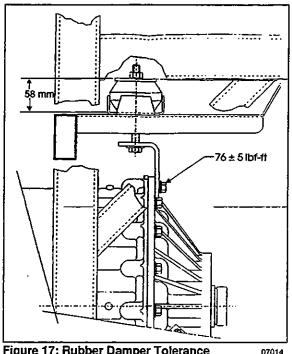
Figure 17: Rubber Damper Tolerance
