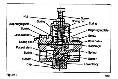
The belt tensioner pressure regulating valve controls pressure in the three belt tensioner cylinders as these latter are parallel mounted. It is located on the structure post at left of the oil reserve tank in engine compartment and is used to limit the air pressure in belt tensioners to  $50 \pm 2$  psi ( $345 \pm 15$  kPa).
