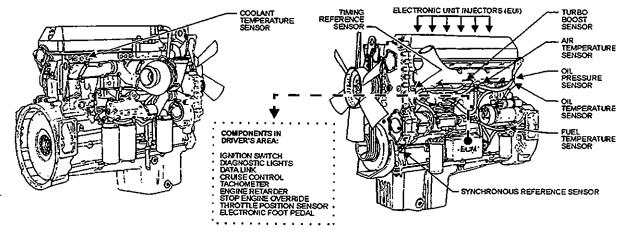
NOTE: COOLANT LEVEL SENSOR IS MOUNTED ON COOLANT SURGE TANK, LOCATED ON UPPER L.H. SIDE OF ENGINE COMPARTMENT.
