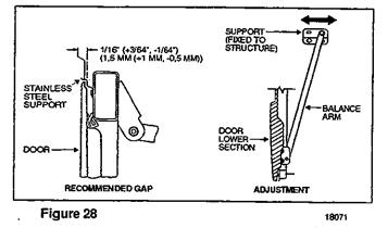
Once the adjustment procedure is achieved, ensure that all bolts are securely tightened.
