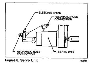
Remove the plastic tube on the bleeding valve. Make sure the bleeding valve is open. Force fluid (meeting DOT 3 specifications) through the bleeding valve opening. Tighten teflon flexible hose connector when fluid is free of air bubbles. Continue to force brake fluid until it enters master cylinder reservoir and flows free of air bubbles.
