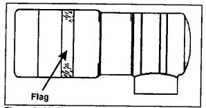
Figure 5: Air Cleaner Restriction Indicator OEH3B744
