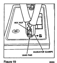
**Note:** If this connection cannot be made because of the alligator clamp design, the load value for testing must be reduced from 290 to 260 amperes.
