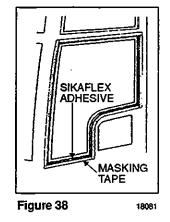
Apply a generous bead of Sikaflex-255 FC polyurethane adhesive (68-1092) on the sealing surface around the window opening from outside the vehicle.
