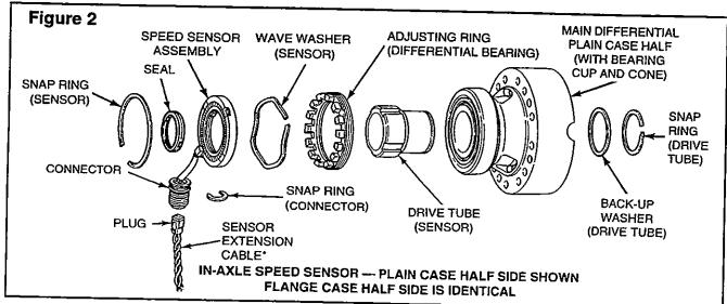
\* NOTE: Sensor Extension Cable — it is recommended that the two wires be twisted together at greater than 20 turns per meter.
