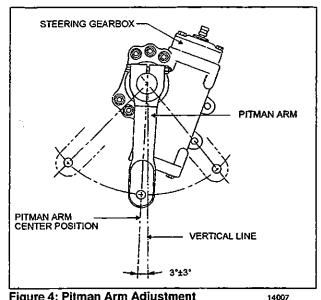
Figure 4: Pitman Arm Adjustment
