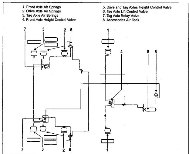
Figure 1: Pneumatic Suspension Components
