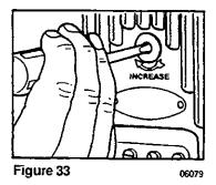
**Note:** If regulator voltage cannot be adjusted to the specified setting, remove the regulator and repair or replace it as necessary.
