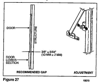
11. Recheck gap mentioned in step 9. If gap has changed, correct half the change by adjusting arm support fixed to structure. Loosen the bolt supporting balance arm on door lower section and close the door, gap adjustment will automatically result. Tighten the bolt from inside the compartment. Refer to figure 28.
