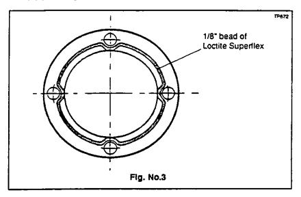
3.13 Fit hub cap along (3) within 5 minutes of applying sealant then secure with hub cap setscrews and washers (1 & 2) tightening setscrews to 85 - 103 lbs. tt. (115 - 140Nm.).
