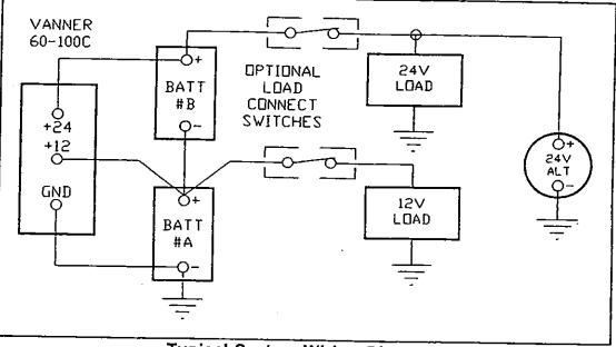
Typical System Wiring Diagram
