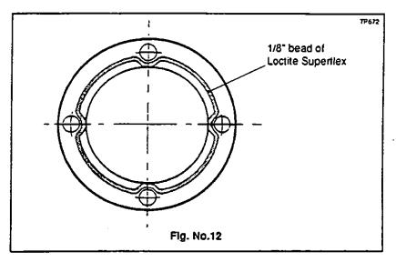
9.13 Fit hub cap along (3) within 5 minutes of applying sealant then secure with hub cap setscrews and washers (1 & 2) tightening setscrews to 85 - 103 lbs. ft. (115 - 140Nm.).
