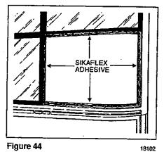
Apply Sikaflex-255 FC adhesive all around the rubber extrusion in the channel for the windshield opening flange. See figure 45.
