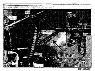
Figure 2: Fuel Tank Access Panel Location
