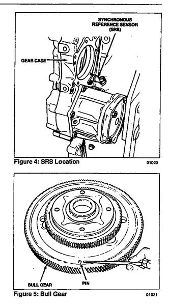
The bull gear pin passes by the SRS as the number one piston reaches 45° before Top-Dead-Center. This information is used by the ECM to determine engine speed.
