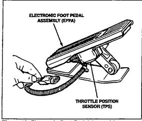
Figure 10: Electronic Foot Pedal Assembly 01026
