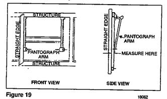
3. Measure distance between a pantograph arm end and the structure. Repeat procedure for the other arm. The distance on each side should be equal as the pantograph arm assembly must be centered in baggage compartment opening. If not, bend the appropriate pantograph arm end until desired measure is obtained. A difference of 3/32" (2 mm) between both sides is accepted. Refer to figure 20.
