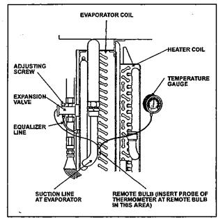
Figure 27: Superheat Adjustment Installation 22046
