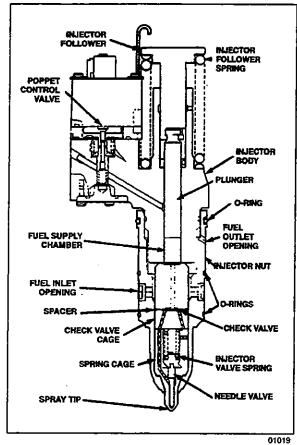
Figure 3: Electronic Unit Injector Cross-Section
