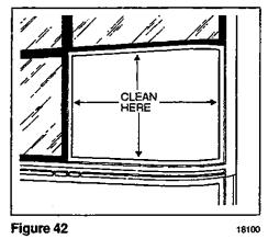
Clean the rubber extrusion with wiping towels soaked with isopropyl alcohol. Wipe with dry wiping towels and let dry 1 to 2 minutes.
