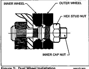
Figure 2: Dual Wheel Installation
