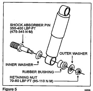
Remove the shock absorber assembly from pins. 3. Remove the two inner bushings from the shock absorber, and discard them.
