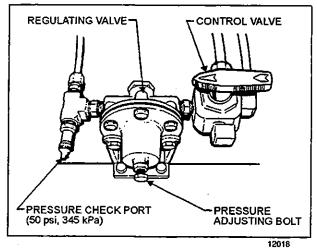
Figure 21: Belt Tensioning Pressure Control Valve
