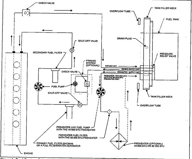
Figure1: Fuel System Schematic
