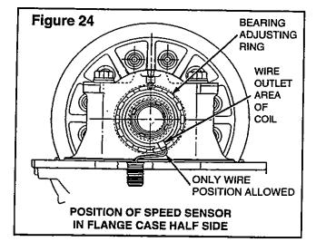
Place the speed sensor assembly over the bearing adjusting ring with the wires in the position shown in Figure 23 or 24. Tum the rotor in the sensor until the tabs align with the slots in the drive tube. Figure 25.
