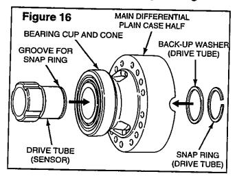
2. While holding the drive tube in position, place the back-up washer over the drive tube and against the inside of the differential case half. Install the snap ring into the groove in the drive tube using a screwdriver if necessary. **Figures 16 and 17.**
