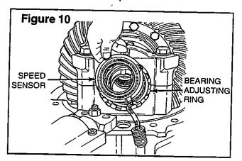
11. Remove the wave washer from inside the bore of the bearing adjusting ring. **Figure 11.**
