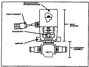
Figure 35: Main Hot Water Solenoid Valve 20054
