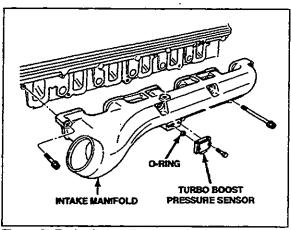
Figure 7: Turbo Boost Pressure Sensor 01023
