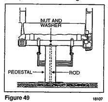
Note: Bottom end of rod is coated with Loctite and threaded in a steel block which slides in the floor track. Removal of rod is possible if loosened from block. Otherwise, slide rod and block assembly to the front end of track after removing all other interfering seats.
