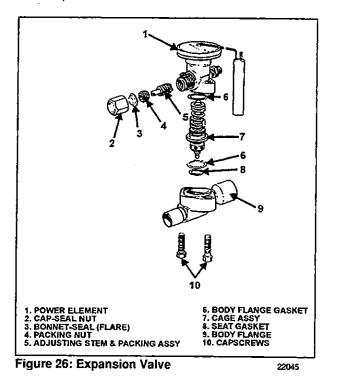
The remote bulb and power assembly is a closed system. The pressure within the remote bulb and power assembly corresponds to the saturation pressure of the refrigerant temperature leaving the evaporator and moves the valve pin in the opening direction.
