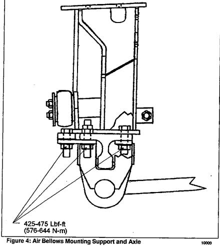
For more torque specifications, see "GKN Parts and Service Manual For Axles", Manual No. 1604, Issue A, Section B annexed to the end of this section, under heading "Tightening Torque Table for Type S82 Steer Axie".
