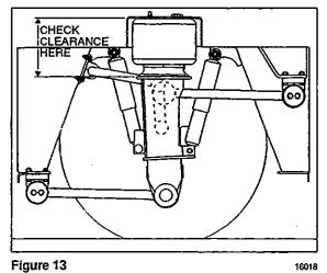
**Note:** The measure should be taken from under the upper air spring support on subframe to top of the lower air spring support on axle (refer to fig. 13 for more details). If adjustment is required, begin with the drive axle.
