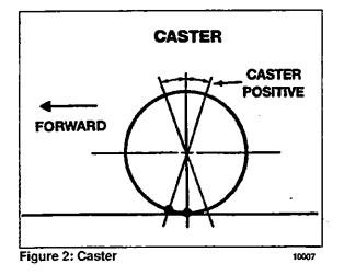
Excessive caster results in hard steering around corners. A shimmy may also develop when returning to the straight-ahead position (pulling out of curves).
