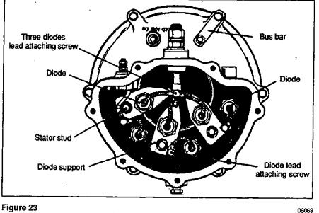
5. Disconnect all diode flexible leads; i.e. three from the output terminal stud and three from the diode supports. See figure 23 for more details.
