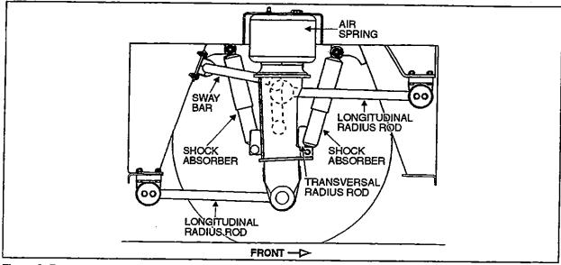
Figure 2: Front Suspension Components
