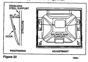
Fully open the door, loosen the two bolts retaining each gas cylinder support to structure, position door parallel with adjacent doors and complete tightening bolts. A measure of 6" ± 1/4", (150 mm ± 7 mm) between door panel lip (at level of upper edge of lower section) and the lateral panel is given as a guide. Refer to figure 23.
