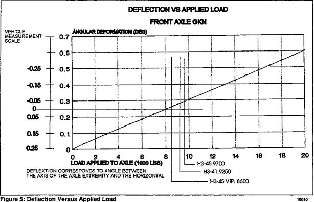
Figure 5: Deflection Versus Applied Load
