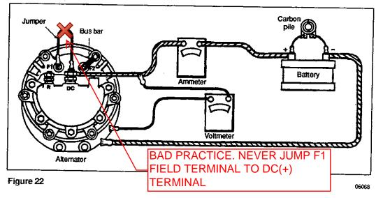
**Caution:** Do not feed the alternator field "F1" terminal for more than 10 seconds. High voltage could burn out the wires and components of charging system, and seriously damage the alternator.
