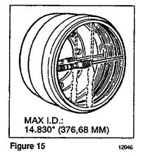
**Caution:** Prévost does not recommend the turning or reboring of the brake drums because it decreases the strength and heat capacity of the drum. However, if drums must be refaced, the new diameter MUST NOT exceed the maximum inside diameter marked on the drum.
