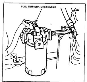
Figure 8: Engine Fuel Temperature Sensor 01024
