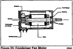
Figure 23: Condenser Fan Motor
