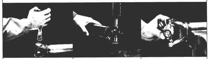
Remove snap ring from yoke. Turn joint over, tap bearing away from snap ring, then remove opposite snap ring.
