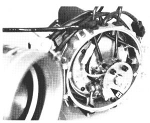
LOCATIONS OF THE PRE-HEAT THERMOSTAT FOR DBW 2020, DWB 300 AND DBW 350 MODELS (1)
