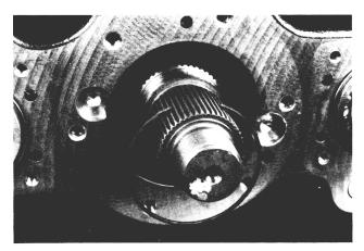
7. Cut the lockwire and slide the reverse gear rearward. install the first gear bore snap ring.
