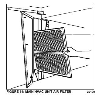
**Caution:** Do not use high pressure water jet to avoid damaging filter.
