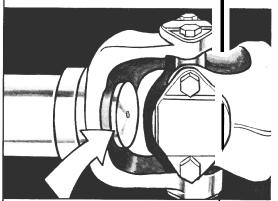
7. For an inboard and outboard slip yoke assembly design, check to be sure the plug is not loose or missing . . if it is, repair or replace it. Loose or missing plugs are commonly caused by not enough driveshaft slip capability.
