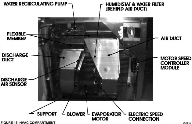
FIGURE 15: HVAC COMPARTMENT
