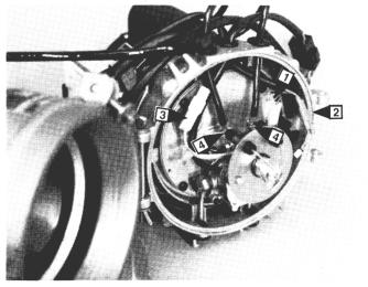
3. Remove the ring (1), holding disc (2), lift and carefully turn the disc (2), so that it releases from the ignition electrodes and the nozzle holder.
