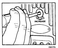
FIGURE 33: ADJUSTING REGULATOR VOLTAGE SETTING
