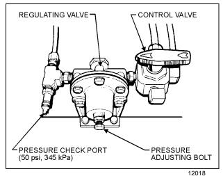
FIGURE 21: BELT TENSIONING PRESSURE CONTROL VALVE
