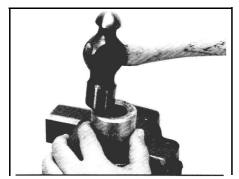
Install input shaft seal
