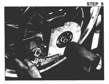
Lightly tap the aligning tool to make sure it is centered and seated into the pilot bearing.
