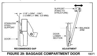
12. Once the adjustment procedure isachieved, ensure that all bolts are securely tightened.
