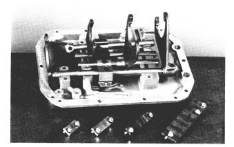
3. Loosen all fork and bracket setscrews, then remove the retainer straps.
