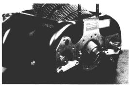
Countershaft alignment blocks for PS 140-7A and PS125-7B (Kent-Moore J 28720). Provide maximum clearance for mainshaft assembly installation. Allow countershafts to be rotated for timing purposes.
