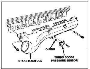
FIGURE 7: TURBO BOOST PRESSURE SENSOR 01023
