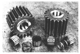
26. Check both idler gears and bearings for excessive wear.
