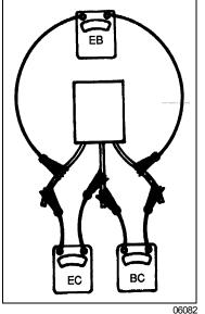
FIGURE 36: CHECKING TRANSISTORS TR2
