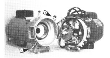
changer. Using a screw driver, pry loose all around a little at a time (1).
