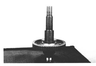
3. Place the internally and externally splined thrust washers on the shaft. The internally splined thrust washer should rest against the mainshaft snap ring.
