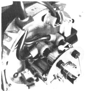
5. Disconnect the return (1) and suction (2) pipes from the fuel pump, Disconnect the delivery pipe (3) from the pump to the nozzle holder. Unscrew the four screws (4) on the back wall and take it out with the nozzle holder and the fuel pump. Remove both bolts (5) which secure the pump.
