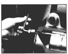
Turn adjusting screw assembly into housing 4.
