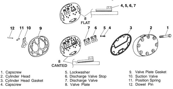
Figure 3-1. Cylinder Head & Valve Plate
