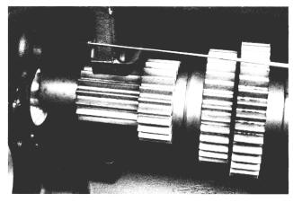
25. Because of this upper idler boss interference, it is easier to remove the right side countershaft first. Then remove the left side countershaft.
