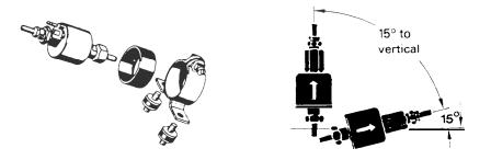
**NOTE:** The mounting angle of the fuel pump is critical, it is necessary to adhere to this angle to allow any air or vapor in the fuel lines to pass through the pump rather than cause a blockage and to provide accurate metering of the fuel.
