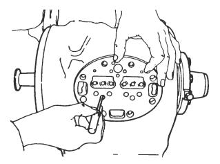
Figure 3-3. Checking Suction Valve
