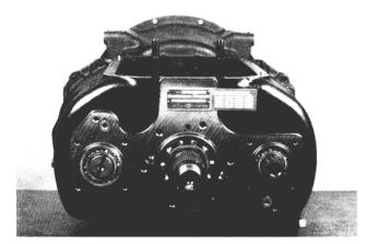
3. Remove the countershaft bearing retainers.
