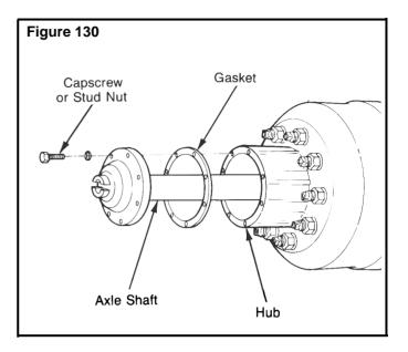
**15.** Install the nuts\* and washers on the studs\*. Tighten nuts\* to the correct torque value. See the torque chart on page 65.
