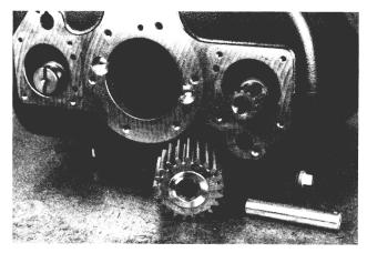
24. Remove the lower idler shaft and idler gear.
