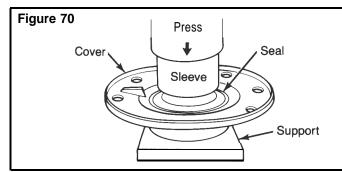
E. Press the seal into cover until seal is flat against the bottom of bore. Use a sleeve or seal driver of the correct size that fits against the metal retainer of seal. **Figure 70.**
