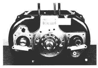
10. Slide the output bearing onto the shaft with a suitable driver. It is properly seated when the snap ring seats against the case.
