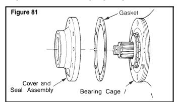
**5.** Align the oil slots in the cover\* and gasket\* with oil slot in the bearing cage.
