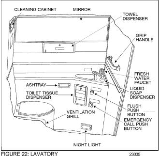
Locking the door from inside will illuminate the ceiling fluorescent light plus outside signs which are mounted on the outer wall of lavatory, over the windshield and an indicator light on the L.H. dashboard. A night-light is always illuminated when ignition switch is in the "ON" position.
