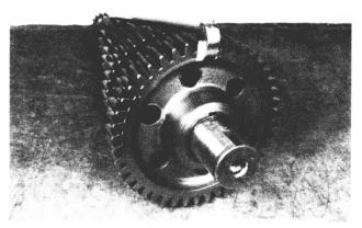
2. If you place a straight edge between these painted teeth, every gear on the countershaft will be in line. When you set the countershafts in time, these marks will be directly across from each other.
