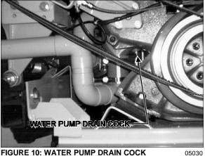
FIGURE 10: WATER PUMP DRAIN COCK
