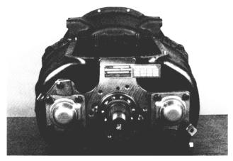
2. Remove the output bearing cap and gasket,
