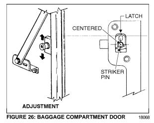
**Note:** Before proceeding with the following step, mark the position of striker pins on structure to avoid upsetting the vertical adjustment of the pin.
