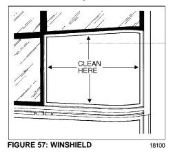
2. Clean the rubber extrusion with wiping towels soaked with isopropyl alcohol. Wipe with dry wiping towels and let dry 1 to 2 minutes.
