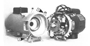
2. Unscrew the pre-heat thermostat (1) and disconnect wires.
