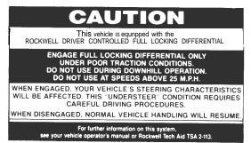
Check to see that the "Driver Caution" label is installed in the vehicle cab. The caution label must be put in a location that is easily visible to the driver. A recommended location is on the instrument panel, next to the differential lock switch and lock indicator light. Driver Caution labels (Tp-861 01) are available from Rockwell International, Troy, Michigan. **Figure 146.**
