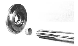
1. The input gear, shaft, and bearing are separate components secured with 2 snap rings.
