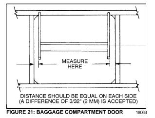
4. Install the baggage compartment door. Unscrew and remove both striker pins. Loosen bolts retaining door to pantograph and balance arm supports. With door closed, adjust height so the top of the door fits flush with the adjacent doors, then complete tightening the four bolts retaining door to each pantograph arm support. A gap of 1/8" (3 mm) between the top of the door and the stainless steel support is given as a guide. Refer to figure 22.
