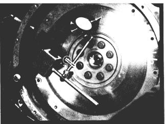
Begin by wiping all surfaces before gauging. Secure the dial indicator to the engine flywheel housing with the gauge finger on the face of the flywheel near the outer edge.
