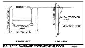
Measure distance between a pantograph arm end and the structure. Repeat procedure for the other arm. The distance on each side should be equal as the pantograph arm assembly must be centered in baggage compartment opening. If not, bend the appropriate pantograph arm end until desired measure is obtained. A difference of 3/32" (2 mm) between both sides is accepted. Refer to figure 21.
