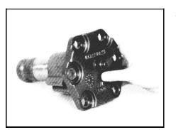
Assemble vent plug 23. Press the new vent plug (49) into the hole provided in the side cover until the plug is bottomed.
