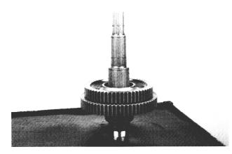
4. Place second gear on the shaft, Install the externally and internally splined thrust washers into the gear. Secure the assembly with a snap ring.
