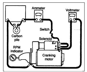
FIGURE 38: STARTING MOTOR TEST CONNECTIONS
