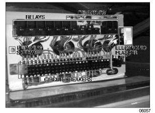
FIGURE 10: FRONT ELECTRICAL COMPARTMENT - ON JUNCTION BOX
