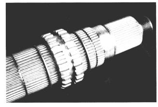
2. Lube all parts prior to reassembly. Install the first-reverse snap ring in the second groove from the bottom of the shaft. Slide the first-reverse collar into place and secure it with a snap ring.
