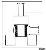
FIGURE 8: RADIUS ROD BUSHING INSTALLATION
