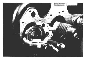
20. Install a puller for bearing removal.
