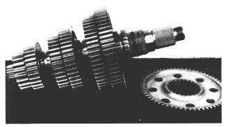
1. Begin disassembly of the mainshaft by cutting the lockwire and removing reverse gear.
