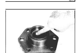
Lubricate side cover bushing/ bearing
