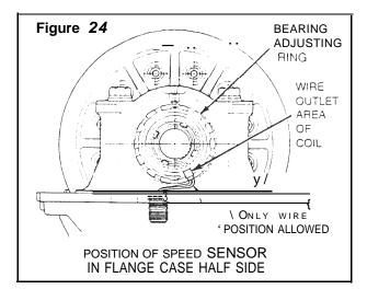
9. Place the speed sensor assembly over the bearing adjusting ring with the wires in the position shown in Figure 23 or 24. Turn the rotor in the sensor until the tabs align with the slots in the drive tube. Figure 25.
