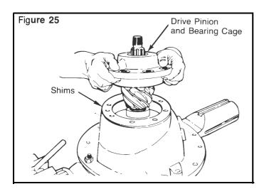
8. Remove the drive pinion, bearing cage and shims from the carrier. If the bearing cage is tight in the carrier, use the following procedures to loosen the cage. Figure 25.
