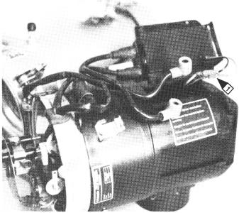
4. Press the connectors for the electric cables (1 upper picture) together.
