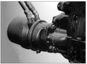
FIGURE 20: TAG AXLE BRAKE AIR CHAMBER 12050
