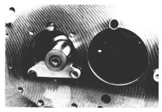
3. Align the countershaft timing marks toward the center of the case.
