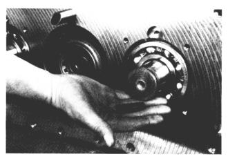
11. Continue by removing the countershaft driver gear countershaft keys.
