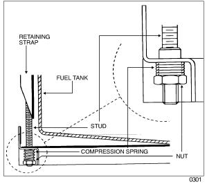
FIGURE 7: NUTS FOR FUEL TANK RETAINING STRAP
