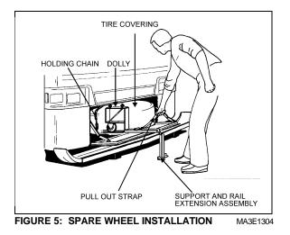
**Note:** Reinstall support and rail extension assembly and fix tire with loading chain before moving vehicle.
