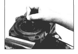
Assemble other oring and seal ring 16. Lightly oil and assemble new o-ring (1 1) and new seal ring (10) into the large diameter seal ring groove in valve housing, bending and working them in and smoothing them out as necessary.
