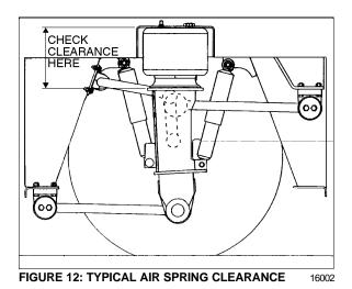
**Note:** The measure should be taken from under the upper air spring support on subframe to top of the lower air spring support on axle (refer to fig. 12 for more details). If adjustment is required, begin with the drive axle.
