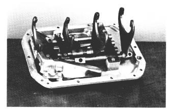
1. Disassembly of the cover begins by placing the cover on a bench with the forks up and in the neutral position.
