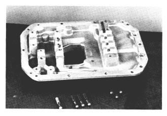
4. All forks lift easily from the cover, Remove the interlocks, poppets and springs. *The first-reverse spring has a different tension than the others, so don 't mix them up.*
