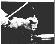
Using a soft drift, tap the outside of the bearing assembly to loosen snap ring. Tap bearing only hard enough to break assembly away from snap ring.
