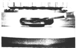
6. When snap ring grooves on the input shaft bearing and bearing retainer are in proper alignment, discontinue pressing and seat the snap ring in place. Inspect the assembly to assure the snap ring is properly seated and secured.
