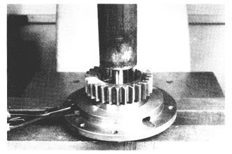
5. Expand the snap ring through the provided slot, while pressing the input shaft assembly into the bearing retainer. CAUTION should be used during this procedure. (This procedure is the same for all 7-speed, 2-piece input gears.
