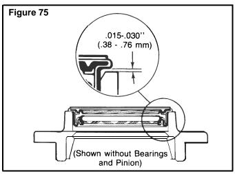
Check the gap with a feeler gauge at several points around the seal. The gap must be within .015 to .030 inch (.38 to .76 mm). The difference between the largest and smallest gap measurement MUST NOT exceed .010 inch.
