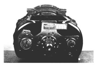
3. Remove the countershaft bearing retainers.
