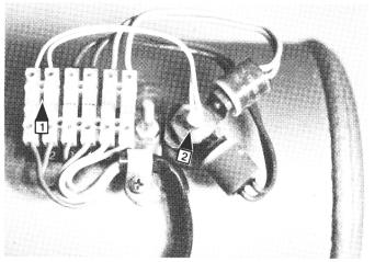
NOTE! The protection cap must be installed, otherwise the thermostats will not function properly.
