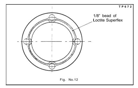
9.13 Fit hub cap along (3) within 5 minutes of applying sealant then secure with hub cap setscrews and washers (1 & 2) tightening setscrews to 85-103 lbs. ft. (115 - 140 Nm.).
