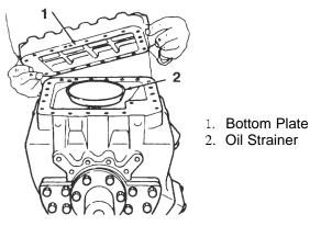
Figure 3-10. Bottom Plate Removal
