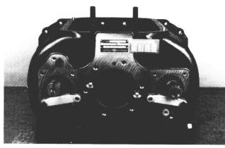
1. Reassembly of the unit begins by placing the lower reverse idler gear into the case. Then install the left side countershaft and the right side countershaft. Use of alignment blocks is recommended.
