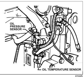
FIGURE 9: ENGINE OIL PRESSURE AND OIL TEMPERATURE SENSOR
