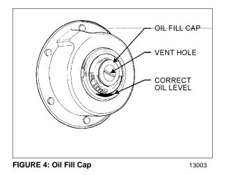
The oil level on the tag axle wheel bearings must be maintained to the level mark in the cap. The level is determined by a line, indicated by arrows, that is incorporated to the plastic lens and passes underneath the words "OIL LEVEL" (Fig. 4). To check oil level after vehicle has been driven, wait at least 15 minutes to ensure that oil has settled.
