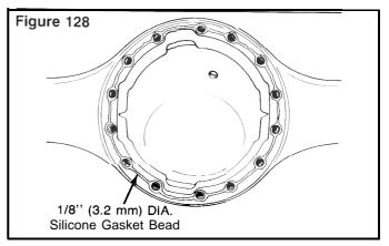
**6.** Install the carrier into the axle housing. Use a hydraulic roller jack or a lifting tool.
