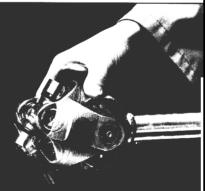
10. Check for proper assembly. Flex the CV joint beyond center. It should snap "over center" in both directions when all needle rollers and components are correctly assembled.
