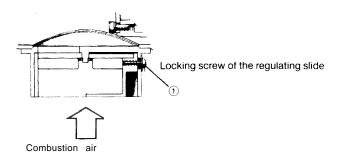
**Description:** The regulation of the combustion air at the intake socket serves to relate exactly the combustion air quantity to the fuel quantity atomized by the high-pressure atomizer nozzle.
