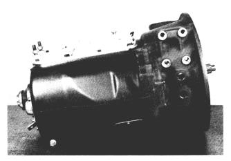
24. Bench shift the transmission to make sure everything is working properly. Then install the shifter housing and secure it with capscrews. Torque to 34-41 ft. lbs.
