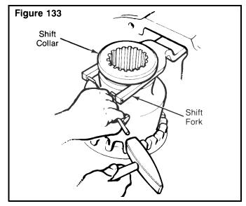
2. If required, remove the differential lock shift unit.
