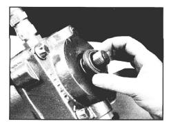
**Remove input shaft** 9. **seal**
