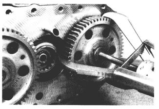
10. Remove the countershaft drive gears with the aid of a large puller.
