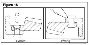
C. Press the rivets through holes in the ring gear and flange case half. Press from the drilled rivet head.
