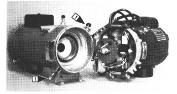
Detach the electric cables (1) for the flame control and connect to an ohm-meter. Calibrate the ohm-meter and check the resistance by placing your thumb over and then removing it from the "window" (2). If the flame control is operating properly, the instrument should clearly register resistance.
