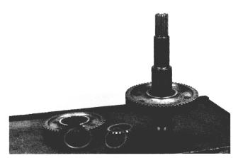
6. Remove the snap ring and second-third shift collar. Remove the next snap ring and lift second gear off the shaft. The gear contains two washers and a snap ring.
