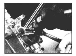
Reconnect column 15, Reconnect the steering column to the input shaft
