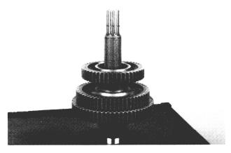
6. Place an internally splined washer and externally splined washer on the shaft. Install third gear.
