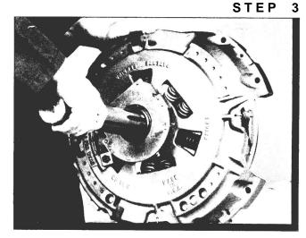
Insert the aligning tool through the release bearing sleeve in the new clutch.
