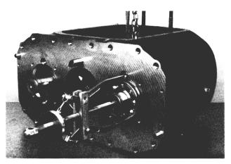
18. Use a puller to remove the countershaft front bearings.
