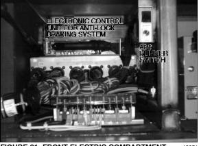
FIGURE 21: FRONT ELECTRIC COMPARTMENT 12051
