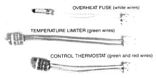
**Description:** The overheat fuse protects the heater against too high and inadmissible temperatures. The overheat fuse contains a fusible link reacting when the admissible temperature is exceeded (138° C [280° F]), and switches the heater off with a purge cycle.
