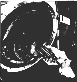
Install a spline aligning tool through the release bearing and the driven discs, into the pilot bearing. You can use an old transmission input shaft for this purpose.
