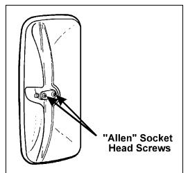
FIGURE 43: MIRRORS ADJUSTMENT SCREWS OEH3B120
