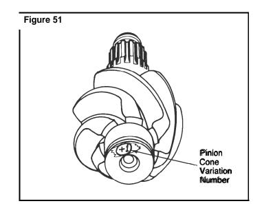
B. Location on Gear Set: End of pinion gear head or outer diameter of ring gear.
