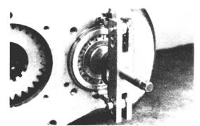
Countershaft front bearing puller (Snap-on-CJ 80).
