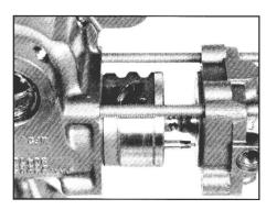
Assemble ball return guide halves 10. Compare the new guides with the guides removed from the gear, use the ones that look the same Left hand guides are copper plated, right hand guides are unplated, Assemble the new ball return guide halves (28) into the rack piston until seated, rotate the input shaft slightly if necessary.
