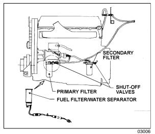
FIGURE 2: LOCATION OF MANUAL SHUT-OFF VALVES
