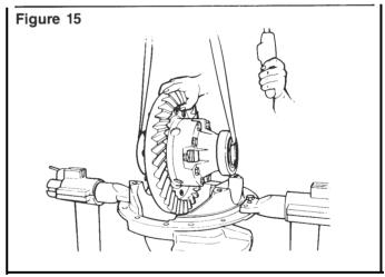
9. Remove the thrust block\* from inside the carrier.
