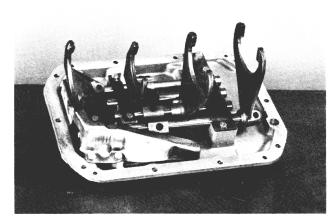
4. Next install the oil trough. Torque the bolts to 34-41 ft. Ibs. Check the cover for correct functioning by shifting one fork into gear. If all interlocks were installed correctly, none of the other forks will shift into gear.
