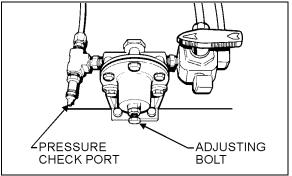
FIGURE 6: AIR PRESSURE REGULATING VALVE 12036
