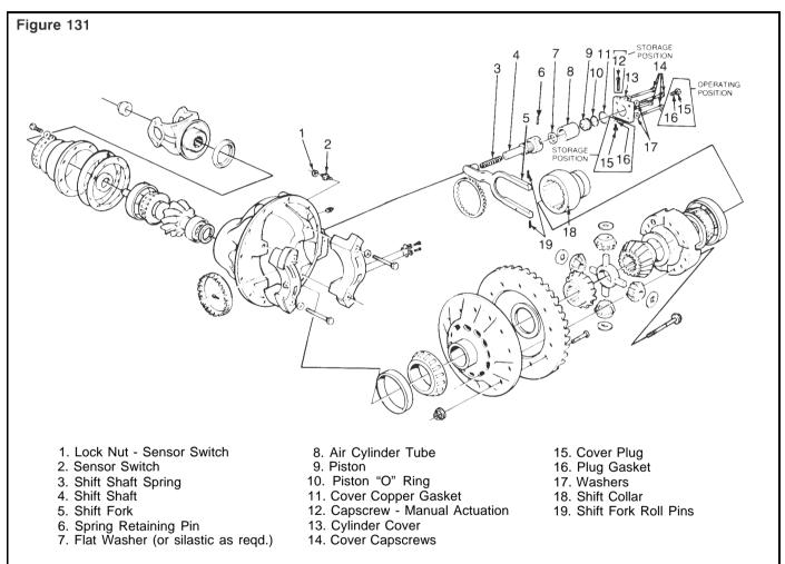
Some Rockwell drive axle models have a driver controlled main differential lock. This differential lock is operated by a carrier mounted, air actuated shift unit. When activated, the shift unit moves a sliding collar which is installed on the splines of the axle shaft. When engaged, the collar locks the axle shaft to a second set of splines on the differential case. **Figure** *131.*
