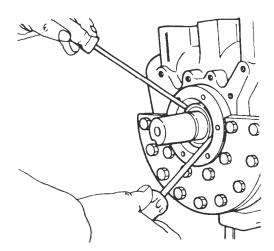
Figure 3-9. Shaft Seal Removal
