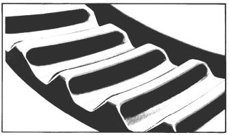
Figure 118B Good Pattern in Operation Generoid Gears
