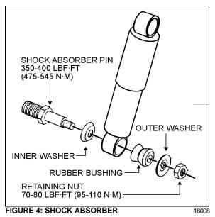
2. Remove the shock absorber assembly from pins.
