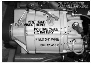
FIGURE 27: ALTERNATOR (HOSES AND WIRES) 06073
