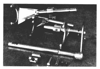
5. Next, disassemble the forks and brackets. Check all parts for wear or damage. Replace them if necessary.
