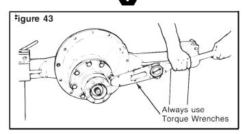
8. DO NOT repair rear axle housings by bending or straightening.
