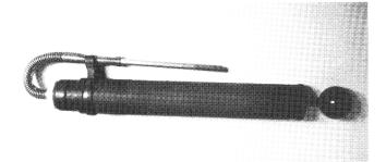
For checking Smoke Number use BRIGON smoke tester.
