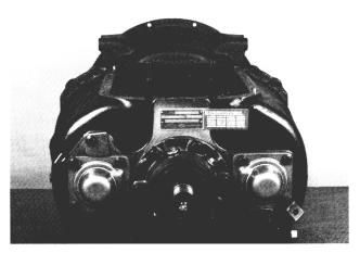
23. Place the countershaft bearing caps on the case and secure them with capscrews. Torque to 34-41 ft. lbs.
