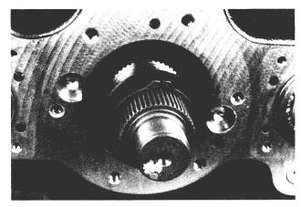
9. Install the internally splined thrust washer and secure it with the mainshaft snap ring.
