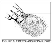
Cover the area with a layer of resin putty and allow to dry for approximately 15 to 20 minutes. See figure 7.
