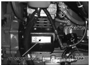
FIGURE 9: AIR COMPRESSOR AND GOVERNOR 12068
