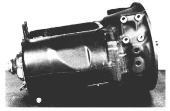
1. Remove the capscrews and shifter housing. If the shifter housing is a forward control, shift the transmission into sixth gear.
