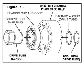
2. While holding the drive tube in position, place the back-up washer over the drive tube and against the inside of the differential case half. Install the snap ring into the groove in the drive tube using a screwdriver if necessary. **Figures 16 and 17.**
