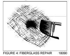
**Note:** Remove all air between surfaces being joined. Allow area to harden and sand surface to remove any wax.
