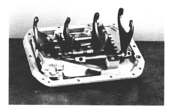
1. Disassembly of the cover begins by placing the cover on a bench with the forks up and in the neutral position.
