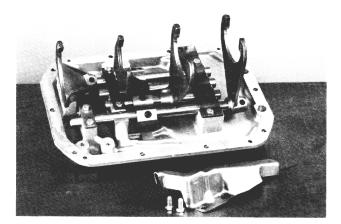
2. Remove the trough. It will make disassembling the rest of the cover easier.
