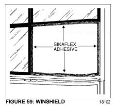
7. Apply Sikaflex-255 FC adhesive all around the rubber extrusion in the channel for the windshield opening flange. See figure 60.
