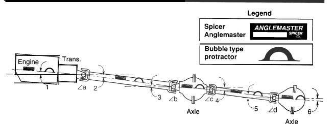
The most convenient way to determine U-joint angles in the side view is through use of a Spicer Anglemaster<sup>™</sup> or a bubble type protractor. Procedure is as follows:
