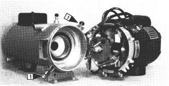
2. Disconnect the ignition cables (1) from the electrodes and loosen the retaining clamp bolt (2).
