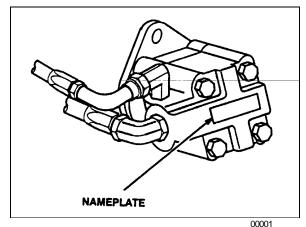
FIGURE 5: POWER STEERING PUMP NAMEPLATE
