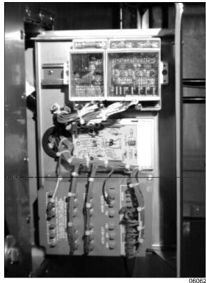
FIGURE 5: A/C HEATING JUNCTION BOX SLIDING DRAWER In the Heat Mode
