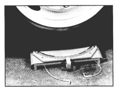
Set axle stops, warm-up system 1. Set the axle stops to vehicle manufacturer's wheelcut or clearance specifications.
