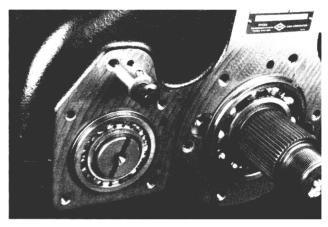
4. Insert a capscrew into the upper reverse idler shaft for removal. Don't lose the lockbail in the shaft.
