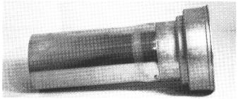
**Description:** Within the burner tube of the combustion chamber the fuel-air mixture, prepared by the high-pressure nozzle, is burned.
