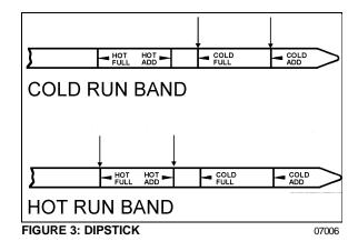
**Note:** The cold check is more appropriate for verifying the oil level after the first fill-up. In case of conflict, the hot check has priority over the cold check; the automatic system of verification via the shift selector has priority over the hot check.
