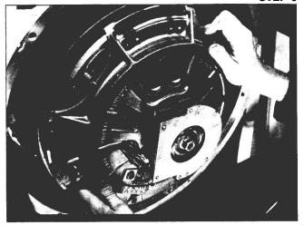
Position the clutch cover over the guide studs installed at the top of the flywheel. Make sure that the Kwik-Adjust mechanism will be aligned with the opening in the bell housing of the transmission.
