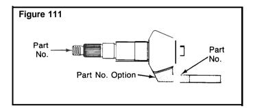
Examples of part numbers for conventional gear sets, 36786 for the ring gear. 36787 for the drive pinion.
