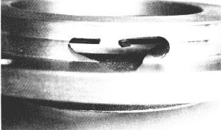
3. When reassembling, first install the snap ring into the input bearing cap.
