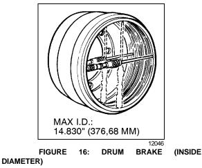
**Caution:** Prévost does not recommend the turning or reboring of the brake drums because it decreases the strength and heat capacity of the drum. However, if drums must be refaced, the new diameter MUST NOT exceed the maximum inside diameter marked on the drum.
