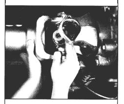
5. Free the trunnion from the end yoke by tilting the trunnion and collapsing the driveshaft.
