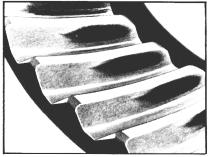
Figure 115A Good Hand Rolled Pattern
