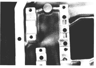
6. Check the poppet and detent holes for burrs or damage.
