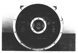
18. Apply a light coat of Loctite 51 5 to the clutch housing. Attach the housing to the case and secure it with capscrews. Torque them to 150-180 ft. lbs.
