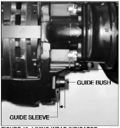
FIGURE 13: LINING WEAR INDICATOR 12043
