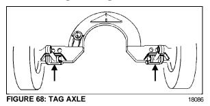
*Warning:* The jacking points on the tag axle must be used for raising the tag axle only.
