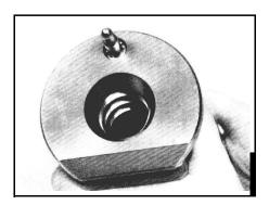
Inspect rack piston 2. ball track grooves Inspect the rack piston (19) ball track grooves for brinelling or spalling. If either condition exists, replace the input shaft, valve/worm assembly, valve housing, rack piston subassembly and balls.
