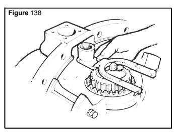
**5.** Hold the shift fork in position and install the shift shaft spring into the shift shaft opening in the carrier, through the shift fork bore and into the bore for the shift shaft spring. **Figure 139.**
