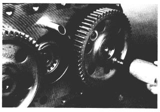
16. Using the alternating method, draw the gear onto the shaft, until it is seated behind the snap ring groove. Repeat this method for the other gear.
