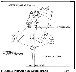
FIGURE 4: PITMAN ARM ADJUSTMENT
