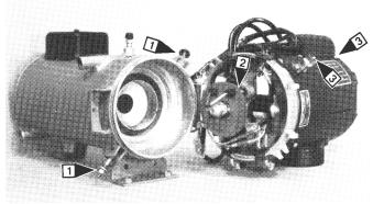
3. Lift up the ignition unit sufficiently in order to disconnect the connectors for the electric cables (I).
