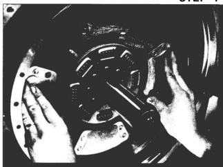
Re-insert the aligning tool through the hub of the front driven disc and into the pilot bearing.
