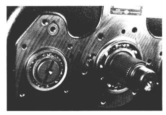
21. Install the upper reverse idler shaft. It is difficult to align the gear with the case hole unless the input shaft is in the unit. It is also necessary to lift up on the mainshaft reverse gear to obtain proper alignment.
