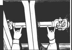
NOTE: Before removal of the driveshaft set the brakes, block the wheels, and mark the slip yoke assembly and tube shaft with a marking stick or paint to assure proper alignment when reassembled, This is known as keeping the driveshaft yokes "In Phase."
