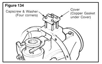
C. Remove the shift unit-cylinder and piston. Remove the O-ring from the piston.
