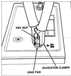
FIGURE 19: ALLIGATOR CLAMPS AND BATTERY 06065
