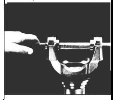
If, after proper cleaning, the alignment gauge still does not pass through both crossholes, the yoke lugs are distorted and the yoke should be replaced.
