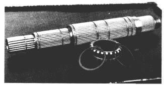
8. Remove the two snap rings and the first-reverse shift collar from the shaft.
