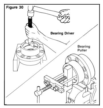
7. If the pinion bearings need to be replaced, remove the inner bearing cone from the drive pinion with a press or bearing puller. The puller MUST fit under the inner race of the cone to remove the cone correctly without damage. **Figure 31.**
