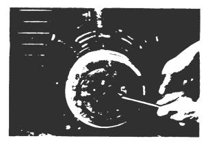
17. Insert a .020 feeler gauge between the outside edge of the clutch bearing mounting hub and the inside edge of the armature mounting hub, as shown. The clearance should be .020 or greater,
