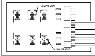
FIGURE 18: HVAC LOGIC PANEL
