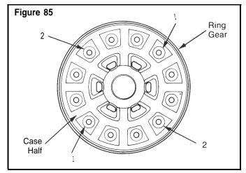
B. Press the rivets\* into position from the ring gear side of the assembly. Use a riveter machine and apply the correct amount of pressure. See Chart 3 for rivet pressures.
