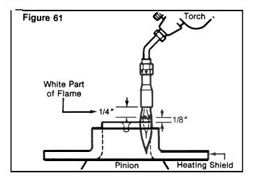
D. Remove the flame and the heat shield from the pinion. Let the pinion air cool for 10 minutes. Use a razor blade to remove the temperature indicating liquid.
