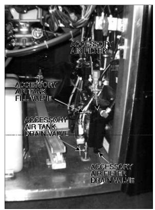
FIGURE 3: FRONT SERVICE COMPARTMENT 12034
