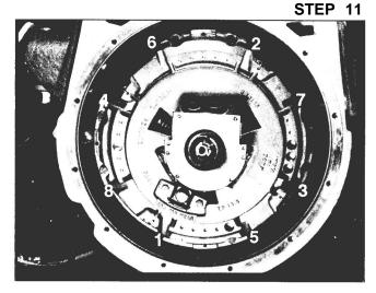
Tighten the bolts in the criss-cross sequence shown to pull the clutch into its proper position in the flywheel pilot. You must start with the lower left-hand bolt.
