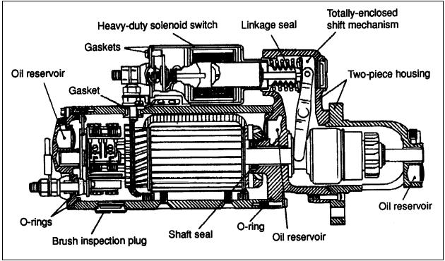
FIGURE 37: TYPICAL CRANKING MOTOR CROSS SECTION
