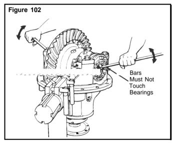
B. Use two pry bars between the differential case or ring gear and the carrier at locations other than described in step A. The prv bars MUST NOT touch the differential bearings. **Figure 103.**
