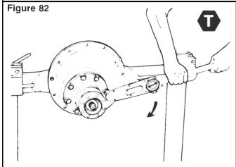
**7.** Install the input yoke or flange, nut and washer\* on the drive pinion. The yoke or flange MUST be against the outer bearing.
