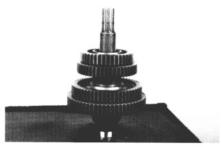
7. Place the externally splined thrust washer, snap ring and internally splined thrust washer in the gear. Slide fourth gear onto the shaft. Secure it with a snap ring.
