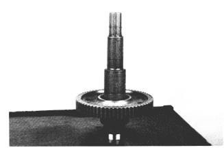
3. Place the internally and externally splined thrust washers on the shaft. The internally splined thrust washer should rest against the mainshaft snap ring.
