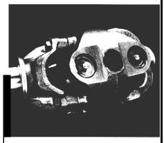
The double-cardan constant velocity (CV) type u-joint is a special design to accommodate necessary installation angles not compatible with single-cardan ujoints. The CV joint also requires special attention. Neglect is its main enemy.
