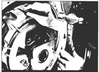
Using a 1/4" diameter flat nose drift, *lightly* tap each of the four positive separator pins toward the flywheel. After tapping, the pins should be flush against the flywheel.
