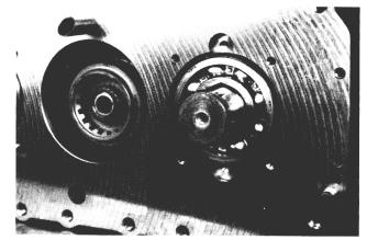
14. Next install the countershaft drive gear keys.
