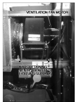
FIGURE 23: VENTILATION FAN MOTOR 23036
