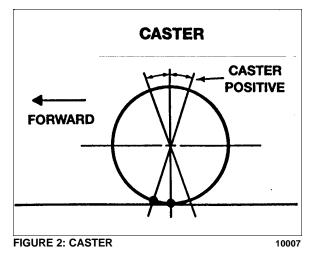
Excessive caster results in hard steering around corners. A shimmy may also develop
