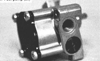
**Description:** The fuel pump (single-staged toothed pump) delivers the fuel from the tank to the heater and brings it to a pressure of 8-0.5 bar (116-7 psi) for DBW 2010,  $10\pm0.5$  bar (145 $\pm7$  psi) for DBW 2020, 300, 350.
