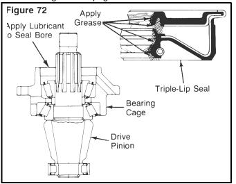
B. Apply the same lubricant used in the axle housing to the outer surface of the seal and the seal bore in the bearing cage. **Figure 72.**
