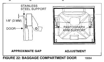
5. Slightly open the door, position it to obtain a gap of 4" (100 mm) between structure and door panel upper lip, maintain door in this position while an assistant completes tightening the two bolts retaining door to each balance arm support. Refer to figure 23.
