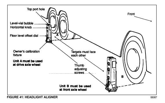
Note: Check that the three indicators on each module are set to zero.
