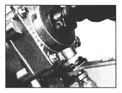
Reconnect return line 16. Reconnect the return line to the steering gear return port.
