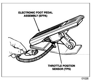
FIGURE 10: ELECTRONIC FOOT PEDAL ASSEMBLY
