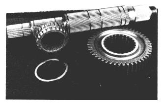
12. Clean all parts and inspect them for wear or damage. Replace them if necessary. Remember: if a gear is damaged and is going to be replaced, also replace its mating countershaft gears.
