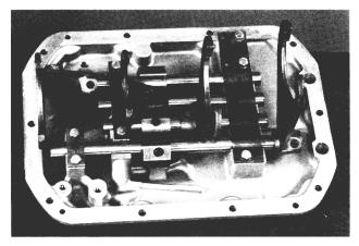
3. Place the fork assemblies into the case. Secure them with the retainer straps. Torque the strap bolts to 34-41 ft. lbs. Move each rod in the cover to confirm that it is moving freely.
