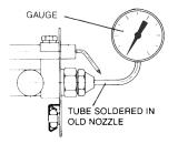
Instead of the fuel nozzle, a used nozzle is screwed in, into which a pipe with connected manometer (indication range  $0 \div 12$  bar (0 ÷180 psi) is soldered (see item 6.19). PART NUMBER 600.190
