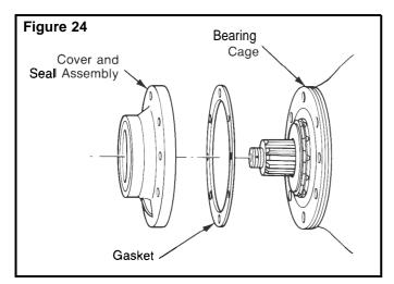
7. If the pinion seal is damaged, remove the seal from the cover\*. Use a press and sleeve or seal driver. If a press is not available, use a screwdriver or small pry bar for removal. Discard the pinion seal.
