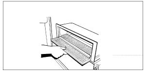
FIGURE 13: DRIVER'S HVAC UNIT AIR FILTER MAXE2209
