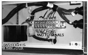
FIGURE 13: IN ALARM JUNCTION BOX
