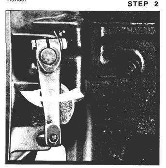
Before pulling the transmission free, disconnect the external clutch linkage and rotate the release yoke so it will clear the release bearing when it is removed. Carefully pull the transmission back to remove the splined shaft from the driven discs and the clutch.
