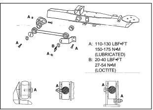
FIGURE 9: RADIUS ROD INSTALLATION 16013
