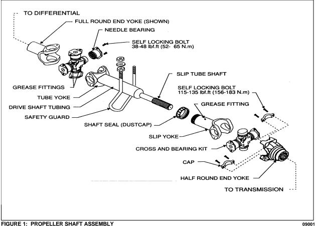
FIGURE 1: PROPELLER SHAFT ASSEMBLY
