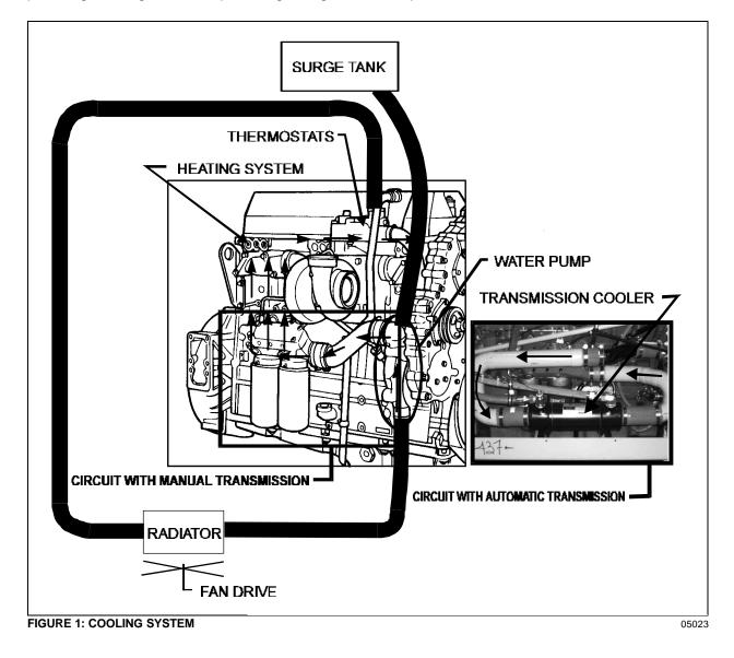
The engine coolant is drawn from the lower portion of the radiator by the water pump and is forced through the oil cooler and into the cylinder block. For vehicles with automatic transmissions the coolant circulates in the transmission cooler before going through the oil cooler and the cylinder block.
