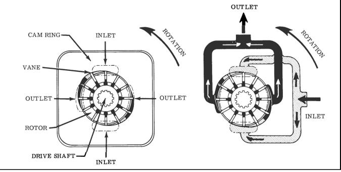
past the large diameter or dwell section of the cam ring. As the outlet section is approached, the cam ring diameter decreases and the fluid is forced out into the system. System pressure is fed under the vanes, assuring their sealing contact against the cam ring during normal operation.
