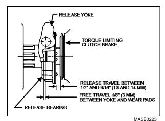
FIGURE 2: RELEASE TRAVEL AND FREE PLAY TRAVEL ADJUSTMENT
