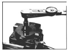
Adjust to required input torque
