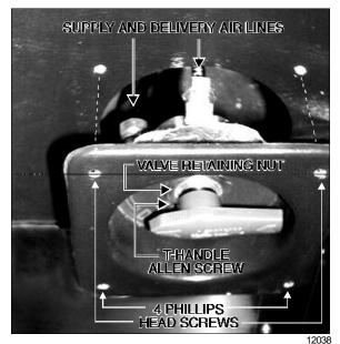
FIGURE 8: R.H. SIDE OF THE DRIVER'S HVAC UNIT ACCESS PANEL
