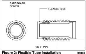
Figure 2: Flexible Tube Installation
