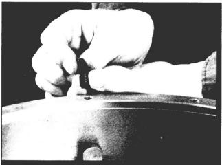
Mark the flywheel to crankshaft positon with a piece of soapstone or chalk and remove the crankshaft bolts. Remove the flywheel and set it on a flat work surface.
