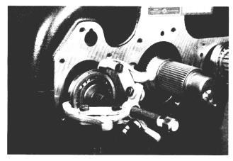
20. Install a puller for bearing removal.
