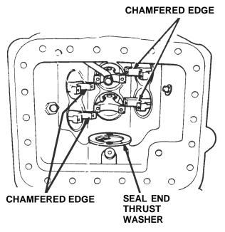
Figure 3-16. Installing Piston Rod Assemblies and Seal End Thrust Washer
