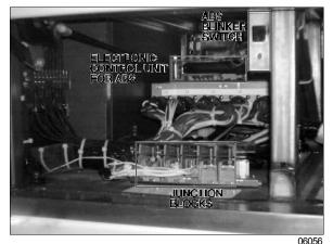
FIGURE 9: FRONT ELECTRICAL COMPARTMENT - LEFT SECTION
