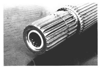
1, Install the pocket bearing to a depth of ,070".
