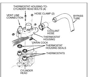
FIGURE 14: THERMOSTAT AND RELATED PARTS 05034
