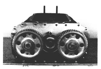
17. Once the gears are seated, install the snap rings and the sixth-seventh clutch collar.
