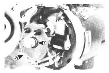
4. Loosen the retaining clamp bolt (1) and dismount ignition electrodes.
