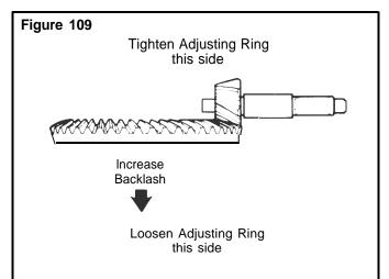
Loosen one bearing adjusting ring one notch then tighten the opposite ring the same amount. See Figures 109 and 110.
