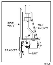
FIGURE 63: PASSENGER SEAT FRAME HOLDING
