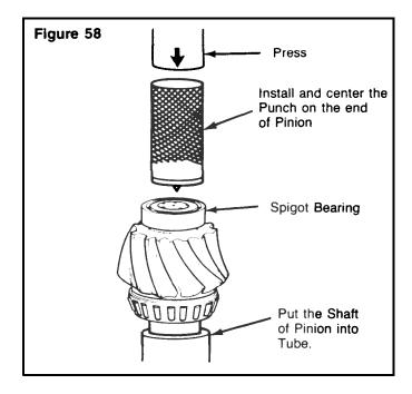
C. Put the punch of the peen tool over the end of the pinion and spigot bearing. Apply the required amount of force on the punch. **Figure 58.**
