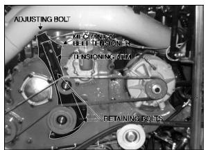
FIGURE 29: ALTERNATOR DRIVE BELT
