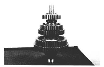
9. Place the externally splined thrust washer, snap ring and internally splined thrust washer in the gear. Slide fifth gear onto the shaft. Secure it with a snap ring.
