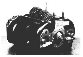
22. Lift the mainshaft assembly out of the case.
