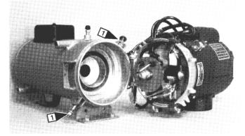
2. Unscrew the nozzle (1), use the nozzle wrench (see page 28, item 7.5) or two wrenches (16 mm and 19 mm). Make sure the ignition electrodes are not moved.
