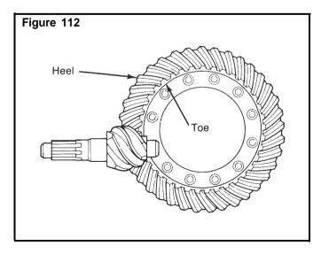
Always check tooth contact patterns on the drive side of the gear teeth. **Figure 113.**
