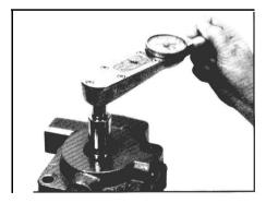
Check input shaft torque
