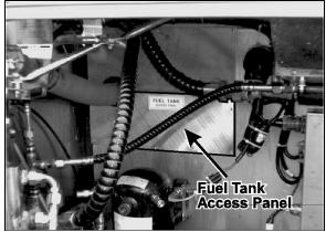
FIGURE 8: FUEL TANK ACCESS PANEL
