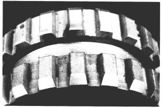
11. The fourth-fifth and sixth-seventh shift collars and gears have Taper-Lok<sup>™</sup> gear locks. They are designed to draw gears into perfect alignment and eliminate gear jump-out.
