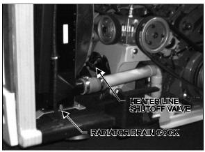
FIGURE 5: ENGINE COMPARTMENT
