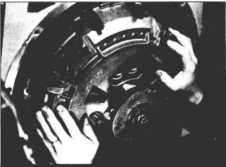
Position the clutch over the guide studs and slide it forward until contact is made with the flywheel surface.
