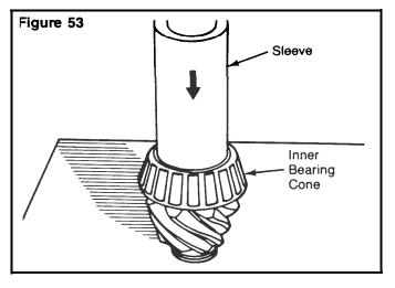
**5.** Press the inner bearing cone on the shaft of the drive pinion until the cone is flat against the gear head. Use a sleeve of the correct size against the bearing inner race.
