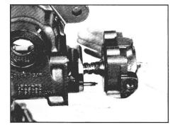
Install rack piston, worm, valve assembly 15
