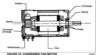
FIGURE 23: CONDENSER FAN MOTOR
