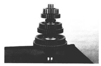
10. Place the externally splined thrust washer, snap ring and internally splined thrust washer in the gear. Slide sixth gear onto the shaft. Secure it with a snap ring.
