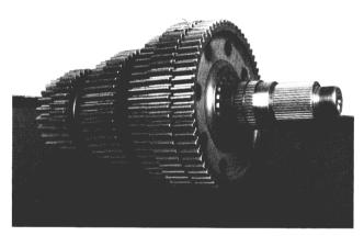
11. Place the shaft on the bench. Install reverse gear, Butt first and reverse gears together, and secure them with lockwire. This will provide the necessary clearance to install the mainshaft back into the case.
