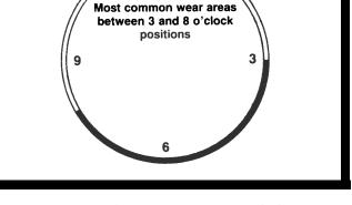
Most wear will be found on the lower half of these surfaces with the most common wear areas between the 3 and 8 o'clock positions.
