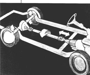
This means the driveshaft must be able to contract, expand and change operating angles when going over bumps or depressions. This is accomplished through universal joints, which permit the driveshaft to operate at different angles, and slip joints, which permit contraction or expansion to take place.
