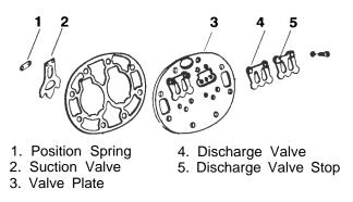
Figure 1-2. Suction & Discharge Valve
