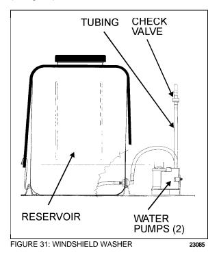
The windshield washer reservoir is located in the front service compartment (Fig. 31). This unit pumps the washer solvent to the spray nozzles where it is dispersed across the windshield. Adjust nozzles with a flat screwdriver as needed to get proper spray coverage.
