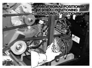
FIGURE 20: COMPRESSOR ALIGNMENT
