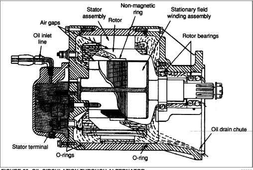
FIGURE 20: OIL CIRCULATION THROUGH ALTERNATOR
