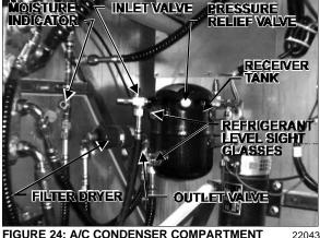
FIGURE 24: A/C CONDENSER COMPARTMENT
