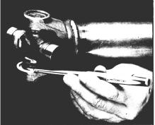
Removing an inside snap ring.
