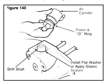
**9.** Install the cylinder into the housing bore. Make sure that the pilot journal on the piston is against its bore on the shift shaft. **Figure 141.**
