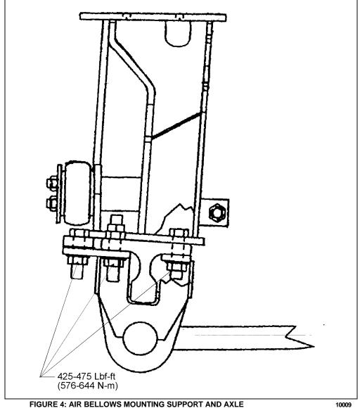
For more torque specifications, see "GKN Parts and Service Manual For Axles", Manual No. 1604, Issue A, Section B annexed to the end of this section, under heading "Tightening Torque Table for Type S82 Steer Axle".
