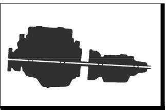
Don't let the rear of the transmission drop and don't let the transmission hang unsupported in the splined hubs of the driven discs because it distorts them and could cause poor clutch operation or clutch release problems.
