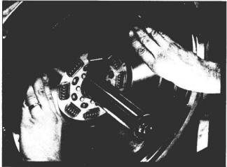
Next, install the intermediate plate by positioning the drive slots on the drive pins and remove the aligning tool.
