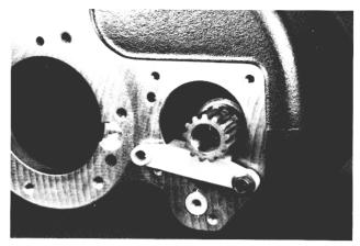
4. Insert the lower idler shaft with lockball.
