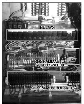
FIGURE 7: REAR ELECTRICAL COMPARTMENT 06054
