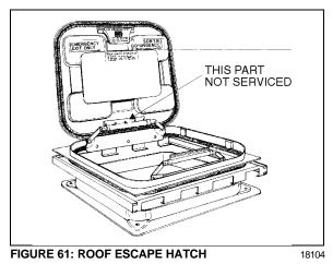
**Caution:** Hinge assembly is critical and hinge should never be removed from cover assembly. Fasteners used in this assembly are special and have critical torque requirements and tamper-resistant heads to discourage tampering.
