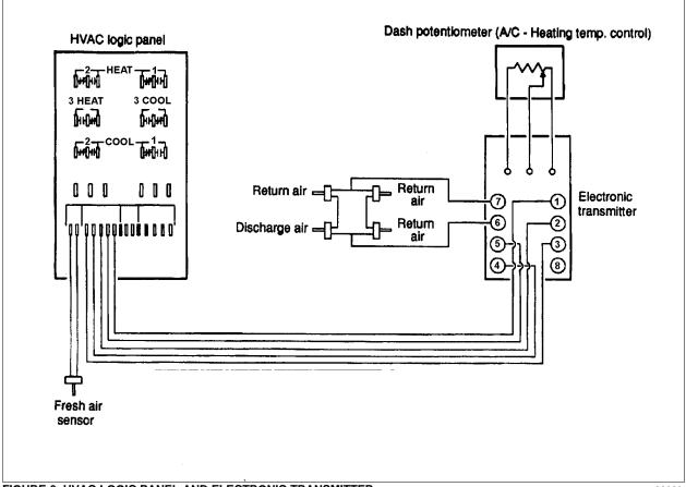
FIGURE 6: HVAC LOGIC PANEL AND ELECTRONIC TRANSMITTER
