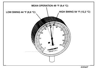
FIGURE 28: HIGH & LOW SWING TEMPERATURE AT REMOTE BULB
