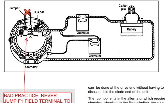
electrical checks are the field winding, the six d iodes, and the stator winding.
