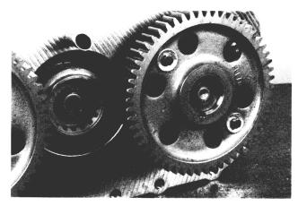
15. Slide the gear onto the shaft. Gather two of the 54103 (.375-1 6 x 3.00) grade eight bolts used for securing the clutch housing to the case, Place these in the two bolt holes in the gear, and thread them into the tapped installation holes provided in the case.
