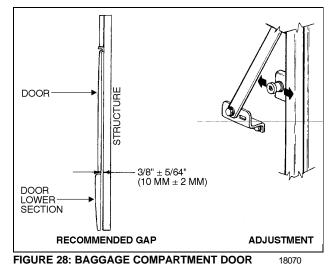
11.Recheck gap mentioned in step 9. If gap has changed, correct half the change by adjusting arm support fixed to structure. Loosen the bolt supporting balance arm on door lower section and close the door, gap adjustment will automatically result. Tighten the bolt from inside the compartment. Refer to figure 29.
