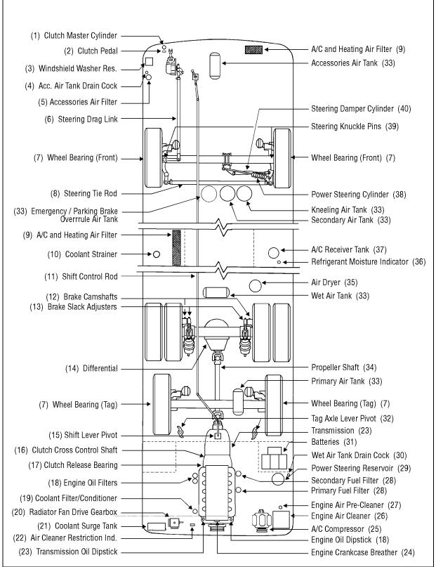
FIGURE 1: LUBRICATION AND SERVICING COMPONENTS
