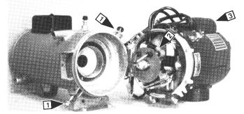
4. Lift up the ignition unit, disconnect wires (1) and unscrew the four screws (2) securing the protection cover (3).
