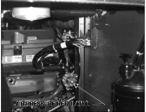
FIGURE 9: ENGINE COMPARTMENT R.H. SIDE 02003
