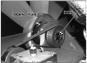
FIGURE 13: MECHANICAL LOCKING DEVICE 05033
