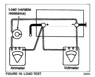
**Caution:** Observe polarity of the meters and the battery when making connections, and select the correct meter range.
