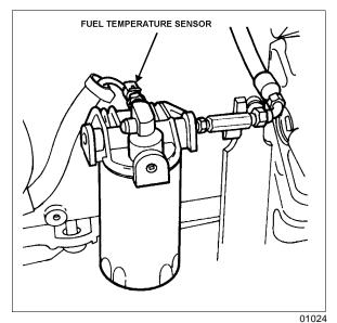
FIGURE 8: ENGINE FUEL TEMPERATURE SENSOR
