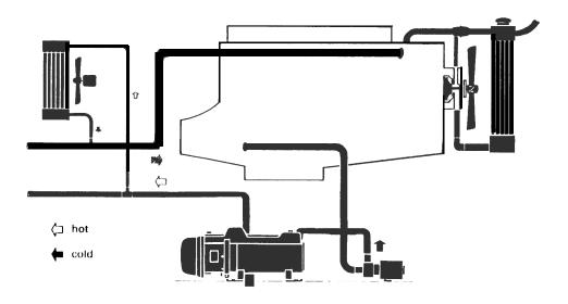
Figure 3 B: Installation in the coolant circulating system without heat exchangers
