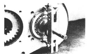
Countershaft front bearing puller (Snap-on-CJ 80).
