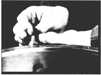
If the alignment and clearance is correct, lock each of the six pins in place with two, new, 3/8" by 3/8" set screws.
