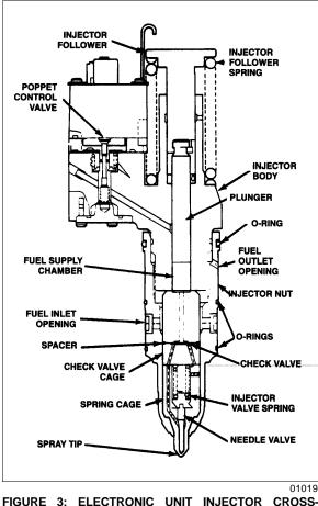
FIGURE 3: ELECTRONIC UNIT INJECTOR CROS SECTION
