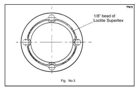
3.13 Fit hub cap along (3) within 5 minutes of applying sealant then secure with hub cap setscrews and washers (1 & 2) tightening setscrews to 85-103 lbs. ft. (115 - 140 Nm.).
