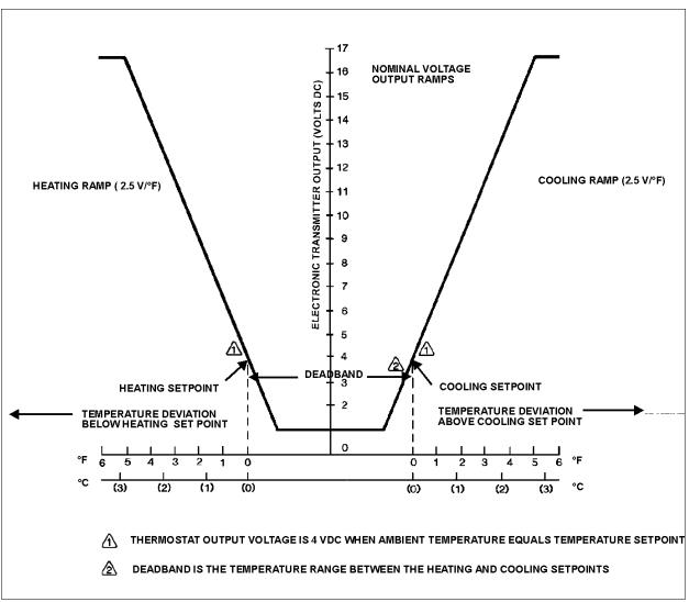
FIGURE 7: ELECTRONIC TRANSMITTER OUTPUT VOLTAGE RAMPS
