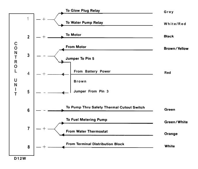
Power Input: + Pin #4 Red - Pin #3 Brown/Yellow Should failure occur, there are several items which should be checked first before any major troubleshooting is done.
