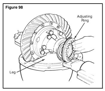
7. Install the bearing caps over the bearings and adjusting rings in the correct location as marked before removal. **Figure 99.**
