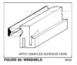
**Caution:** Sikaflex adhesive hardens quickly. Continue installation immediately after application of adhesive is completed.
