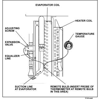
FIGURE 27: SUPERHEAT ADJUSTMENT INSTALLATION
