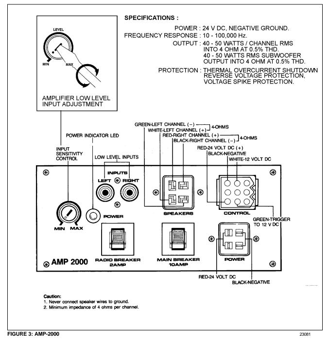
The AMP-2000 brings an added dimension to your stereo equipment and increases the total output of the system. The amplifier will perform with any unit operating in a 24-volt with negative ground electric system. The AMP-2000 is located over front wheelhousing. To access, open the first baggage compartment door.
