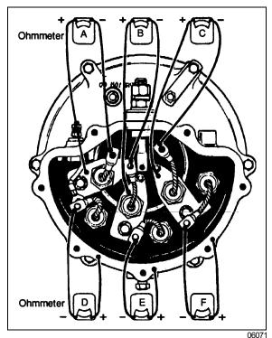
FIGURE 25: CHECKING DIODES WITH OHMMETER ON A TYPICAL OIL COOLED ALTERNATOR (END COVER REMOVED)
