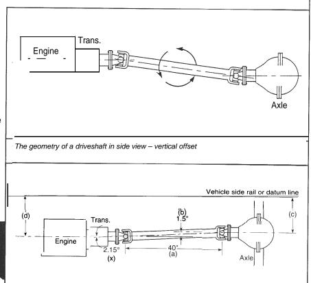
The geometry of a driveshaft in p/an view - horizonta/ offset
