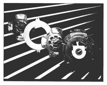
**Note:** This clutch comes with 14" dampened ceramic super-duty discs which cannot be mixed or matched with other discs.
