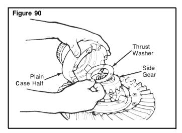
Put the plain half of the differential case over the flange half and gears. Rotate the plain half as needed to align the match marks. Figure 90 and 91.
