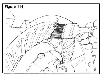
3. Rotate ring gear forward and backward so that the 12 gear teeth go past the drive pinion six times to get the contact patterns. Repeat if needed to get a more clear pattern.
