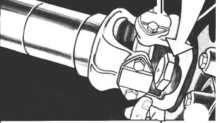
Check the output and input end yokes on both the transmission and axle, or axles, for looseness. If loose, disconnect the driveshaft and retorque the end yoke retaining nut to specification. If yoke replacement is required, check for manufacturer's recommendation regarding replacement frequency of the end yoke retaining nut.
