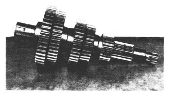
1. This view shows the hub direction of the gears. Firstreverse gear is an integral part of the shaft, while the remaining gears are secured with individual woodruff keys under each gear.
