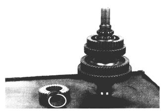
3. Remove fifth gear. There are two thrust washers and a snap ring inside the gear. There is also a gear bore snap ring inside each gear except reverse gear. This snap ring need not be removed unless otherwise specified.
