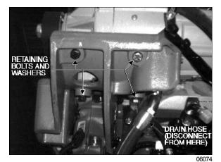
FIGURE 28: ALTERNATOR RETAINING BOLTS AND WASHERS
