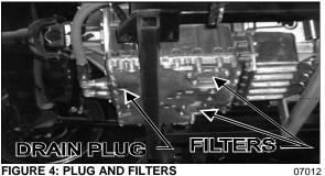
FIGURE 4: PLUG AND FILTERS
