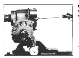
Tighten adjusting 2 screw
