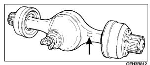
FIGURE 3: TYPICAL SERIAL AND MODEL NUMBERS
