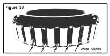
F. Damage on rollers and on surfaces of the cup and cone inner race that touch the rollers. Figure 39.
