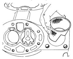
Figure 3-19. Installing Suction Strainer
