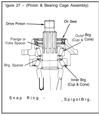
1. Put the drive pinion and bearing cage in a press. The pinion shaft must be toward the top of the assembly. **Figure 28.**
