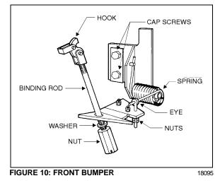
Partly recline the bumper, remove both chain end snap hooks from their attaching points, and let the bumper rest face down on the lifting equipment platform. 4. Ask assistant to relieve spring tension on one eye bolt with proper tool. Remove 2 nuts and eye bolt holding spring and slowly release spring. Repeat procedure for the other eye bolt.
