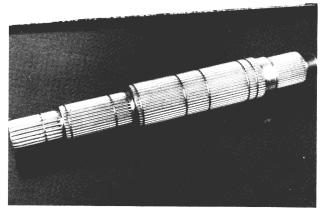
10. Notice that the mainshaft has rolled involute splines. They provide greater strength which means longer life.
