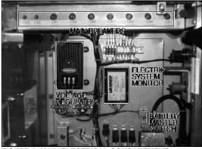
FIGURE 5: MAIN ELECTRICAL COMPARTMENT 06052
