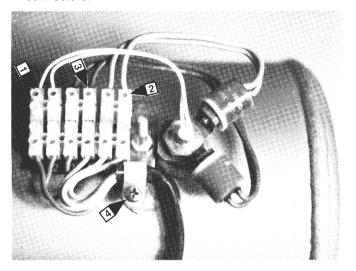
2. Remove block connectors A and B from the control unit and disconnect the fuel lines from the heater connection pipes. Plug the pipes.
