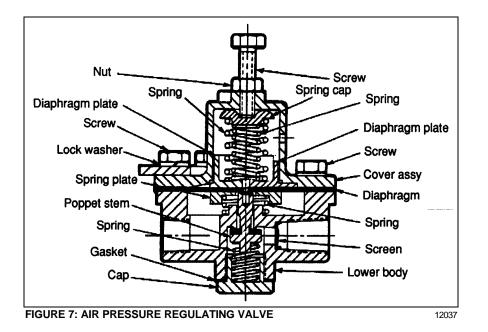
The belt tensioner pressure regulating valve controls pressure in the three belt tensioner cylinders as these latter are parallel mounted. It is located on the structure post at left of the oil reserve tank in engine compartment and is used to limit the air pressure in belt tensioners to  $50 \pm 2$  psi (345 ± 15 kPa).
