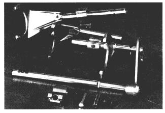
2. Reassemble the forks and brackets. Torque the allenhead setscrews to 26-32 ft. lbs. Torque the second-third bracket screws to 13-18 ft. tbs.
