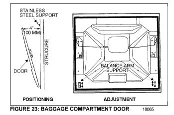
Fully open the door, loosen the two bolts retaining each gas cylinder support to structure, position door parallel with adjacent doors and complete tightening bolts. A measure of 6" ± 1/4", (150 mm ± 7 mm) between door panel lip (at level of upper edge of lower section) and the lateral panel is given as a guide. Refer to figure 24.
