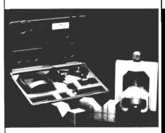
CAUTION: Never heat components or use sledge hammers and floor jacks to disassemble driveshafts. This can result in damaged, weakened or bent components.
