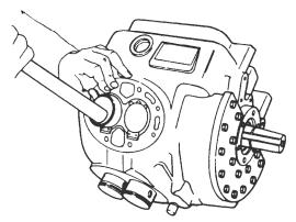
**Figure 3-18. Installing Pistons**
