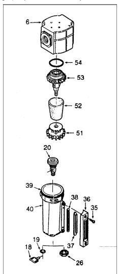
FIG. 4: ACCESSORY AIR FILTER ASSEMBLY 12088
