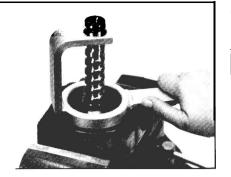
Assemble new locknut
