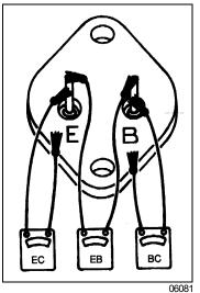
FIGURE 35: CHECKING TRANSISTORS TR1
