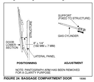
**Caution:** For converted vehicles provided with "Awning" windows, fully open window then adjust door opening angle so the door does not interfere with window.
