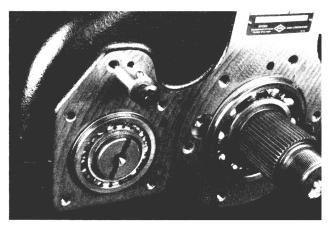
4. Insert a capscrew into the upper reverse idler shaft for removal. Don't lose the lockball in the shaft.
