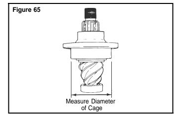
I. Use the following procedure to calculate the bearing preload (torque).
