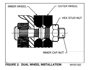
**Caution:** Do not attempt to tighten an inner cap nut without having previously loosened the hex head nut.
