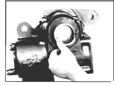
Install retaining 2 ring Install the second retaining ring (36) seating it firmly in the housing retaining ring groove.
