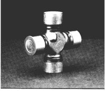
If the universal joint kit is replaced, it must be replaced with a kit designed specifically for use with aluminum. The use of non-endurion coated kits will result in damage to the driveshaft through galvanic corrosion.
