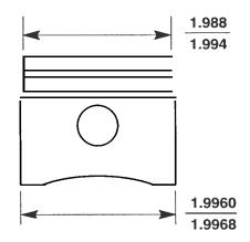
Figure 3-20. Piston Dimension (Wear Limits)
