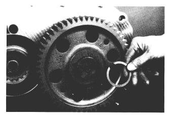
9. Remove the snap rings from the countershafts,
