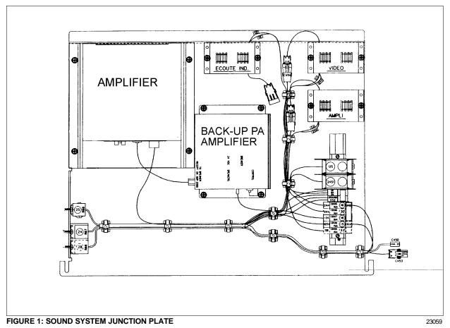
Each service module mounted to the underside of the parcel racks contains a 40-watt speaker. The speakers in passenger section (Twelve H3-41 or sixteen H3-45) are wired in stereo and are powered by the amplifier. A BACK-UP PA MODULE with volume control and one microphone outlet mounted in driver's area are provided as standard equipment.
