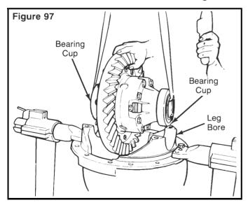
5. Safely lift the differential and ring gear assembly and install into the carrier. The bearing cups MUST be flat against the bores between the carrier legs. **Figure 97.**  6. Install both of the bearing adjusting rings into position between the carrier legs. Turn each adjusting ring hand tight against the bearing cup. **Figure 98.**
