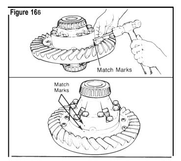
2. Remove the lock wire\* capscrews' and washers\* or bolts\*, nuts\* and washers that hold the case halves together.
