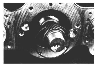
16. Remove the remaining gear bore snap ring.
