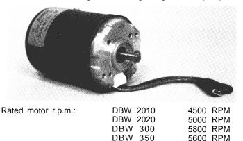
Checks: Check the mounting condition (rough running). The single parts of the motor cannot be exchanged. The cables and the drain hole must show downwards.
