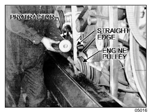
FIGURE 19: MEASURING ENGINE PULLEY VERTICAL ANGLE
