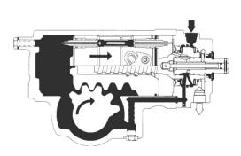
Steering Wheel Input: Counter-Clockwise Rotation
