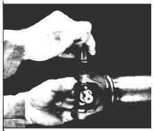
5. Repeat steps 3 and 4 to install the opposite bearing assembly. If the joint is stiff, strike the yoke ears with a soft hammer to seat the needle bearings.
