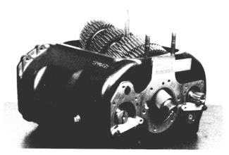
6. Lower the mainshaft assembly into the case.
