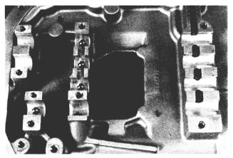
1. Lube all parts prior to reassembly. Clean the cover, then install the springs, poppets and interlocks.
