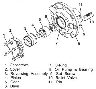
Figure 3-5. Low Profile Gear Oil Pump
