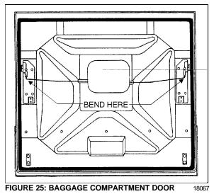
8. Install both striker pins, bring the door close to them, and adjust the height of pins so they are well centered with latches. Refer to figure 26.
