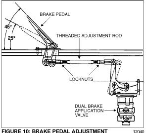
FIGURE 10: BRAKE PEDAL ADJUSTMENT
