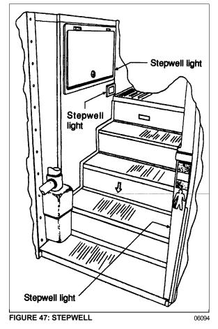
Stepwell lights are illuminated when the door opening system is activated (Fig. 47).
