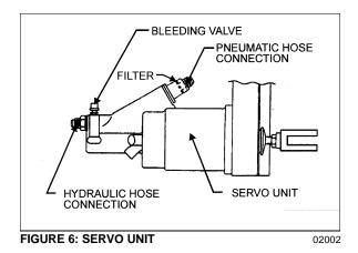
3. Remove the plastic tube on the bleeding valve. Make sure the bleeding valve is open. Force fluid (meeting DOT 3 specifications) through the bleeding valve opening. Tighten teflon flexible hose connector when fluid is free of air bubbles. Continue to force brake fluid until it enters master cylinder reservoir and flows free of air bubbles.
