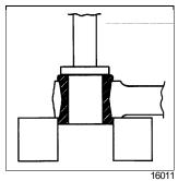
FIGURE 7: RADIUS ROD BUSHING REMOVAL
