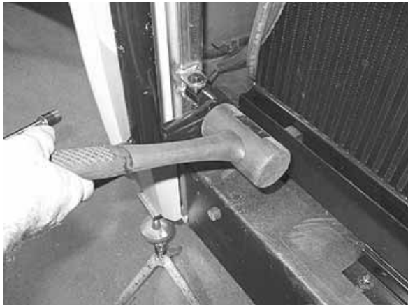
FIGURE 60: PANTOGRAPH ARM ADJUSTMENT
