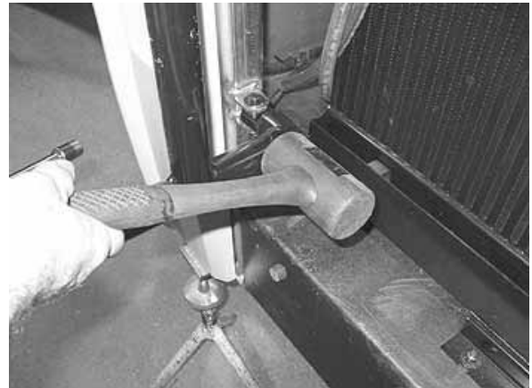
FIGURE 64: PANTOGRAPH ARM ADJUSTMENT
