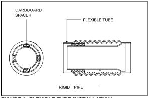
FIGURE 3: FLEXIBLE TUBE INSTALLATION
