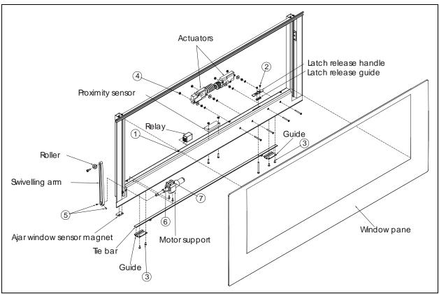
FIGURE 40: ELECTRIC AWNING WINDOW EXPLODED VIEW (SASH)
