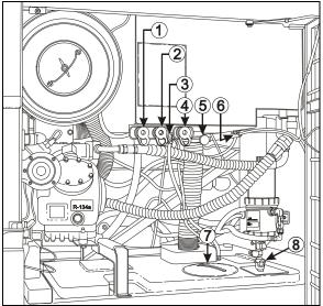
FIGURE 27: F/W TANK SERVICE VALVES
