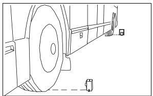
FIGURE 56: INSTALLING CALIBRATION FIXTURES 06497
