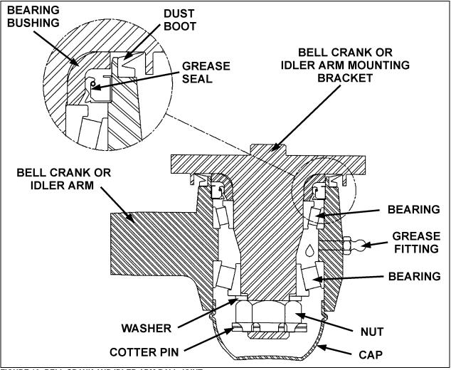
FIGURE 10: BELL CRANK AND IDLER ARM BALL JOINT
