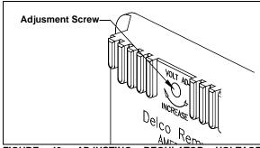
FIGURE 43: ADJUSTING REGULATOR **VOLTAGE SETTING**
