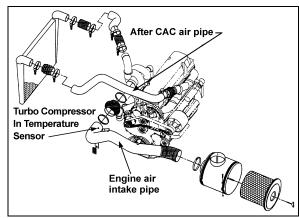
FIGURE 9: TURBO COMPRESSOR IN TEMPERATURE SENSOR LOCATION
