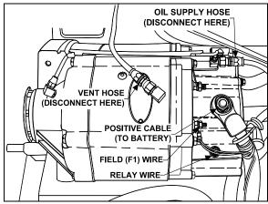
FIGURE 37: ALTERNATOR (HOSES AND WIRES)
