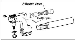
FIGURE 3: TIE ROD END PLAY ADJUSTMENT
