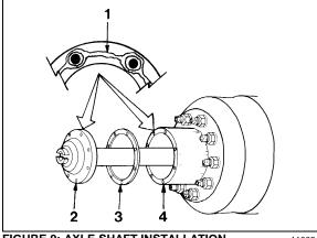
FIGURE 9: AXLE SHAFT INSTALLATION
