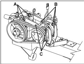
FIGURE 35: COMPRESSOR REMOVAL OR INSTALLATION
