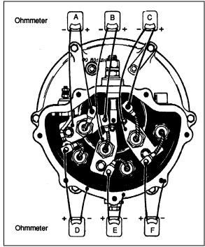
FIGURE 34: DIODE TESTING
