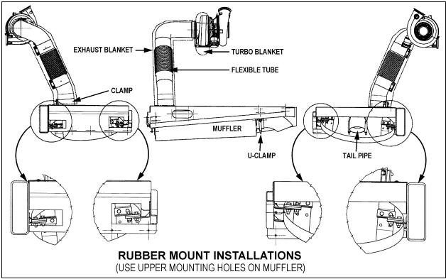
FIGURE 1: EXHAUST SYSTEM - XL2-40 & 45E (SHELL) INSTALLATION
