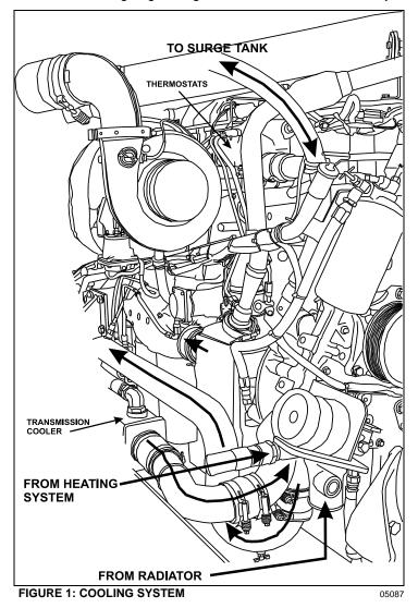
From the cylinder block, the coolant passes up through the cylinder head and, when the engine is at normal operating temperature, it goes through the thermostat housing and into the upper portion of the radiator. The coolant then passes through a series of tubes where its heat is dissipated by air streams created by the revolving fan and the motion of the vehicle.
