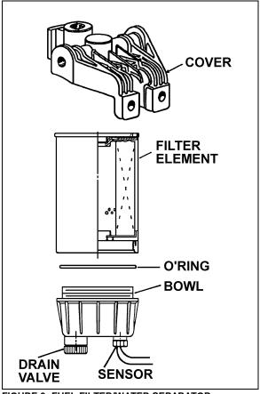
FIGURE 3: FUEL FILTER/WATER SEPARATOR
