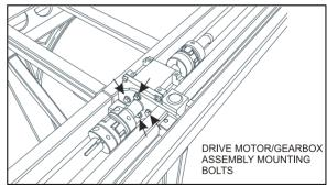
FIGURE 18: DRIVE MOTOR/GEARBOX ASSEMBLY MOUNTING BOLTS
