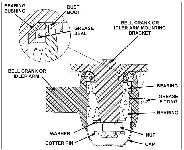
FIGURE 10: BELL CRANK AND IDLER ARM 16
