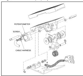
FIGURE 11: ELECTRONIC FOOT PEDAL ASSEMBLY03035
