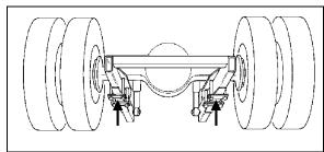
FIGURE 6: JACKING POINTS ON DRIVE AXLE
