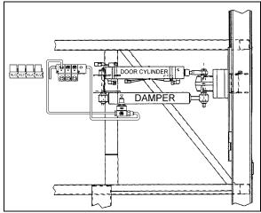
FIGURE 16: DOOR CYLINDER AND DAMPER
