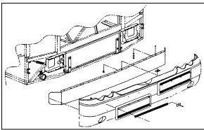
FIGURE 27: FRONT BUMPER REMOVAL
