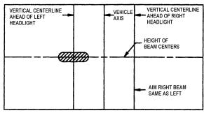
FIGURE 58: HIGH-INTENSITY ZONE (SHADED AREA) OF A PROPERLY AIMED UPPER BEAM ON THE AIMING SCREEN 7.6 M (25FT) IN FRONT OF VEHICLE 06503
