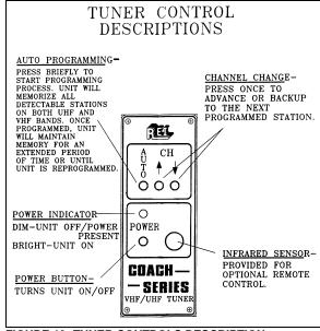
FIGURE 13: TUNER CONTROLS DESCRIPTION
