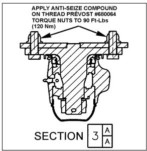
FIGURE 3: CLAMP POSITIONING
