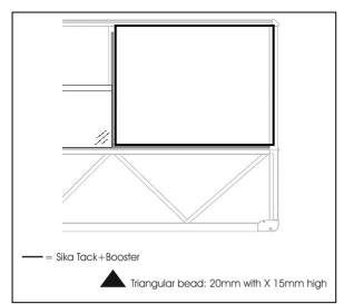
FIGURE 56: FACE FIXED WINDOW INSTALLATION - SIKA TACK+BOOSTER
