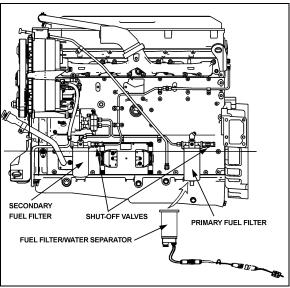
FIGURE 2: MANUAL SHUT-OFF VALVES
