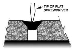
13. If welding was not performed properly, there will a loss of adhesion on one side. If this is the case, repair the joint.
