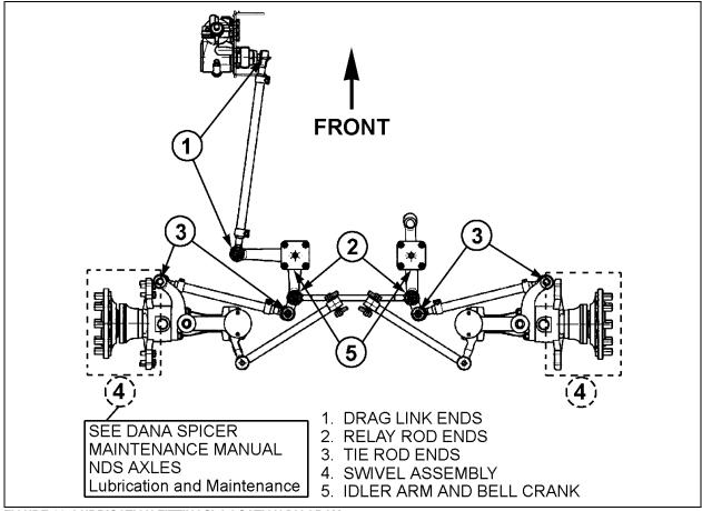
FIGURE 11: LUBRICATION FITTINGS' LOCATION DIAGRAM
