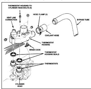
FIGURE 13: THERMOSTAT AND RELATED PARTS 05034
