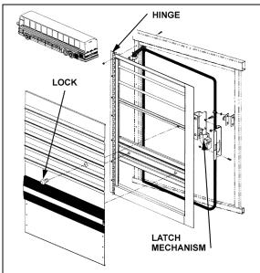
FIGURE 49: L.H. SIDE REAR SERVICE COMPARTMENT DOOR
