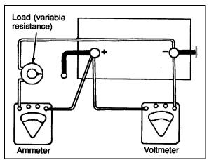
FIGURE 26: LOAD TEST
