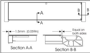
FIGURE 49: BOTTOM PANEL INSTALLATION
