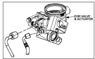
FIGURE 6: EGR VALVE & ACTUATOR ASSEMBLY
