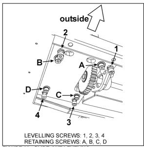
FIGURE 22: SLIDE-OUT LEVELING
