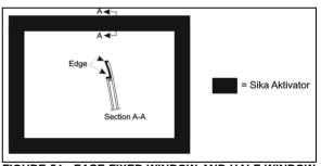
FIGURE 54 : FACE FIXED WINDOW AND HALF-WINDOW – SIKA AKTIVATOR
