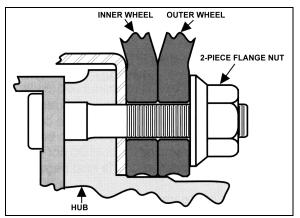
FIGURE 5: HUB-MOUNTED WHEELS
