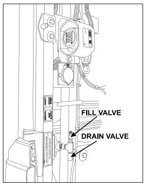
FIGURE 31: REAR VALVE LOCATION
