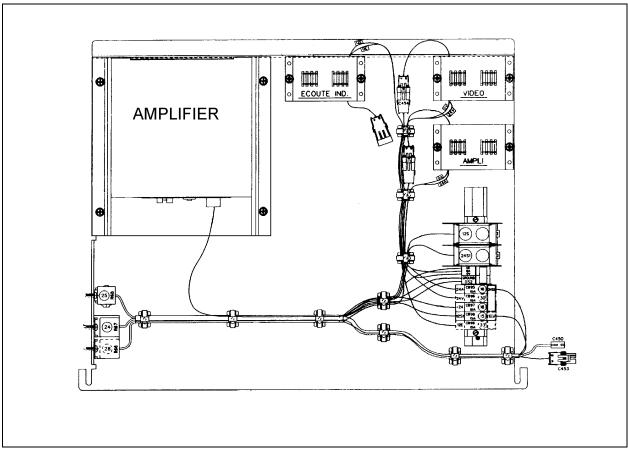
FIGURE 1: SOUND SYSTEM JUNCTION PLATE
