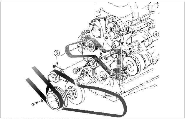
FIGURE 28: TWIN BOSCH ALTERNATORS INSTALLATION
