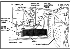
FIGURE 28: A/C CONDENSER COMPARTMENT
