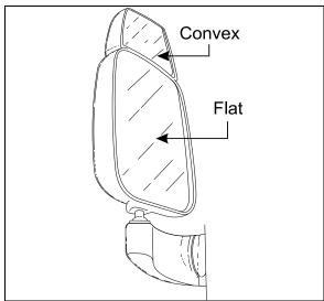
FIGURE 51: REAR VIEW MIRROR (RAMCO)
