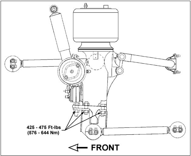
FIGURE 7: AIR BELLOWS MOUNTING SUPPORT AND AXLE
