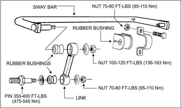
FIGURE 26: SWAY BAR (REAR SUSPENSION)
