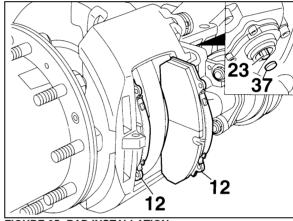
FIGURE 35: PAD INSTALLATION
