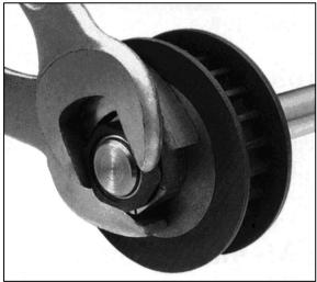
FIGURE 14: KEYLESS BUSHING TIGHTENING
