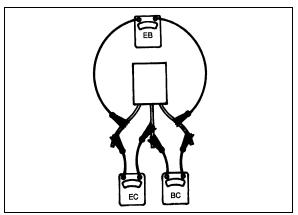
FIGURE 46: CHECKING TRANSISTOR TR2
