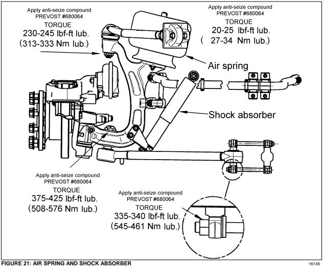
FIGURE 21: AIR SPRING AND SHOCK ABSORBER
