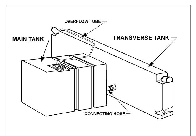
FIGURE 7: 250 US GALLONS FUEL TANKS (MAIN TANK & TRANSVERSE FUEL TANK) (MTH 40 & MTH 45E)
