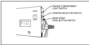
FIGURE 22: REAR JUNCTION BOX SWITCHES
