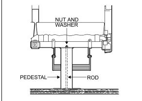
FIGURE 34: SEAT PEDESTAL ASSEMBLY
