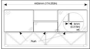
FIGURE 59: FACE FIXED WINDOW INSTALLATION
