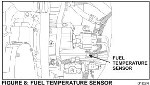
FIGURE 8: FUEL TEMPERATURE SENSOR
