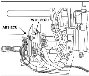
FIGURE 16: WTEC / ELECTRONIC CONTROL UNIT 07075
