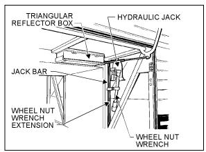
FIGURE 8: FORWARD R. H. SIDE COMPARTMENT 23012
