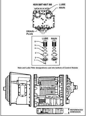
FIGURE 7: DRAIN PLUG AND FILTERS
