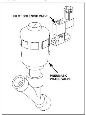
FIGURE 53: CENTRAL HOT WATER PNEUMATIC VALVE ASSEMBLY 22240
