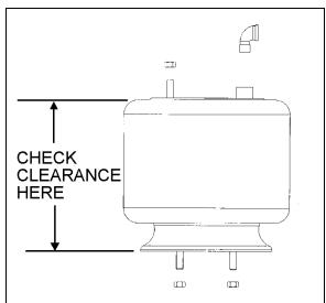
FIGURE 25: TYPICAL AIR SPRING CLEARANCE
