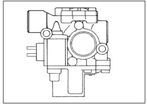
FIGURE 44: ABS MODULATOR VALVE
