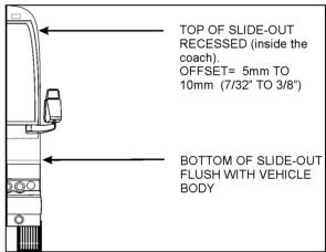
FIGURE 23: TILT ADJUSTMENT
