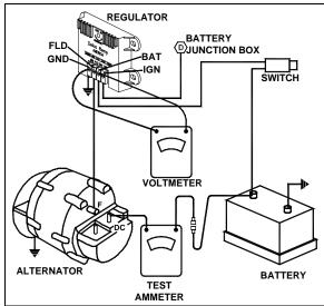
FIGURE 42: REGULATOR VOLTAGE SETTING
