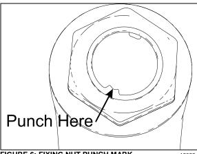
FIGURE 6: FIXING NUT PUNCH MARK
