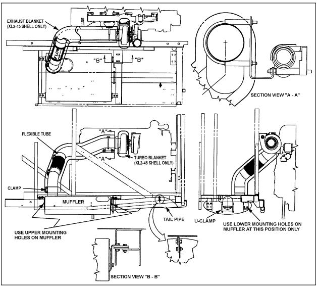
FIGURE 2: EXHAUST SYSTEM - XL2-45 (COACH & SHELL) INSTALLATION
