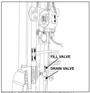
FIGURE 2: REAR VALVE LOCATION (TYPICAL)
