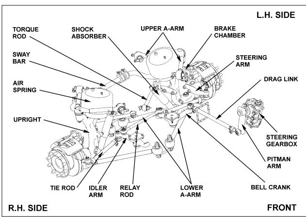
FIGURE 1: SUSPENSION AND STEERING LINKAGE
