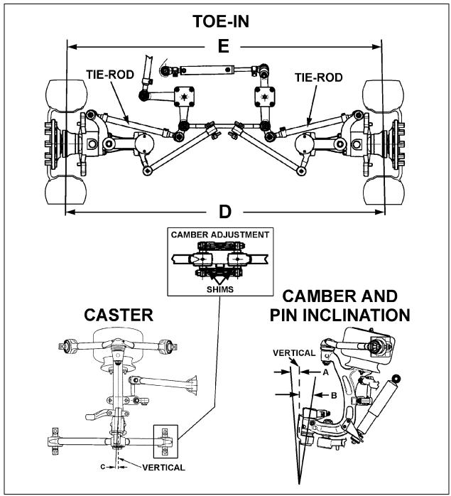
FIGURE 21: FRONT END ALIGNMENT DIAGRAM
