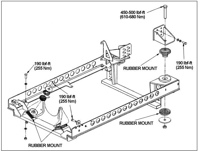
FIGURE 20: POWER PLANT CRADLE INSTALLATION
