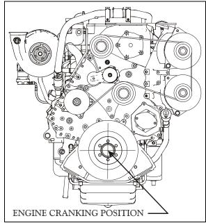
FIGURE 11: ENGINE CRANKING POSITION
