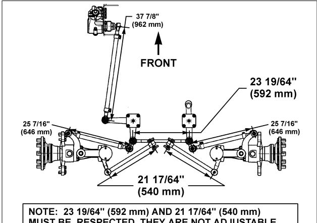
NOTE: 23 19/64" (592 mm) AND 21 17/64" (540 mm) MUST BE RESPECTED, THEY ARE NOT ADJUSTABLE. OTHER LENGTH ARE ADJUSTABLE, THEY ARE GIVEN ONLY FOR PRELIMINARY ADJUSTMENT. ALL LENGTHS ARE MEASURE FROM CENTER TO CENTER END OF ROD.
