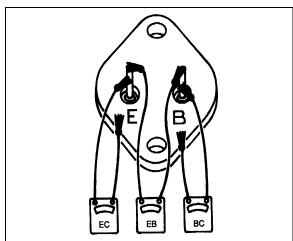
FIGURE 45: CHECKING TRANSISTOR TR1
