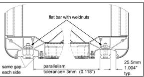
FIGURE 24: RAIL POSITIONING
