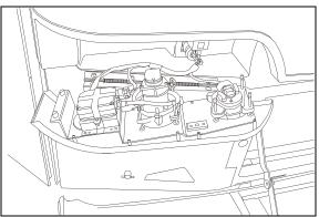
FIGURE 49: OPENING HEADLIGHT ASSEMBLY
