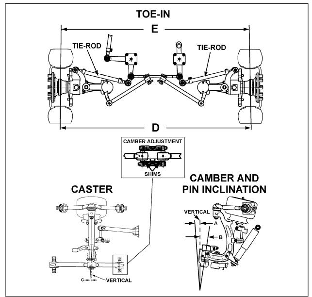
FIGURE 19: FRONT END ALIGNMENT DIAGRAM
