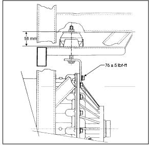
FIGURE 14: NUT TOLERANCE
