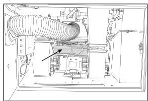
FIGURE 10: EVAPORATOR COIL CLEANING
