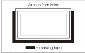
FIGURE 63: MASKING TAPE APPLICATION
