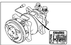
FIGURE 38: COMPRESSOR OIL LABEL
