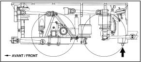
FIGURE 54: REAR SUBFRAME JACKING POINTS
