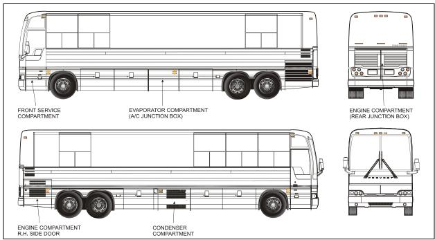
FIGURE 12: ELECTRICAL COMPARTMENTS (XL2-40 BUS SHELLS)
