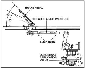
FIGURE 12: BRAKE PEDAL ADJUSTMENT
