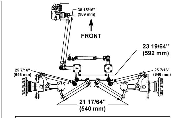
NOTE: 23 19/64" (592 mm) AND 21 17/64" (540 mm) MUST BE RESPECTED, THEY ARE NOT ADJUSTABLE. OTHER LENGTH ARE ADJUSTABLE, THEY ARE GIVEN ONLY FOR PRELIMINARY ADJUSTMENT. ALL LENGTHS ARE MEASURE FROM CENTER TO CENTER END OF ROD.
