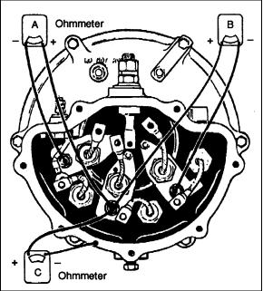
FIGURE 36: STATOR WINDING TEST
