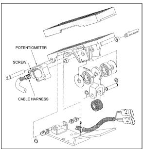
FIGURE 13: ELECTRONIC FOOT PEDAL ASSEMBLY03035
