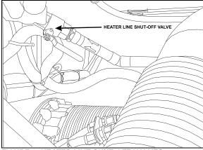
FIGURE 6: HEATER LINE SHUT-OFF VALVES
