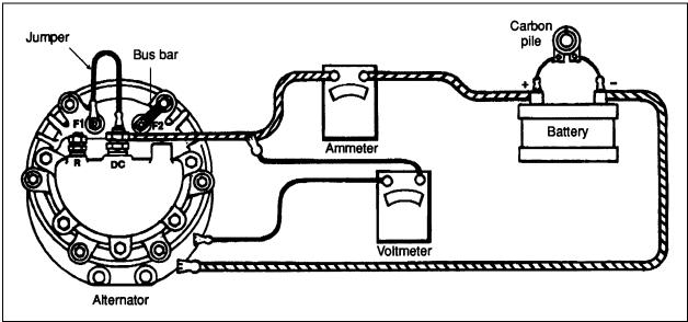
FIGURE 32: CONNECTIONS FOR CHECKING ALTERNATOR OUTPUT
