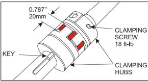
FIGURE 20: JAW COUPLING
