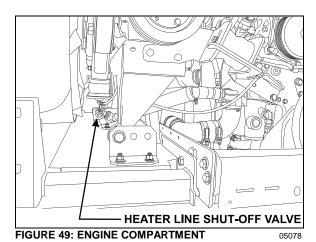
On XL2-45 vehicles, one valve is located in the engine compartment, under the radiator fan gearbox (Fig. 49), another valve is located in the engine compartment behind splash guard panel
