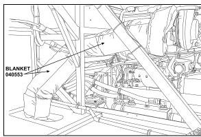
FIGURE 4: EXHAUST BLANKET INSTALLATION
