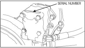
FIGURE 7: POWER STEERING PUMP NAMEPLATE 00035
