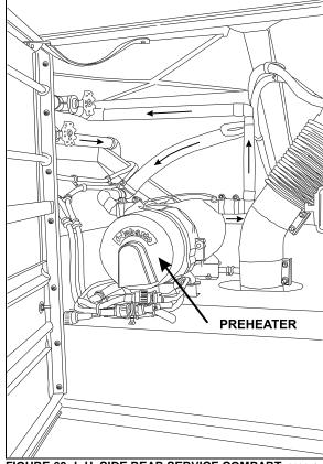
FIGURE 60: L.H. SIDE REAR SERVICE COMPART. 22245A
