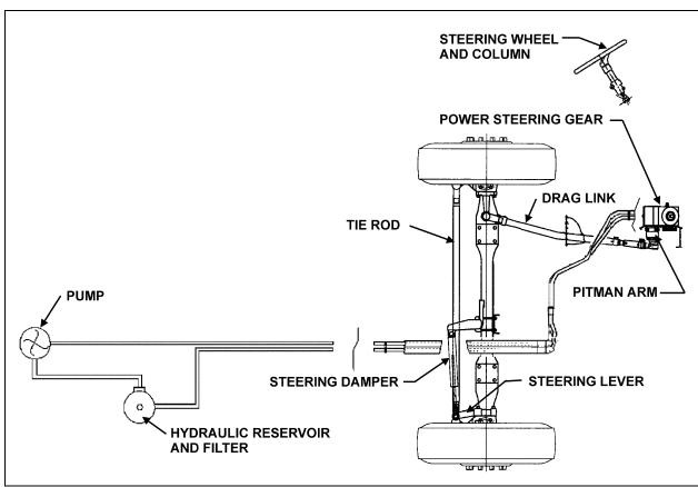
FIGURE 1: STEERING SYSTEM AXLE SETUP
