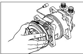
FIGURE 37: ROTATING MAGNETIC CLUTCH
