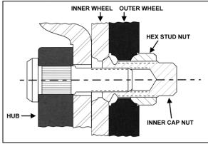
FIGURE 4: STUD-MOUNTED WHEELS
