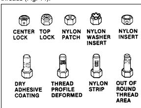
FIGURE 14: SELF-LOCKING FASTENERS
