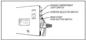
FIGURE 10: REAR JUNCTION BOX SWITCHES 010
