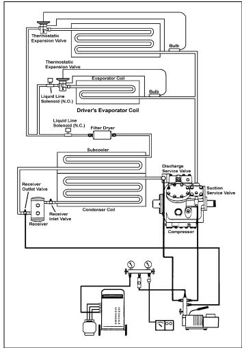
FIGURE 21: DOUBLE SWEEP EVACUATION SET-UP
