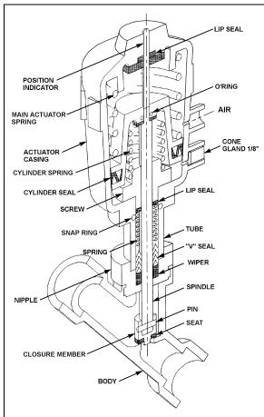
FIGURE 54: PNEUMATIC WATER VALVE
