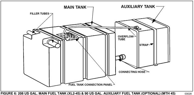
FIGURE 6: 208 US GAL. MAIN FUEL TANK (XL2-45) & 90 US GAL. AUXILIARY FUEL TANK (OPTIONAL) (MTH 45)
