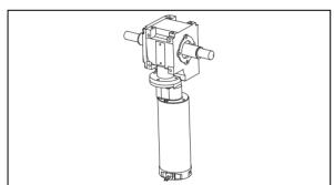
FIGURE 17: ELECTRIC MOTOR AND SPEED REDUCTION GEARBOX
