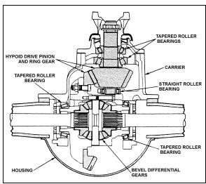
FIGURE 2: DIFFERENTIAL ASSEMBLY
