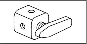
FIGURE 22: THREE-WAY VALVE
