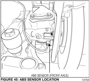
FIGURE 45: ABS SENSOR LOCATION
