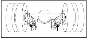
FIGURE 57: JACKING POINTS ON DRIVE AXLE OEH3B762
