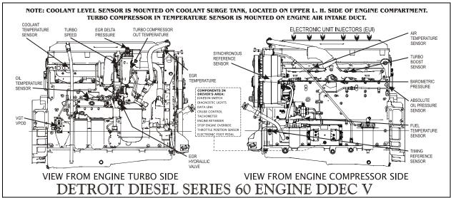
FIGURE 1: DETROIT DIESEL SERIES 60 ENGINE (TYPICAL)
