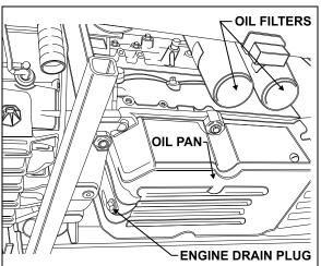
FIGURE 14: ENGINE DRAIN PLUG AND OIL FILTERS
