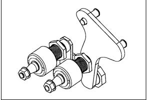
FIGURE 37: DRIVING MECHANISM (MOTOR SIDE) 23254
