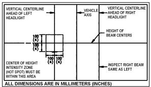
FIGURE 60: AIM INSPECTION LIMITS FOR UPPER-BEAM HEADLIGHTS 06505
