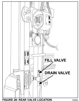
FIGURE 28: REAR VALVE LOCATION
