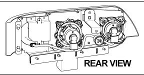
FIGURE 50: HEADLIGHT ASSEMBLY REAR VIEW 06548
