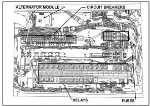
FIGURE 7: TOP SECTION OF FRONT SERVICE COMPARTMENT 06319
