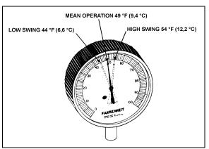
FIGURE 33: HIGH & LOW SWING TEMPERATURE AT REMOTE BULB 22047
