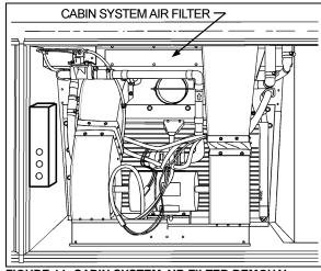
FIGURE 14: CABIN SYSTEM AIR FILTER REMOVAL22178E
