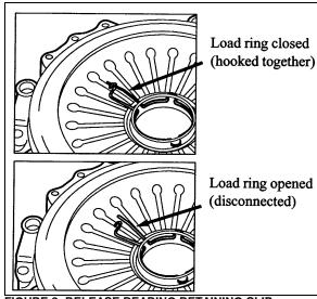
FIGURE 8: RELEASE BEARING RETAINING CLIP 0711
