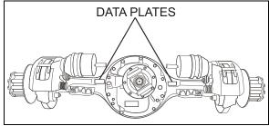
FIGURE 4: TYPICAL SERIAL & MODEL NUMBERS 110
