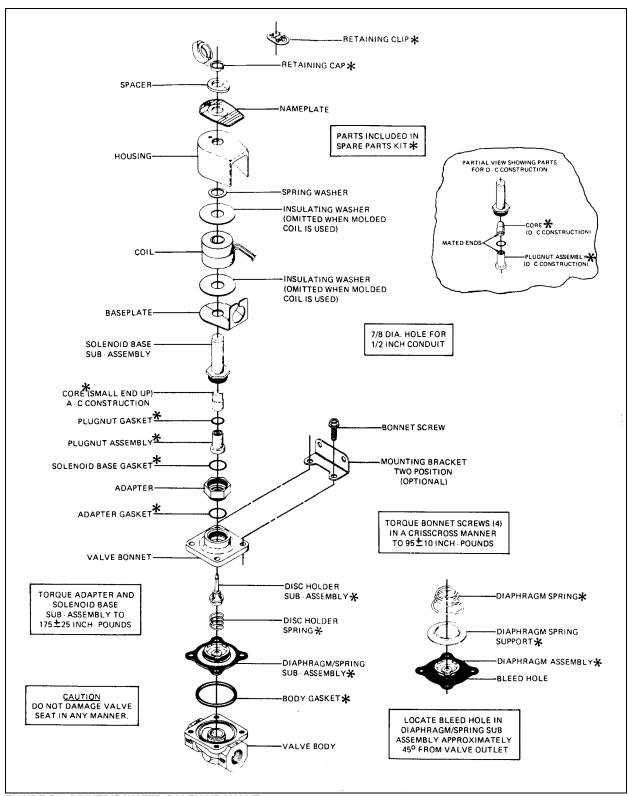
FIGURE 52: DRIVER'S WATER SOLENOID VALVE
