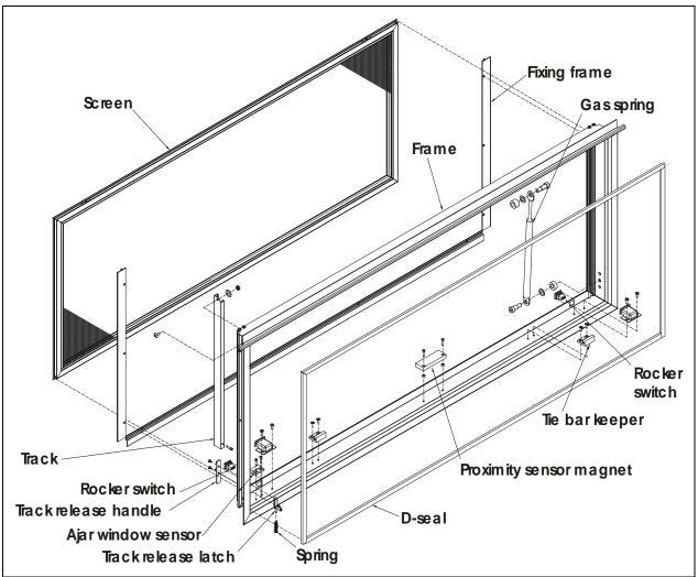
FIGURE 39: ELECTRIC AWNING WINDOW EXPLODED VIEW (FRAME)
