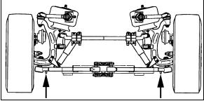
FIGURE 55: JACKING POINTS ON IND. SUSPENSION 16095
