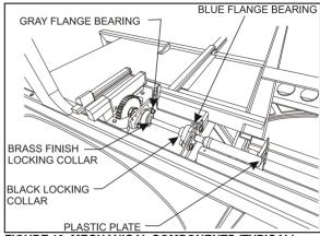
FIGURE 13: MECHANICAL COMPONENTS (TYPICAL)
