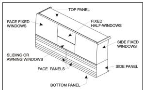
FIGURE 40 : SLIDE-OUT PANELS AND WINDOWS
