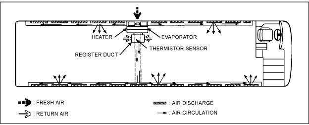
FIGURE 3: CENTRAL HVAC SYSTEM AIR CIRCULATION
