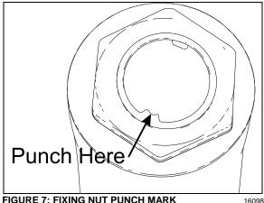
FIGURE 7: FIXING NUT PUNCH MARK
