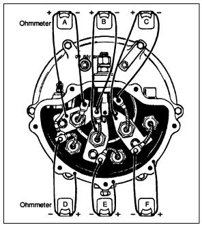
FIGURE 35: DIODE TESTING
