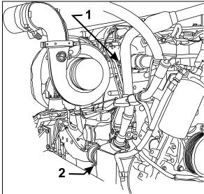
FIGURE 8: ENGINE COOLANT DRAIN COCKS
