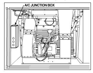
FIGURE 17: LOCATION OF A/C JUNCTION BOX IN EVAPORATOR COMPARTMENT
