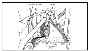
FIGURE 11: MECHANICAL LOCKING DEVICE
