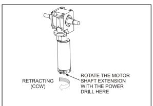
FIGURE 92: SLIDE-OUT MOTOR ROTATION
