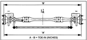
FIGURE 6: TOE-IN MEASUREMENTS
