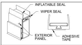
FIGURE 30 : SEAL ASSEMBLY
