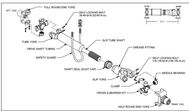
FIGURE 1: PROPELLER SHAFT ASSEMBLY
