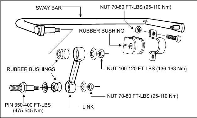
FIGURE 24: SWAY BAR (REAR SUSPENSION)
