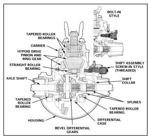
FIGURE 3: DRIVER-CONTROLLED DIFFERENTIAL LOCK
