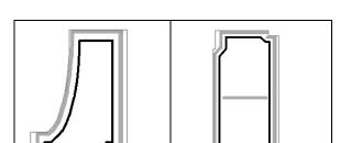
Apply evenly around the perimeter of the panel. Use two clothes, first one applies product while second one immediately dries surface off before product evaporation.
