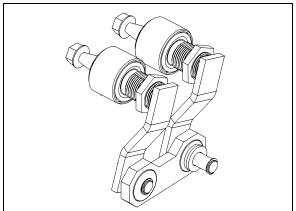
FIGURE 36: DRIVING MECHANISM (DRIVER SIDE) 23334
