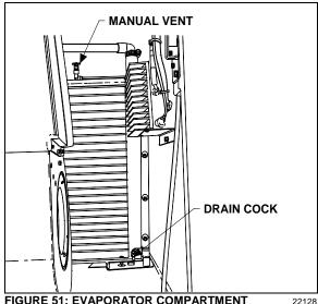
FIGURE 51: EVAPORATOR COMPARTMENT
