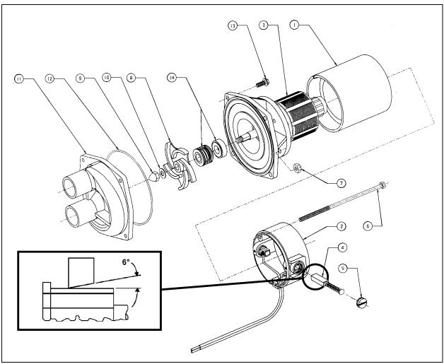
FIGURE 56: WATER RECIRCULATING PUMP (CONVERTED VEHICLE - CENTRAL A/C)
