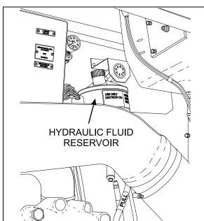
FIGURE 7: HYDRAULIC FLUID RESERVOIR LOCATION
