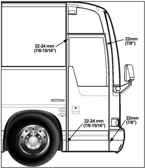
FIGURE 22: SEAL COMPRESSION ADJUSTMENT
