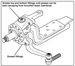
FIGURE 2: FRONT AXLE GREASING POINTS
