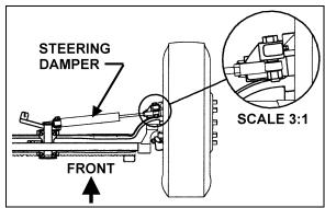
FIGURE 9: STEERING STABILIZER (DAMPER)
