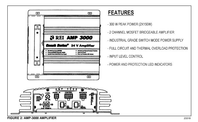
The AMP-3000 brings an added dimension to your stereo equipment and increases the total output of the system. The amplifier will perform with any unit operating in a 24-volt with negative ground electric system. The AMP-3000 is located on the first baggage compartment ceiling. To access, open the first baggage compartment door.
