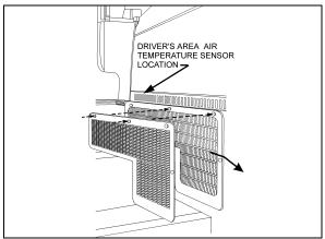
FIGURE 12: DRIVER'S AREA AIR FILTERS
