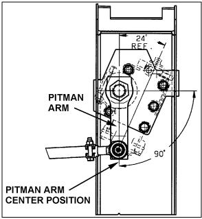
FIGURE 8: PITMAN ARM ALIGNMENT
