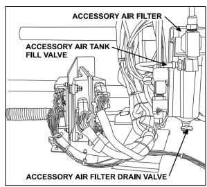
FIGURE 3: FRONT SERVICE COMPARTMENT
