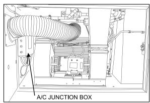
FIGURE 5: LOCATION OF A/C JUNCTION BOX IN EVAPORATOR COMPARTMENT 222244B
