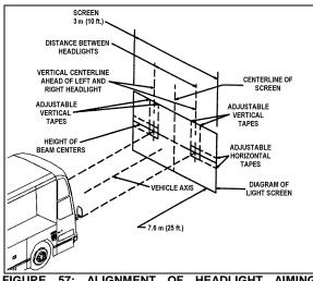
FIGURE 57: ALIGNMENT OF HEADLIGHT AIMING SCREEN 06502
