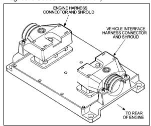
FIGURE 2: ELECTRONIC CONTROL MODULE (ECM)
