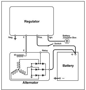
FIGURE 41: TYPICAL WIRING DIAGRAM OF A
