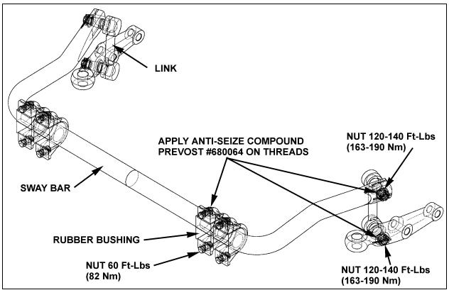
FIGURE 23: SWAY BAR (FRONT SUSPENSION)
