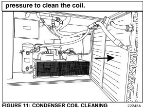
FIGURE 11: CONDENSER COIL CLEANING
