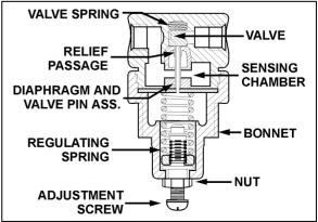
FIGURE 6: AIR PRESSURE REGULATING VALVE 12141B
