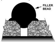
10. Shave filler bead to make it level to the floor. Use supplied knife designed for that purpose.
