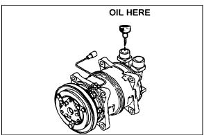
FIGURE 41: ADDING OIL AFTER REPLACING A COMPONENT
