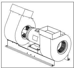
FIGURE 17: EVAPORATOR MOTOR ASSEMBLY
