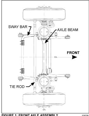
FIGURE 1: FRONT AXLE ASSEMBLY
