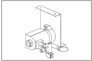
FIGURE 30: AIR HORN VALVE
