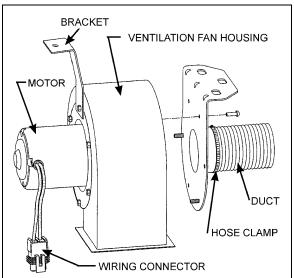
FIGURE 25: VENTILATION FAN INSTALLATION
