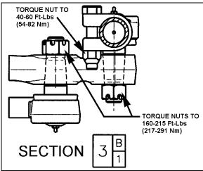
FIGURE 4: CLAMP POSITIONING
