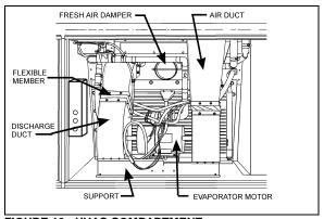
FIGURE 16: HVAC COMPARTMENT
