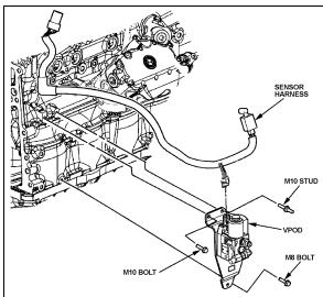
FIGURE 5: VPOD INSTALLATION
