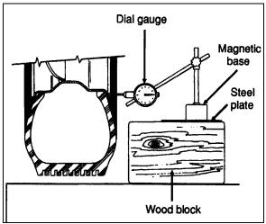
FIGURE 3: DIAL GAUGE INSTALLATION
