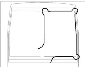
FIGURE 11: WINDSHIELD INSTALLATION USING ROPE
