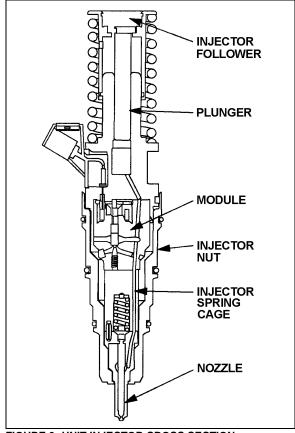
FIGURE 3: UNIT INJECTOR CROSS SECTION
