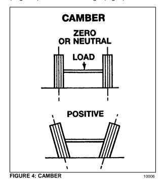
The camber angle is not adjustable. Camber variations may be caused by wear at the wheel bearings, steering knuckle pins or by a bent knuckle or sagging axle center. Steering effort is affected by improper camber, and uneven tire wear will result. Excessive positive camber causes an irregular wear of tire at the outer shoulder and excessive negative camber causes wear at the inner shoulder.
