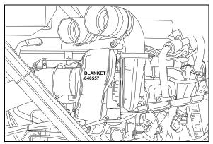
FIGURE 5: TURBO BLANKET INSTALLATION
