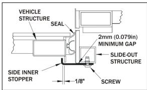
FIGURE 3: SIDE INNER STOPPER ADJUSTMENT
