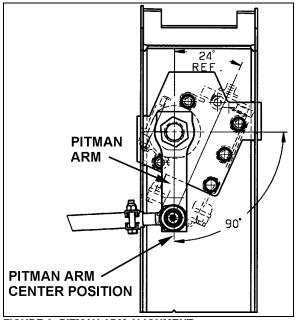
FIGURE 6: PITMAN ARM ALIGNMENT
