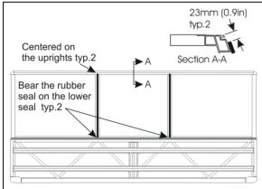
FIGURE 51: FACE FIXED WINDOWS - RUBBER SEAL INSTALLATION
