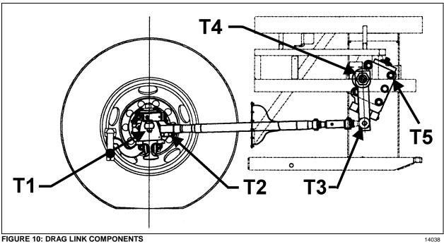
FIGURE 10: DRAG LINK COMPONENTS
