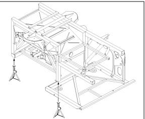
FIGURE 53: FRONT SUBFRAME JACKING POINTS 18592
