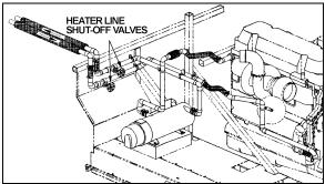
FIGURE 7: COACHES SHUT-OFF VALVES (TYP.) 0114
