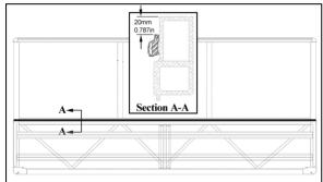
FIGURE 50 : FACE FIXED WINDOWS - RUBBER SEAL INSTALLATION
