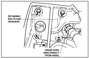
FIGURE 38: ALTERNATOR RETAINING BOLTS AND WASHERS 06350
