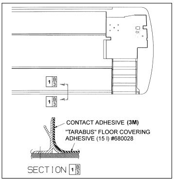
FIGURE 35: TARABUS FLOOR COVERING ADHESIVE APPLICATION
