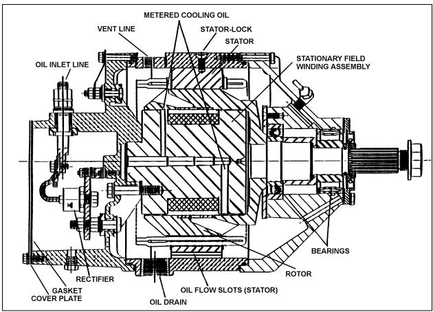
FIGURE 30: 50DN DELCO ALTERNATOR SECTIONAL VIEW
