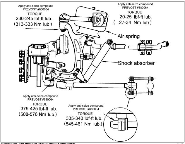
FIGURE 23: AIR SPRING AND SHOCK ABSORBER
