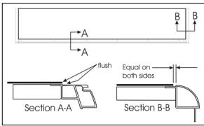
FIGURE 48: TOP PANEL INSTALLATION
