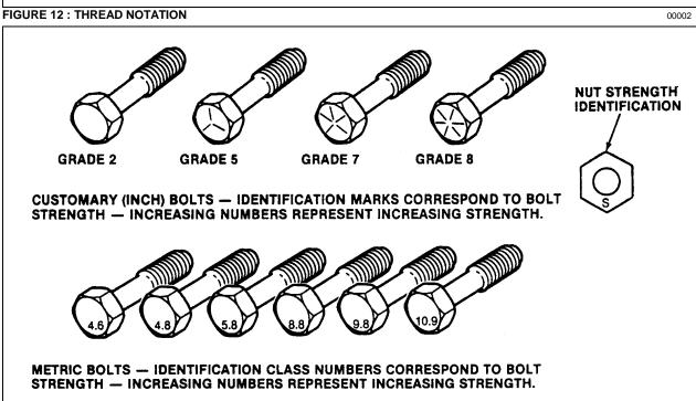
FIGURE 13: BOLT STRENGTH MARKINGS
