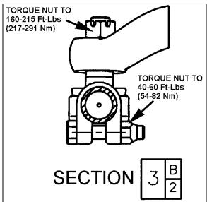
FIGURE 5: CLAMP POSITIONING
