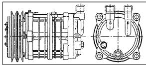
FIGURE 34: SELTEC TM-16HD COMPRESSOR
