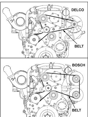
FIGURE 39: ALTERNATOR DRIVE BELT
