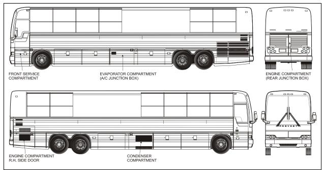
FIGURE 14: ELECTRICAL COMPARTMENTS (XL2-45 BUS SHELLS)
