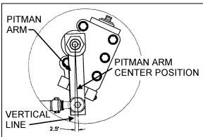
FIGURE 5: PITMAN ARM ADJUSTMENT
