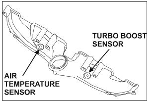
FIGURE 7: TURBO BOOST PRESSURE SENSOR
