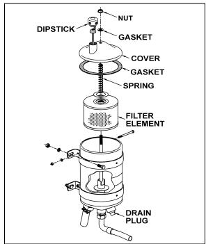
FIGURE 8: POWER STEERING FLUID RESERVOIR 14018A
