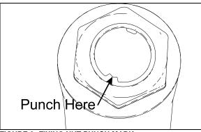
FIGURE 9: FIXING NUT PUNCH MARK
