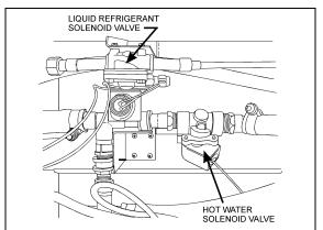
FIGURE 29: DRIVER'S EVAPORATOR LIQUID SOLENOID VALVE
