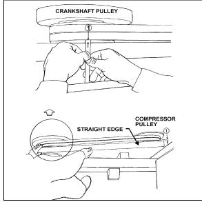
FIGURE 26: COMPRESSOR ALIGNMENT
