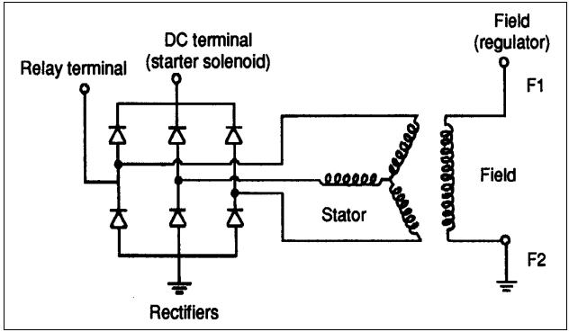
FIGURE 31: ALTERNATOR WIRING DIAGRAM (DELCO)
