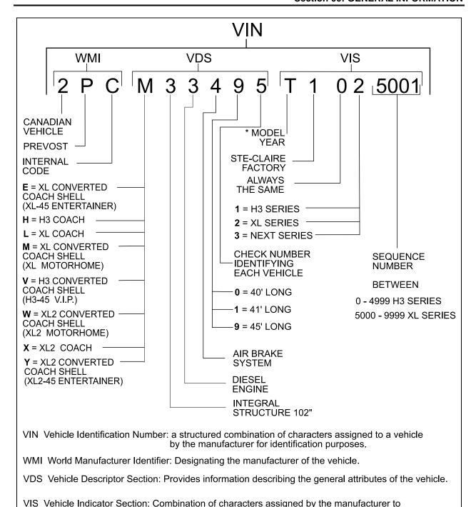
FIGURE 11: VEHICLE IDENTIFICATION NUMBER
