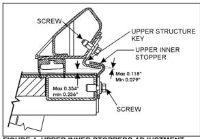
FIGURE 4: UPPER INNER STOPPERS ADJUSTMENT
