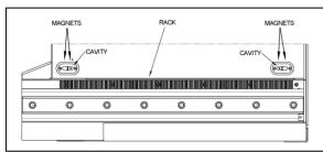
FIGURE 39: MAGNETS ON SLIDE-OUT UNDERBODY
