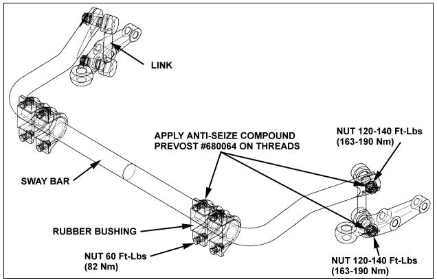
FIGURE 25: SWAY BAR (FRONT SUSPENSION)
