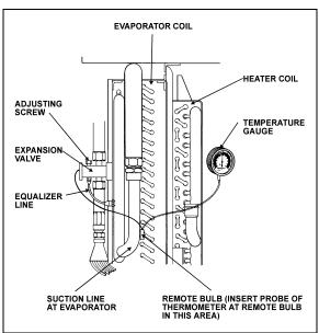
FIGURE 32: SUPERHEAT ADJUSTMENT INSTALLATION22046
