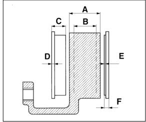
FIGURE 32: ROTOR AND PAD WEAR LIMITS
