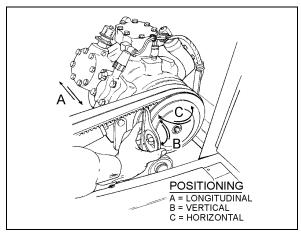
FIGURE 25: COMPRESSOR ALIGNMENT
