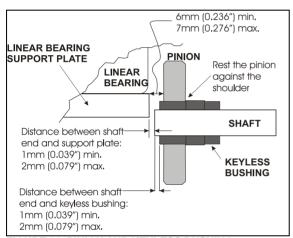
FIGURE 11: PINION AND KEYLESS BUSHING POSITIONING
