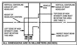
FIGURE 61: AIM INSPECTION LIMITS FOR LOWER-BEAM HEADLIGHTS 06506
