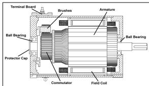
FIGURE 27: CONDENSER FAN MOTOR
