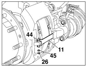
FIGURE 24: CLEARANCE INSPECTION
