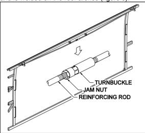
FIGURE 9 : FRONT SLIDE-OUT ROOF REINFORCING
