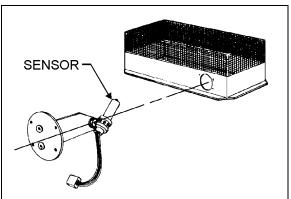
FIGURE 6: THERMISTOR SENSOR
