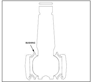
FIGURE 16: LOWER A-ARM CENTRAL BALL JOINT 16113
