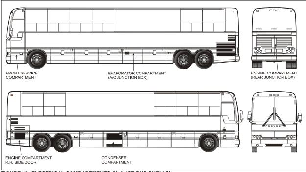
FIGURE 13: ELECTRICAL COMPARTMENTS (XL2-45E BUS SHELLS)
