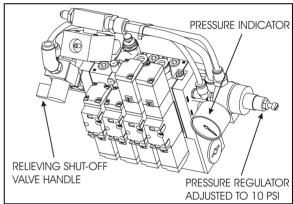
FIGURE 91: INFLATABLE SEAL RELIEVING SHUT-OFF VALVE
