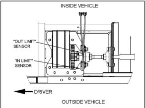
FIGURE 38: REAR SLIDE-OUT SENSORS
