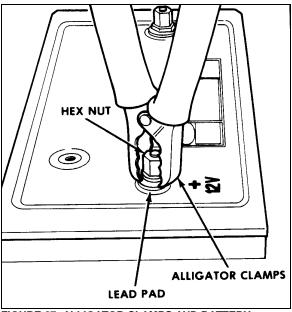
FIGURE 27: ALLIGATOR CLAMPS AND BATTERY 06065
