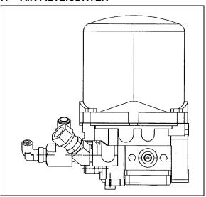
FIGURE 5: HALDEX AIR FILTER DRYER
