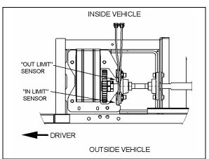
FIGURE 38: REAR SLIDE-OUT SENSORS
