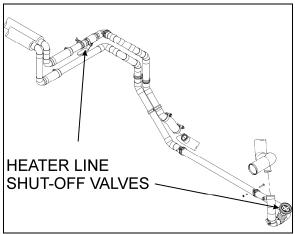
FIGURE 39: HEATER LINE SHUT-OFF VALVES
