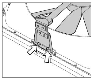
FIGURE 19: REMOVING UPPER FAN DRIVE SUPPORT BRACKET
