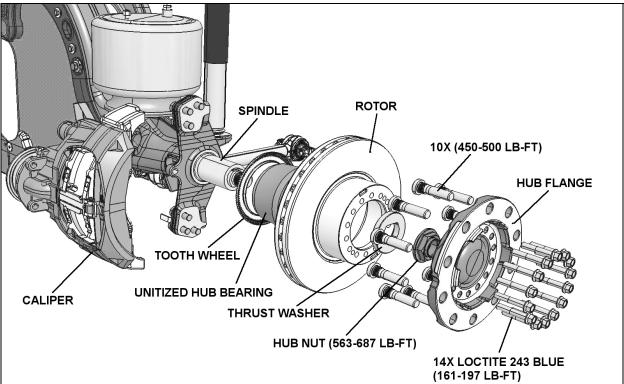
FIGURE 7: FRONT & TAG AXLE HUB AND ROTOR ASSEMBLY
