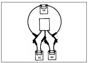
FIGURE 46: CHECKING TRANSISTOR TR2
