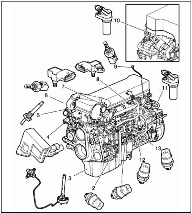
FIGURE 1: ENGINE SENSORS LOCATION
