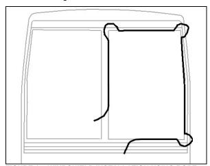
FIGURE 15: WINDSHIELD INSTALLATION USING ROPE
