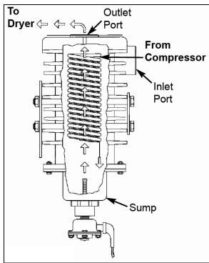
FIGURE 6: HALDEX CONSEP CONDENSER/SEPARATOR
