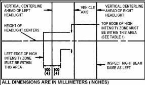
FIGURE 61: A IM INSPECTION LIMITS FOR LOWER-BEAM HEADLIGHTS 06506
