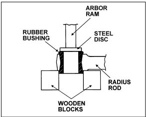
FIGURE 7: RADIUS ROD BUSHING REMOVAL
