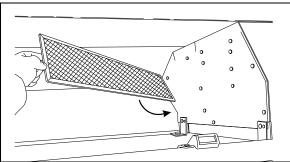
FIGURE 17: OVERHEAD COMPARTMENT FAN AIR **FILTER**
