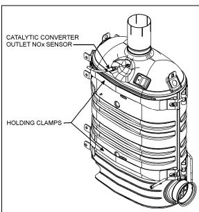
FIGURE 5: CATALYTIC CONVERTER
