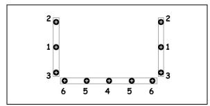
FIGURE 67: CORRECT TIGHTENING SEQUENCE
