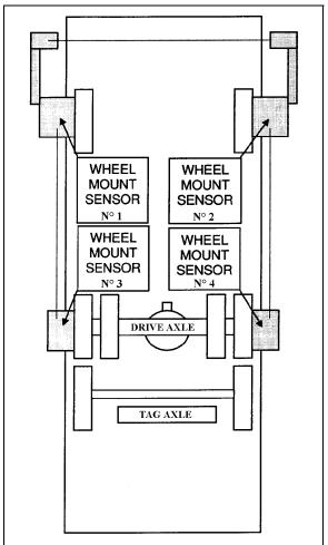
FIGURE 6: FRONT & DRIVE AXLE ALIGNMENT 11025
