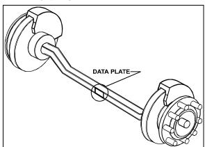
FIGURE 5: TYPICAL SERIAL & MODEL NUMBERS 10024
