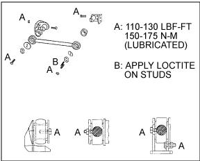
FIGURE 47: RADIUS ROD INSTALLATION
