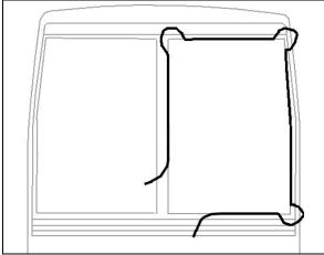
FIGURE 74: WINDSHIELD INSTALLATION USING ROPE
