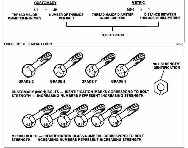
FIGURE 13: BOLT STRENGTH MARKINGS
