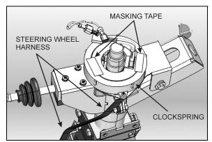
FIGURE 11: LOCKING THE CLOCKSPRING IN PLACE
