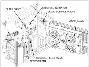
FIGURE 30: A/C CONDENSER COMPARTMENT
