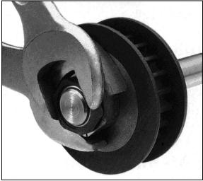
FIGURE 14: KEYLESS BUSHING TIGHTENING
