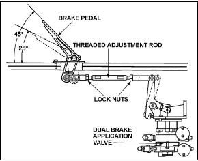
FIGURE 13: BRAKE PEDAL ADJUSTMENT
