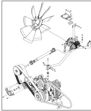
FIGURE 21: COOLING FAN DRIVE MECHANISM
