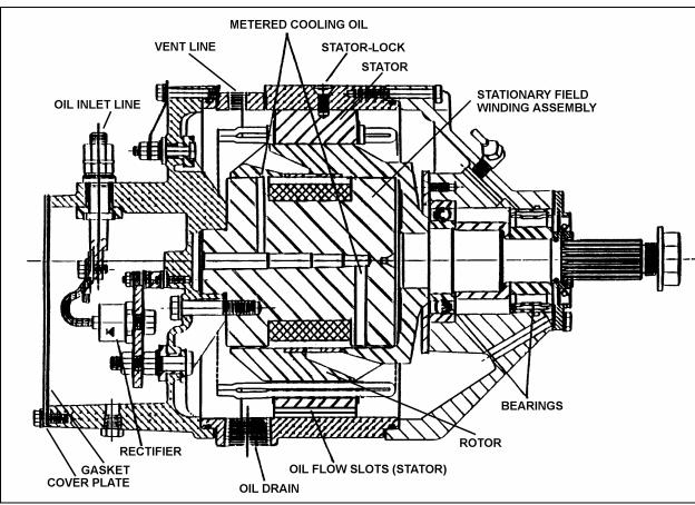
FIGURE 30: 50DN DELCO ALTERNATOR SECTIONAL VIEW
