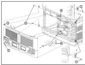
FIGURE 57: ENGINE COMPARTMENT DOORS
