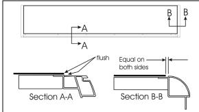
FIGURE 48: TOP PANEL INSTALLATION
