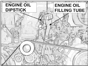
FIGURE 7: ENGINE OIL FILLING TUBE
