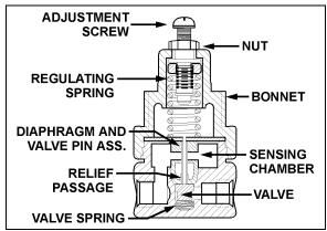
FIGURE 7: AIR PRESSURE REGULATING VALVE 12141A
