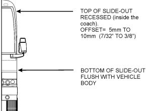
FIGURE 23: TILT ADJUSTMENT
