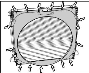
FIGURE 20: REMOVING FAN SHROUD FROM RADIATOR
