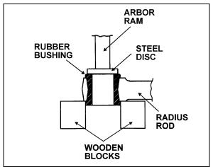
FIGURE 45: RADIUS ROD BUSHING REMOVAL
