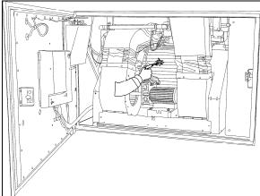
FIGURE 12: EVAPORATOR COIL CLEANING
