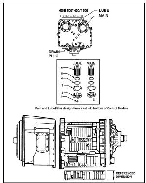
FIGURE 6: DRAIN PLUG AND FILTERS
