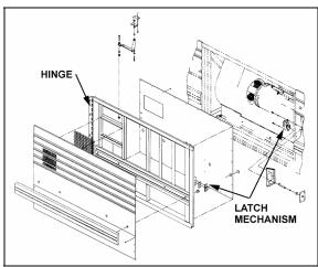
FIGURE 65: EVAPORATOR DOOR
