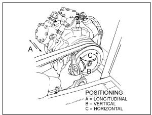
FIGURE 24: COMPRESSOR ALIGNMENT
