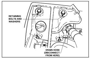
FIGURE 38: A LTERNATOR RETAINING BOLTS AND WASHERS 06350
