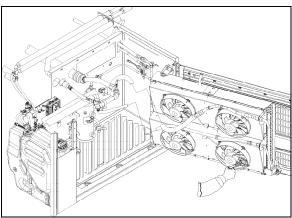
FIGURE 13: CONDENSER COMPARTMENT
