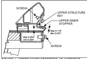
FIGURE 4: UPPER INNER STOPPERS ADJUSTMENT
