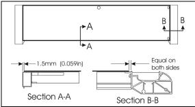
FIGURE 49: BOTTOM PANEL INSTALLATION
