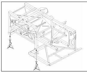
FIGURE 95: FRONT SUBFRAME JACKING POINTS 18592
