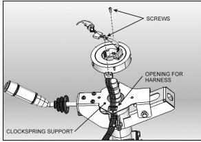
FIGURE 12: CLOCKSPRING INSTALLATION
