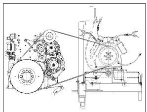
FIGURE 23: A/C COMPRESSOR BELT ADJUSTMENT22288
