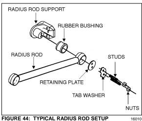
FIGURE 44: TYPICAL RADIUS ROD SETUP
