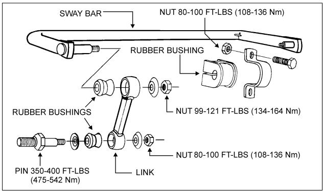
FIGURE 37: SWAY BAR (REAR SUSPENSION)
