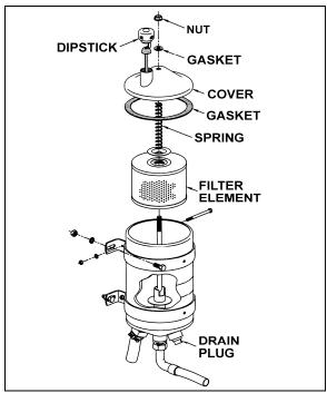
FIGURE 18: POWER STEERING FLUID RESERVOIR 14018
