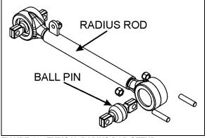
FIGURE 48: TYPICAL RADIUS ROD SETUP
