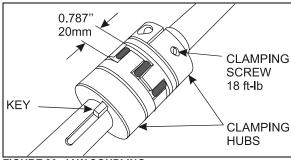
FIGURE 20: JAW COUPLING
