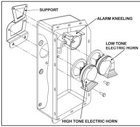
FIGURE 2: ELECTRIC HORN INSTALLATION
