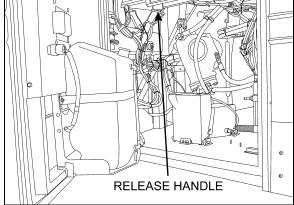
FIGURE 50: FRONT BUMPER RELEASE HANDLE 18613
