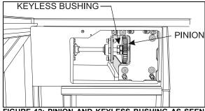
FIGURE 12: PINION AND KEYLESS BUSHING AS SEEN FROM EVAPORATOR COMPARTMENT
