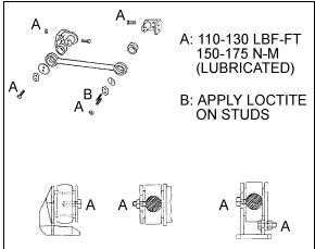
FIGURE 9: RADIUS ROD INSTALLATION
