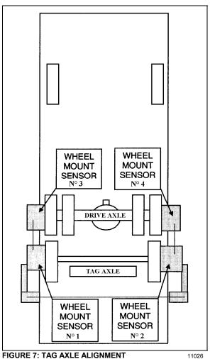
FIGURE 7: TAG AXLE ALIGNMENT
