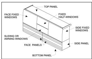
FIGURE 40 : SLIDE-OUT PANELS AND WINDOWS
