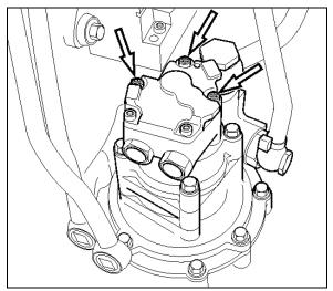
FIGURE 6: FUEL PUMP REMOVAL
