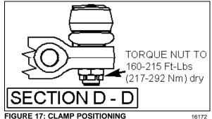
FIGURE 17: CLAMP POSITIONING
