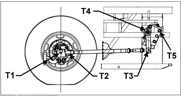
FIGURE 20: DRAG LINK COMPONENTS
