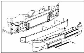
FIGURE 12: FRONT BUMPER REMOVAL
