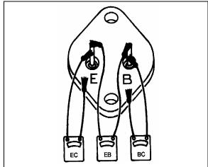
FIGURE 45: CHECKING TRANSISTOR TR1
