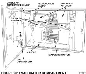
FIGURE 26: EVAPORATOR COMPARTMENT
