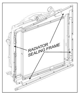
FIGURE 11: RADIATOR SEALING FRAME
