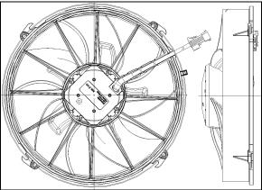
FIGURE 29: CONDENSER FAN MOTOR
