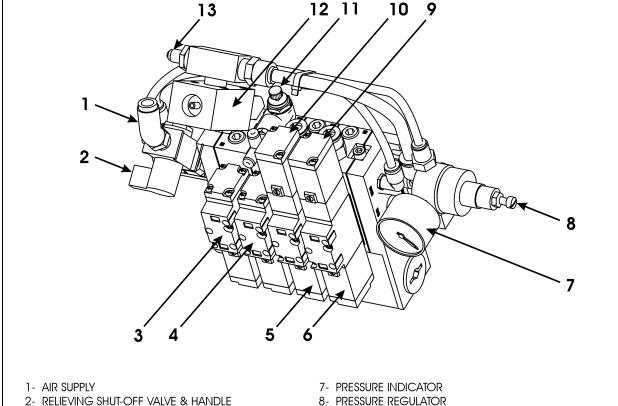
FIGURE 29: PNEUMATIC COMPONENT PANEL
