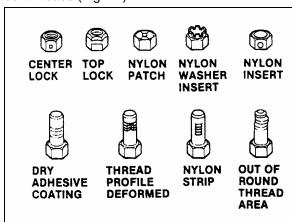
FIGURE 14: SELF-LOCKING FASTENERS
