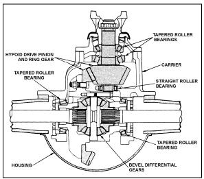
FIGURE 2: DIFFERENTIAL ASSEMBLY
