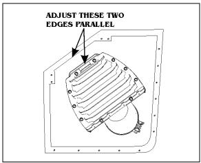
FIGURE 7: DIFFUSER POSITION ADJUSTMENT 04015 1
