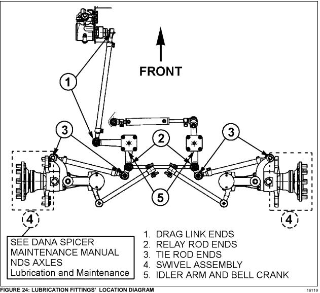
FIGURE 24: LUBRICATION FITTINGS' LOCATION DIAGRAM
