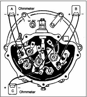
FIGURE 36: STATOR WINDING TEST
