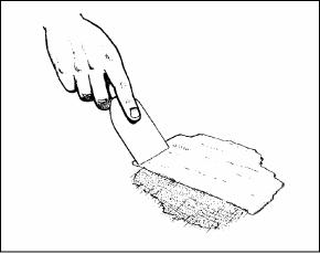
FIGURE 8: FIBERGLASS REPAIR
