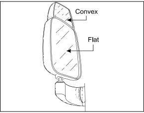
FIGURE 14: REAR VIEW MIRROR (RAMCO)
