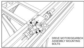
FIGURE 18: DRIVE MOTOR/GEARBOX ASSEMBLY MOUNTING BOLTS
