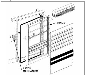
FIGURE 34: R.H. SIDE REAR SERVICE COMPARTMENT DOOR
