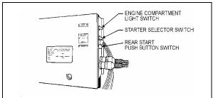
FIGURE 10: REAR JUNCTION BOX SWITCHES 01017
