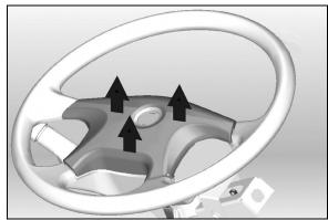
FIGURE 9: REMOVING THE HORN PAD
