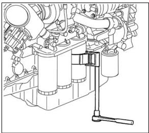
FIGURE 5: OIL FILTER WRENCH
