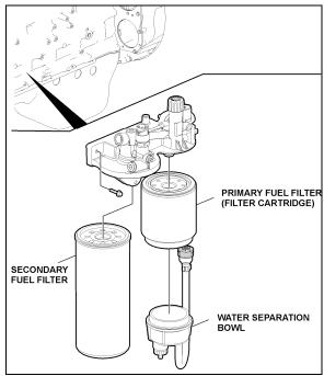
FIGURE 4: FUEL FILTERS WITH VOLVO D13 ENGINE
