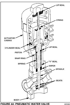
FIGURE 44: PNEUMATIC WATER VALVE
