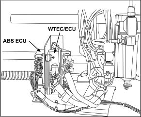
FIGURE 8: BOTTOM SECTION OF FRONT SERVICE COMPARTMENT 06394
