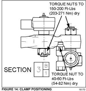
FIGURE 14: CLAMP POSITIONING
