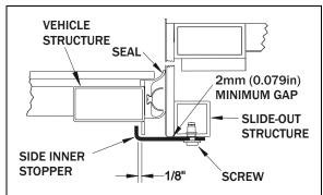
FIGURE 3: SIDE INNER STOPPER ADJUSTMENT
