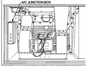
FIGURE 17: LOCATION OF A /C JUNCTION BOX IN EVAPORATOR COMPARTMENT 22178
