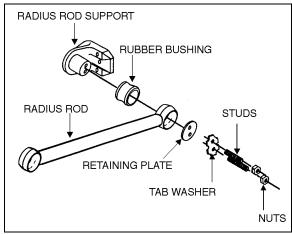
FIGURE 6: TYPICAL RADIUS ROD SETUP
