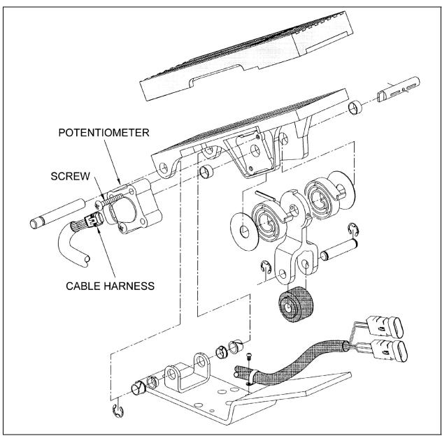
FIGURE 14: ELECTRONIC FOOT PEDAL ASSEMBLY
