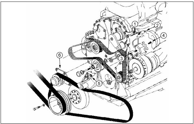
FIGURE 28: TWIN BOSCH ALTERNATORS INSTALLATION
