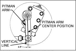
FIGURE 14: PITMAN ARM ADJUSTMENT
