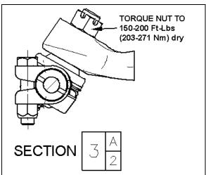
**FIGURE 16: CLAMP POSITIONING**
