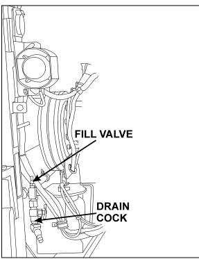
FIGURE 55: REAR VALVE LOCATION
