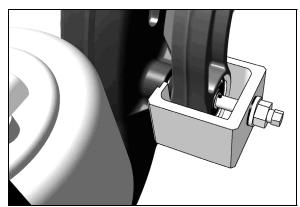
FIGURE 11: INSTALLING EXTRACTOR TOOL
