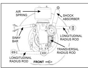
FIGURE 1: FRONT SUSPENSION COMPONENTS
