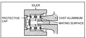
FIGURE 24: IDLER MOUNTED ON THE CAST ALUMINUM SUPPORT
