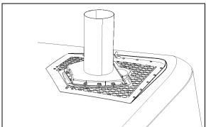
FIGURE 10: EXHAUST GAS COLLECTION ADAPTER04020
