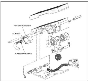
FIGURE 11: ELECTRONIC FOOT PEDAL ASSEMBLY 03035
