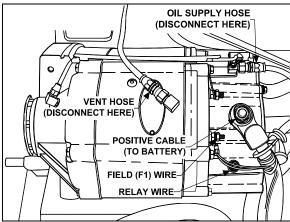
FIGURE 37: ALTERNATOR (HOSES AND WIRES) 06
