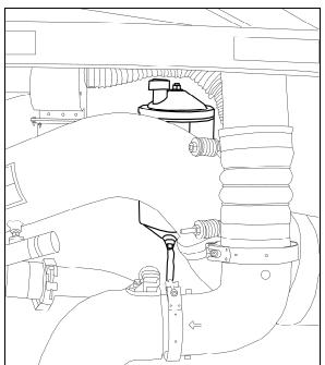
FIGURE 17: HYDRAULIC FLUID RESERVOIR LOCATION
