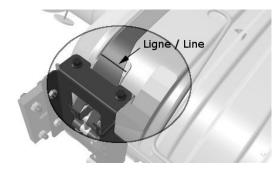
Mark, with a vertical line the central position of the lower and upper clamps with regard to the emboss located at the bottom and at the top of the catalytic converter.
