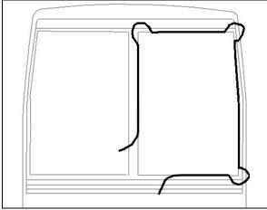
FIGURE 52: WINDSHIELD INSTALLATION USING ROPE
