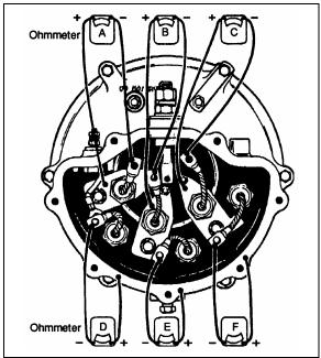
FIGURE 35: DIODE TESTING
