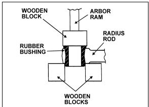
FIGURE 46: RADIUS ROD BUSHING INSTALLATION 16012
