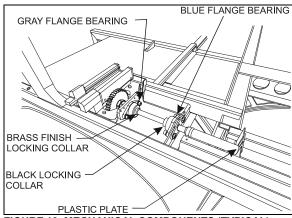
FIGURE 13: MECHANICAL COMPONENTS (TYPICAL)
