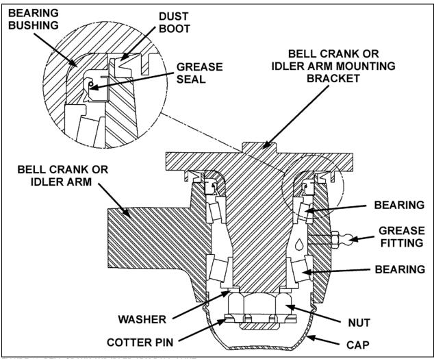
FIGURE 23: BELL CRANK AND IDLER ARM BALL JOINT
