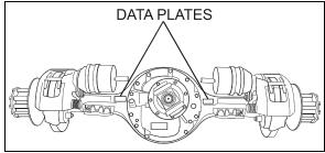
FIGURE 4: TYPICAL SERIAL & MODEL NUMBERS 1101
