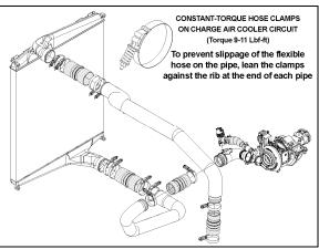
FIGURE 4: CHARGE AIR COOLER HOSE CLAMPS
