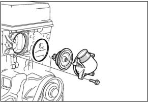
FIGURE 5: VOLVO D13 THERMOSTAT HOUSING
