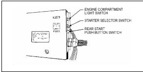
FIGURE 22: REAR JUNCTION BOX SWITCHES 0
