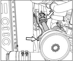
FIGURE 16: DISCONNECTING FAN DRIVE SHAFT
