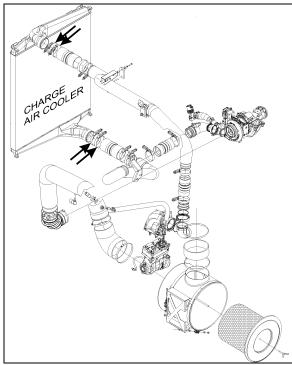
FIGURE 13: CHARGE AIR COOLER HOSE CLAMPS
