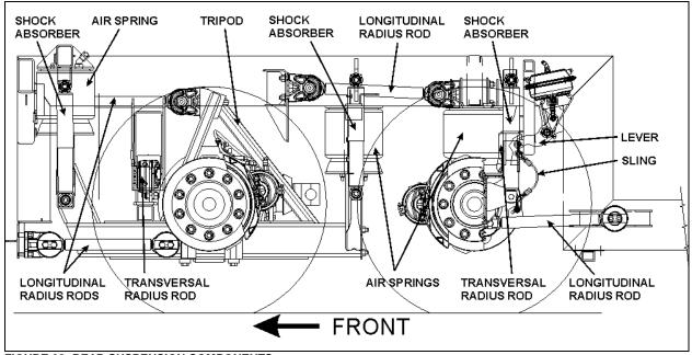
FIGURE 38: REAR SUSPENSION COMPONENTS
