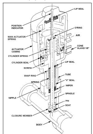
FIGURE 42: PNEUMATIC WATER VALVE
