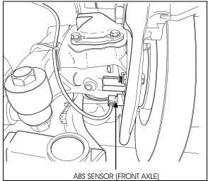
FIGURE 33: ABS SENSOR LOCATION
