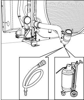
FIGURE 7: EXTRACTING COOLANT
