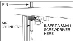
FIGURE 8: SECURITY PIN AIR CYLINDER REMOVAL
