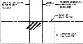
FIGURE 59: HIGH-INTENSITY ZONE (SHADED AREA) OF A PROPERLY AIMED LOWER BEAM ON THE AIMING SCREEN 7.6 M (25FT) IN FRONT OF VEHICLE 06504
