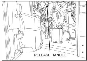
FIGURE 13: FRONT BUMPER RELEASE HANDLE
