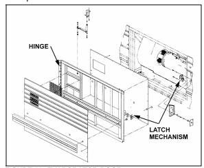
FIGURE 88: EVAPORATOR DOOR
