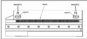
FIGURE 39: MAGNETS ON SLIDE-OUT UNDERBODY
