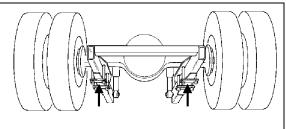
FIGURE 98: JACKING POINTS ON DRIVE AXLE OEH3B762
