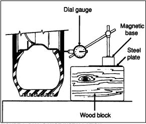
FIGURE 3: DIAL GAUGE INSTALLATION
