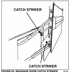
If the lower part of the baggage door does not close evenly with the side of the vehicle, adjust the lock plates by loosening their retaining bolts and positioning the locking plates correctly (Fig. 63).
