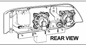
FIGURE 50: HEADLIGHT ASSEMBLY REAR VIEW 06548
