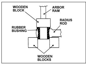
FIGURE 8: RADIUS ROD BUSHING INSTALLATION 16012
