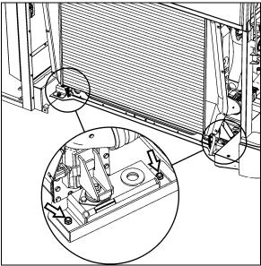
FIGURE 15: RADIATOR ASSEMBLY LOWER MOUNTING FASTENERS
