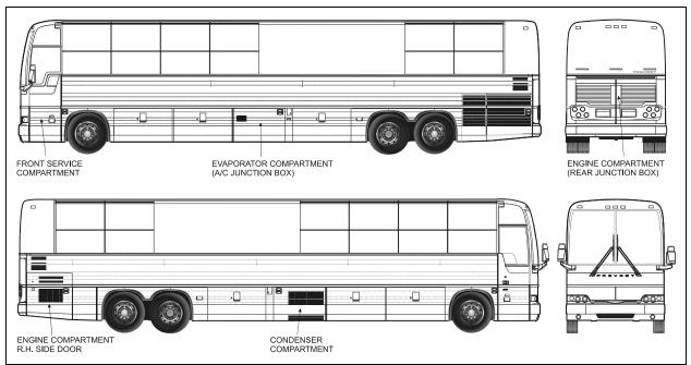
FIGURE 14: ELECTRICAL COMPARTMENTS (XL2-45 BUS SHELLS)
