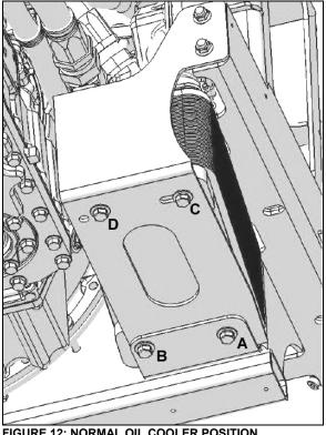
FIGURE 12: NORMAL OIL COOLER POSITION
