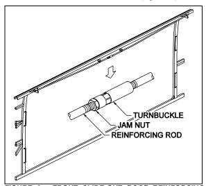
FIGURE 9 : FRONT SLIDE-OUT ROOF REINFORCING ROD
