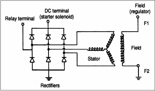
FIGURE 31: ALTERNATOR WIRING DIAGRAM (DELCO)
