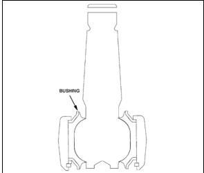
FIGURE 29: LOWER A-ARM CENTRAL BALL JOINT 16113
