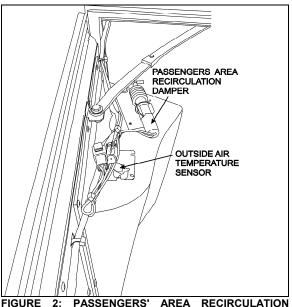
FIGURE 2: PASSENGERS' AREA RECIRCULATION DAMPER 22302
