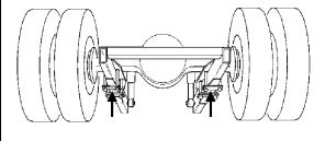
FIGURE 5: JACKING POINTS ON DRIVE AXLE
