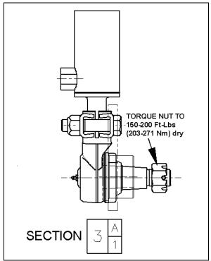
FIGURE 15: CLAMP POSITIONING
