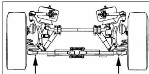
FIGURE 97: JACKING POINTS ON IND. SUSPENSION 16095
