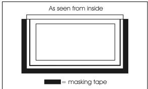
FIGURE 63: MASKING TAPE APPLICATION
