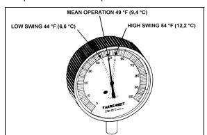
FIGURE 35: HIGH & LOW SWING TEMPERATURE AT REMOTE BULB 22047
