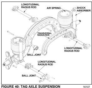
**FIGURE 40: TAG AXLE SUSPENSION**
