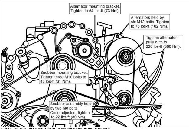
FIGURE 29: ALTERNATORS AND ACCESSORIES MOUNTING TORQUES
