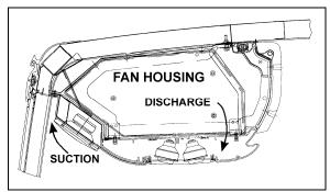
FIGURE 4: PASSENGERS OVERHEAD COMPARTMENT VENTILATION SYSTEM 22211
