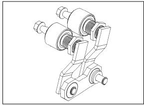
FIGURE 9: DRIVING MECHANISM (DRIVER SIDE) 23284
