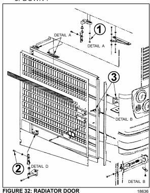
Adjust the door position depending on the gap needed between exterior finishing panels.
