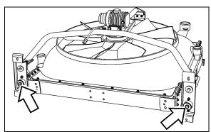
FIGURE 18: REMOVING FASTENERS
