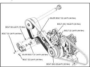
FIGURE 23: TIGHTENING SPECIFICATION (VOLVO D13 ENGINE)
