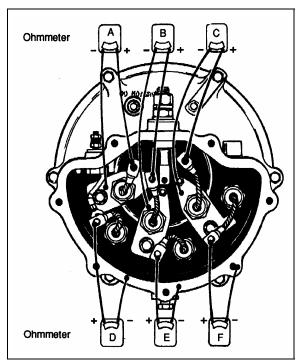
FIGURE 34: DIODE TESTING
