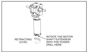
FIGURE 92: SLIDE-OUT MOTOR ROTATION
