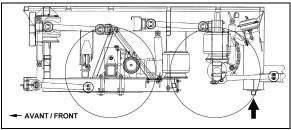
FIGURE 96: REAR SUBFRAME JACKING POINTS
