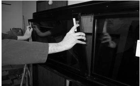
FIGURE 22: REMOVING THE SASH
