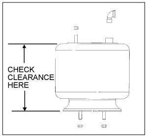
FIGURE 50: TYPICAL AIR SPRING CLEARANCE 160
