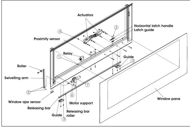
FIGURE 20: ELECTRIC AWNING WINDOW EXPLODED VIEW (SASH)
