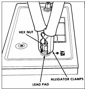
FIGURE 27: ALLIGATOR CLAMPS AND BATTERY 06065
