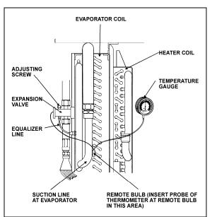
FIGURE 34: SUPERHEAT ADJUSTMENT INSTALLATION22046
