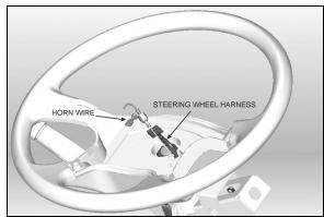
FIGURE 10: STEERING HARNESS & HORN WIRE
