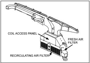
FIGURE 15: DRIVER'S SECTION AIR FILTERS
