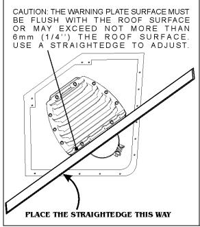
FIGURE 8: DIFFUSER POSITION ADJUSTMENT 04015\_2
