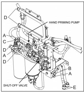
FIGURE 2: MANUAL SHUT-OFF VALVE (VOLVO D13 ENGINE)
