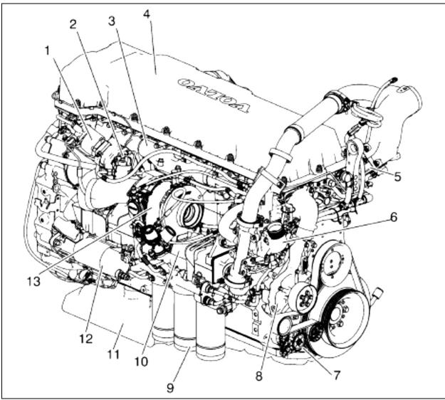
FIGURE 2: D13F ENGINE, TURBO SIDE (TYPICAL)
