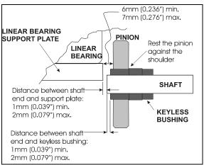
FIGURE 11: PINION AND KEYLESS BUSHING POSITIONING
