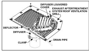
FIGURE 6: DIFFUSER ASSEMBLY
