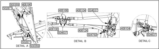
FIGURE 13: NOZZLE BRACKETS IDENTIFICATION AND INSTALLATION
