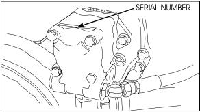
FIGURE 7: POWER STEERING PUMP NAMEPLATE 00035
