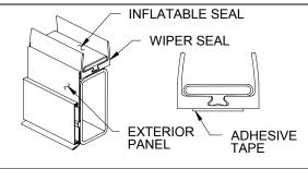
FIGURE 30 : SEAL ASSEMBLY
