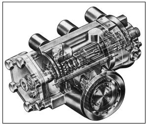
FIGURE 2: POWER STEERING GEAR
