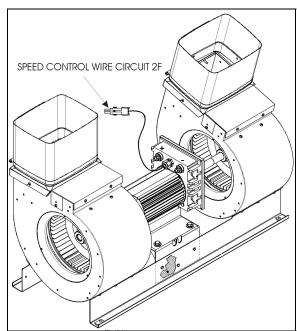
FIGURE 28: EVAPORATOR MOTOR ASSEMBLY
