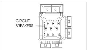
FIGURE 36: VEC CIRCUIT BREAKERS & FUSES
