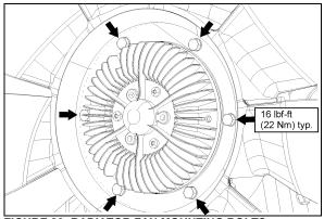
FIGURE 26: RADIATOR FAN MOUNTING BOLTS
