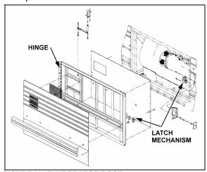
FIGURE 39: EVAPORATOR DOOR
