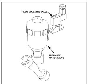
FIGURE 41: DRIVER'S HOT WATER PNEUMATIC VALVE ASSEMBLY
