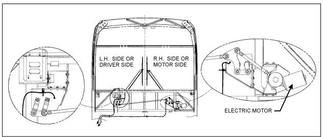
FIGURE 6: WINDSHIELD WIPER INSTALLATION
