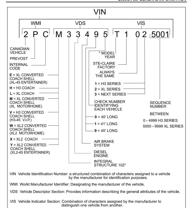
FIGURE 11: VEHICLE IDENTIFICATION NUMBER
