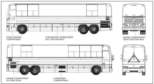
FIGURE 12: ELECTRICAL COMPARTMENTS (XL2-40 BUS SHELLS)
