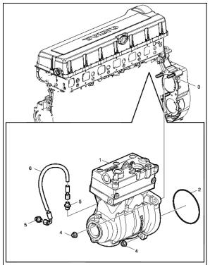
FIGURE 9: AIR COMPRESSOR LOCATION
