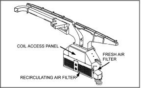
FIGURE 10: DRIVER'S HVAC UNIT COIL ACCESS PANEL
