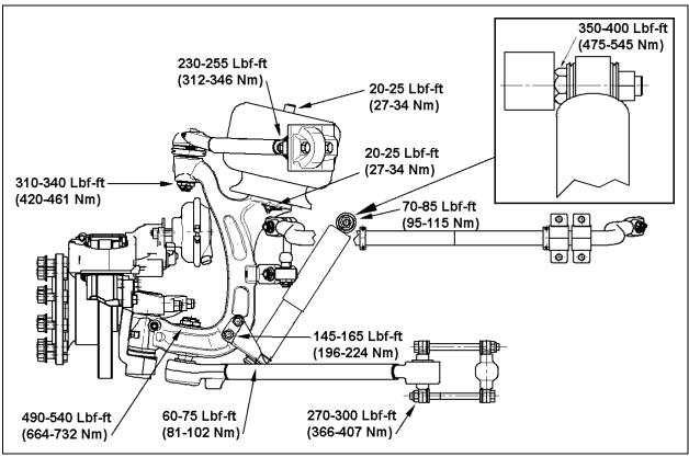
FIGURE 34: AIR SPRING AND SHOCK ABSORBER
