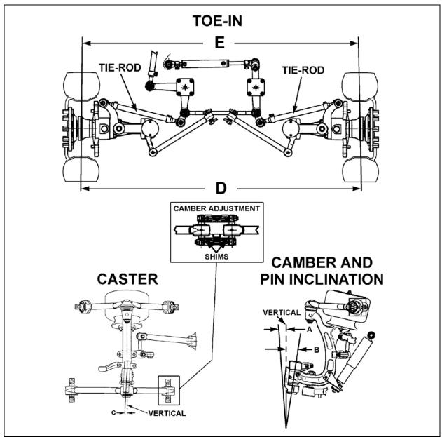
FIGURE 32: FRONT END ALIGNMENT DIAGRAM
