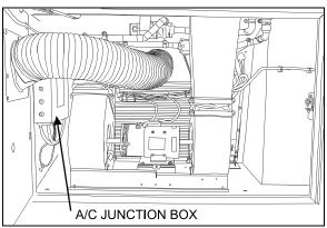
FIGURE 5: LOCA TION OF A /C JUNCTION BOX IN EVAPORATOR COMPARTMENT 22244B
