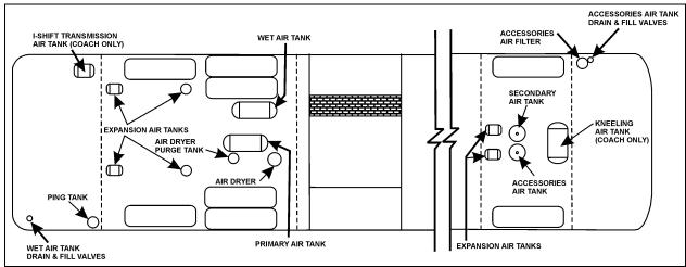
FIGURE 53: IFS AIR TANKS LOCATION
