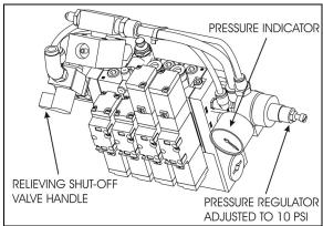
FIGURE 91: INFLATABLE SEAL RELIEVING SHUT-OFF VALVE
