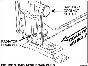
FIGURE 9: RADIATOR DRAIN PLUG
