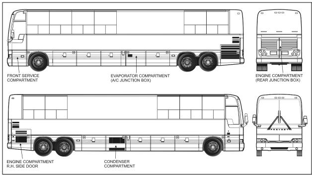
FIGURE 13: ELECTRICAL COMPARTMENTS (XL2-45E BUS SHELLS)
