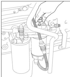
FIGURE 5: HAND PRIMING PUMP
