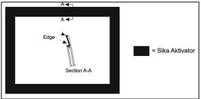
FIGURE 54 : FACE FIXED WINDOW AND HALF-WINDOW – SIKA AKTIVATOR
