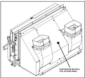
FIGURE 11: EVAPORATOR COIL ACCESS PANEL (TYPICAL) 22309
