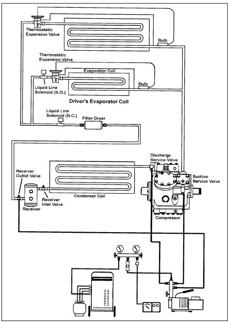
FIGURE 19: DOUBLE-SWEEP EVACUATION SET-UP
