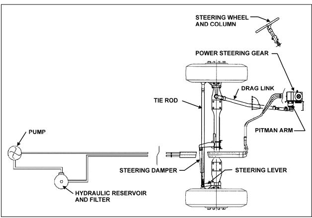
FIGURE 1: I-BEAM AXLE STEERING SYSTEM SETUP
