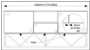
FIGURE 59: FACE FIXED WINDOW INSTALLATION
