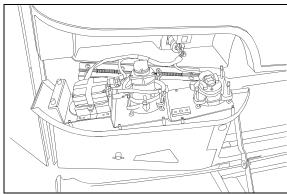
FIGURE 49: OPENING HEADLIGHT ASSEMBLY
