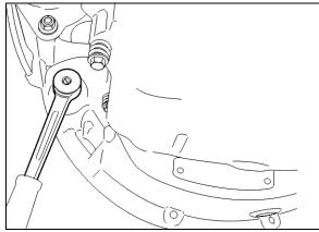
FIGURE 7: VOLVO ENGINE CRANKING POSITION
