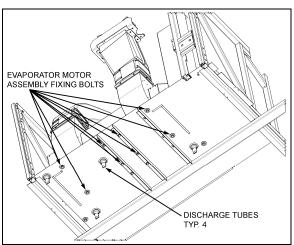
FIGURE 27: EVAPORATOR MOTOR ASSY FIXING BOLTS
