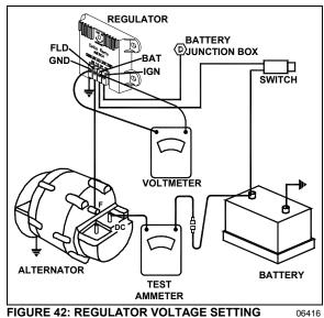
FIGURE 42: REGULATOR VOLTAGE SETTING
