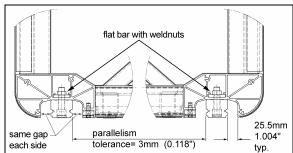
FIGURE 24: RAIL POSITIONING
