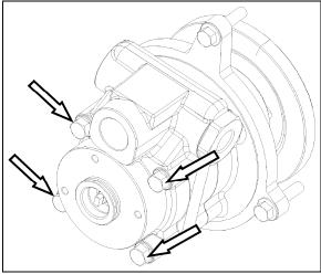
FIGURE 6: POWER STEERING PUMP REMOVAL
