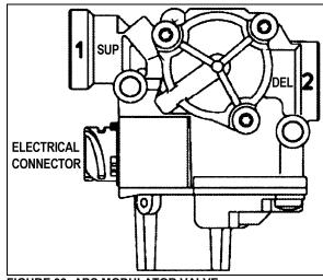
FIGURE 32: ABS MODULATOR VALVE
