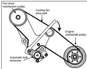
FIGURE 29: DRIVE BELT ROUTING (VOLVO D13 ENGINE)
