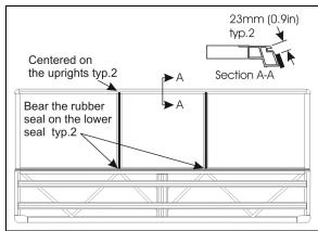
FIGURE 51 : FACE FIXED WINDOWS - RUBBER SEAL INSTALLATION
