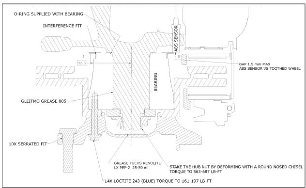
FIGURE 6: FRONT & TAG AXLE WHEEL HUB
