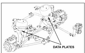
FIGURE 6: ISS TYPICAL SERIAL & MODEL NUMBERS
