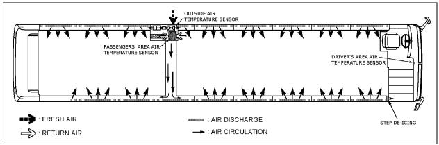
FIGURE 3: CENTRAL HVAC SYSTEM AIR CIRCULATION
