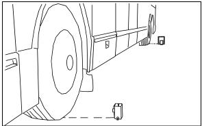
FIGURE 56: INSTALLING CALIBRATION FIXTURES 06497
