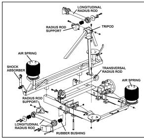
FIGURE 39: REAR UNDERFRAME SUSPENSION
