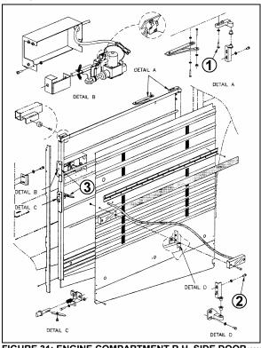
FIGURE 31: ENGINE COMPARTMENT R.H. SIDE DOOR 18635
