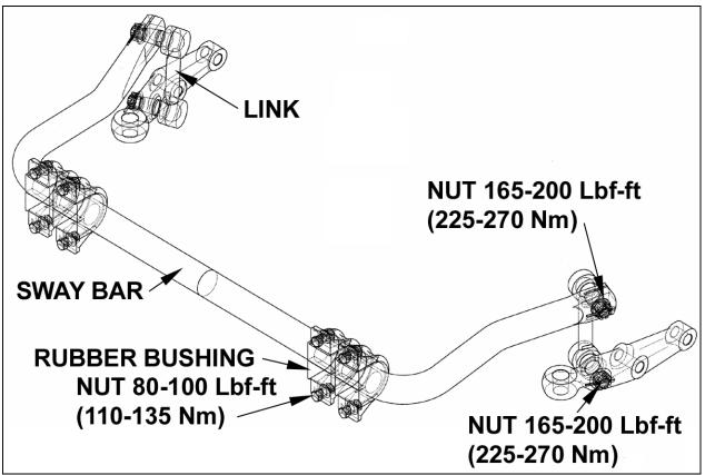
FIGURE 36: SWAY BAR (FRONT SUSPENSION)
