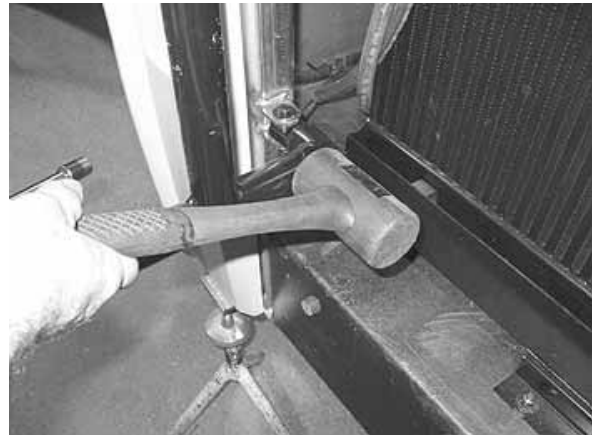
FIGURE 70: PANTOGRAPH ARM ADJUSTMENT
