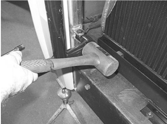
FIGURE 63: PANTOGRAPH ARM ADJUSTMENT
